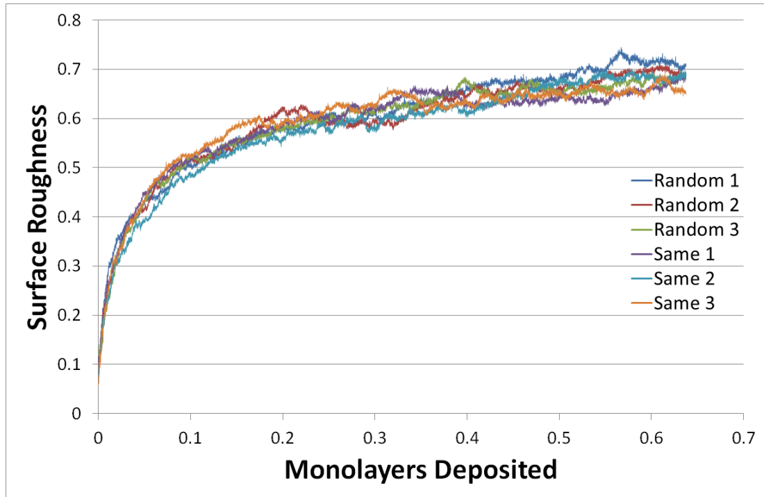
Figure 54: Comparison of surface roughness for simulations of a polar angle of 30^\circ with 3 using random azimuthal angles and 3 using the same azimuthal angle
