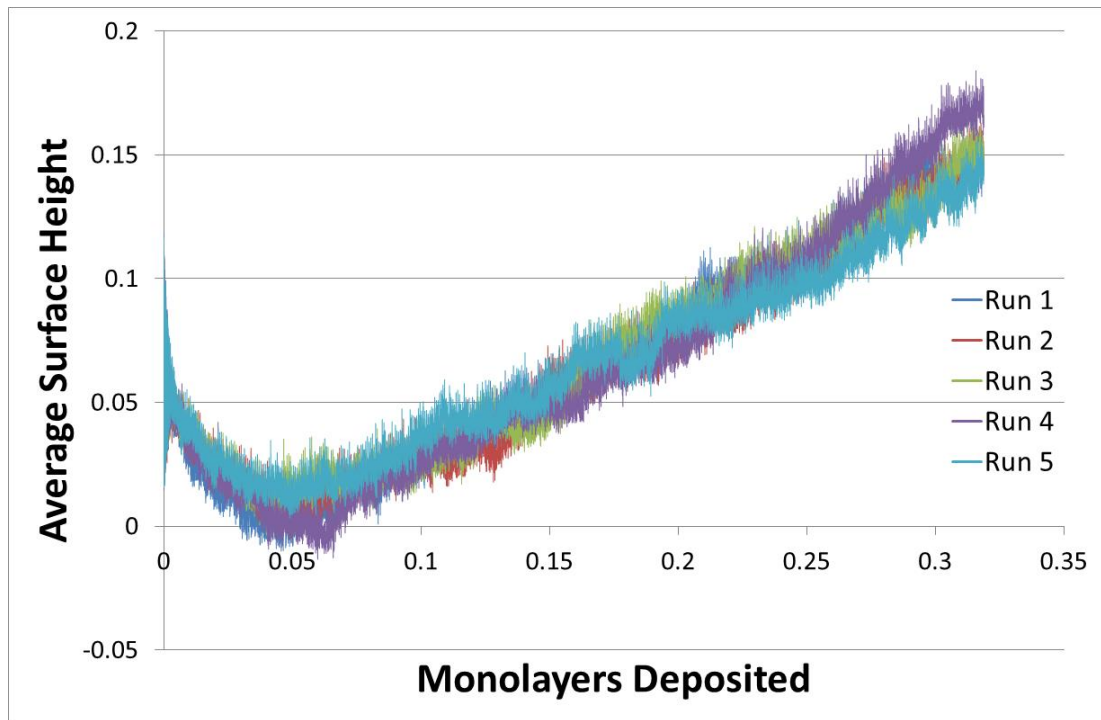
Figure 48: Comparison of average surface height surface roughness for multiple simulations on the 56 by 28 surface using the same input conditions
