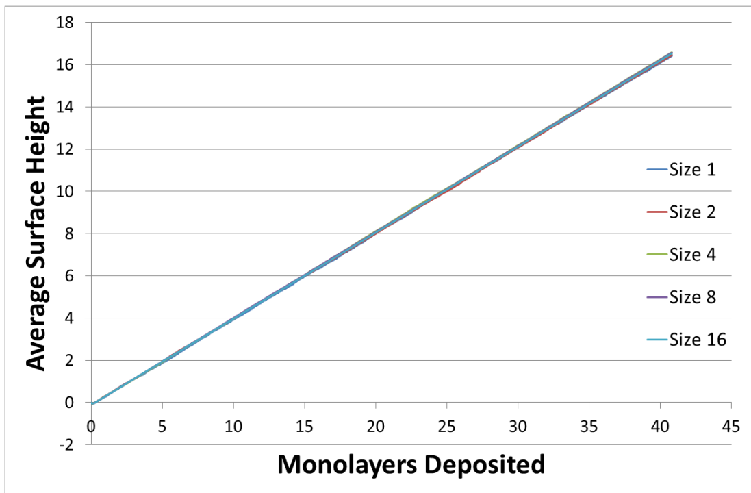
Figure 113: Average surface height during simulations of the deposition of the equivalent of 40 monolayers at various surface sizes
