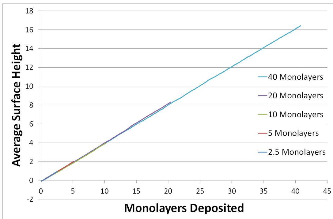
Figure 108: Average surface height of Jv3 simulation after depositing the equivalent of 2.5, 5, 10, 20 and 40 monolayers
