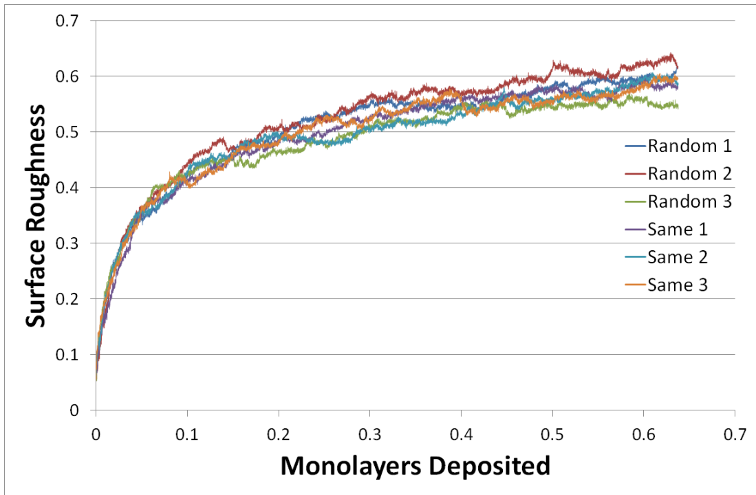
Comparison of surface roughness for simulations of a polar angle of 60° with 3 using random azimuthal angles and 3 using the same azimuthal angle
