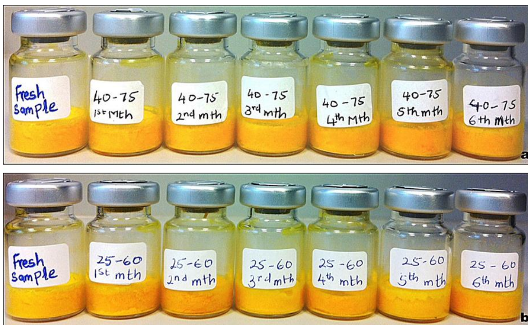
Figure 2.6 Photograph of nCUR subjected to ICH stability test conditions (a) fresh and 1-6 months at room temperature conditions (b) fresh and 1-6 months at refrigerated conditions.
