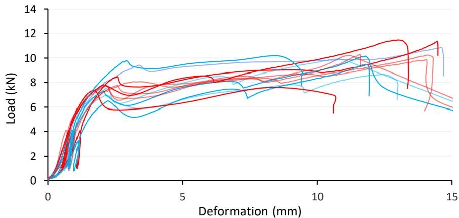
**Figure 7-36: Load deformation curve for 4 plane shear test using 20mm laminations parallel to the grain.**
