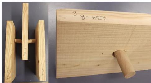
**Figure 7-43: Embedment of laminations and crushing of hardwood dowel.**
