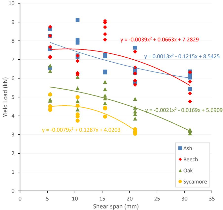
Figure 6-17: Graph illustrating the ultimate bending resistance of a 20.50mm dowel as a function of the shear span.
