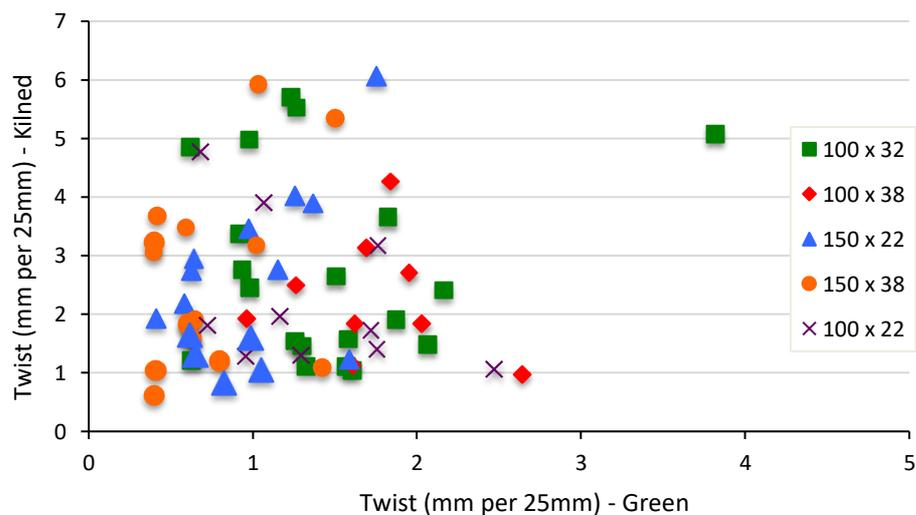
**Figure 6-10: Comparison between twist of Scottish Sitka spruce pre and post kilning.**
