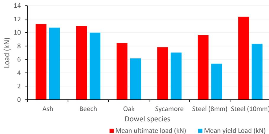
**Figure 7-21: Comparison of the mean yield and ultimate loads of 20.50mm diameter hardwood dowels and 8-10mm mild steel dowels in 30mm diameter larch laminations**
