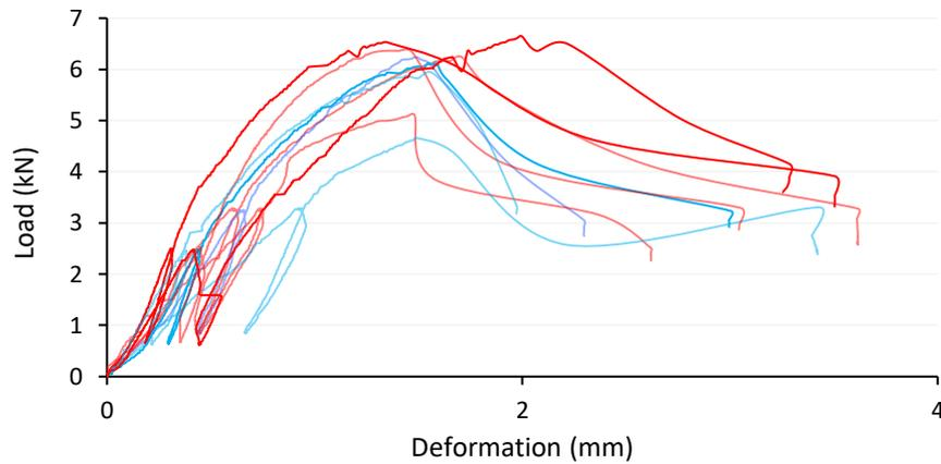
**Figure 7-40: Load deformation curve for 4 plane shear test using 20mm laminations perpendicular to the grain.**
