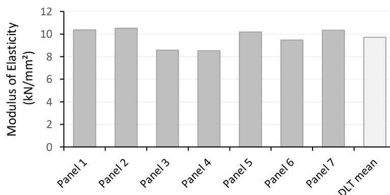
**Figure 8-13: Comparison between stiffness of DLT and similar products.**
