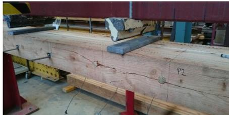
**Figure 8-15: Perpendicular to the grain splitting occurring in the centre of the sample.**
