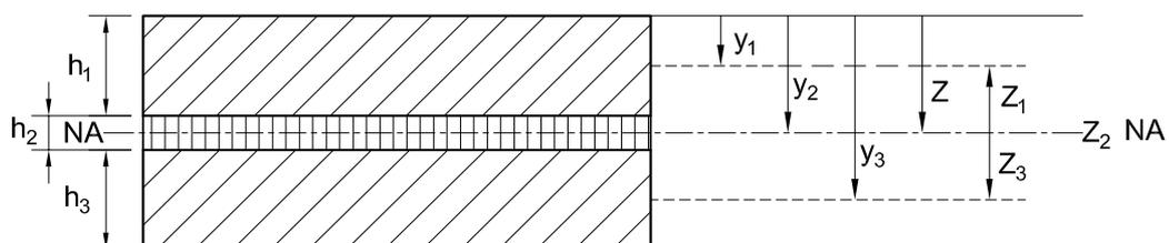
**Figure 8-18: Shear Analogy layers**
