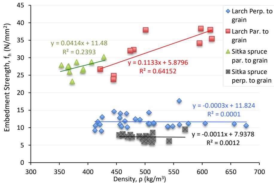
**Figure 6-29: Embedment strength vs. density of all tested samples**
