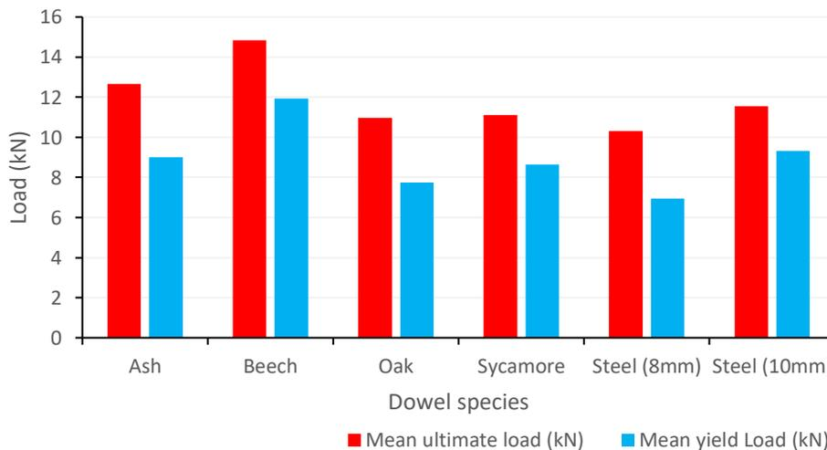
**Figure 7-9: Comparison of the mean yield and ultimate loads of 20.50mm diameter hardwood dowels and 8-10mm mild steel dowels in 30mm diameter larch laminations**
