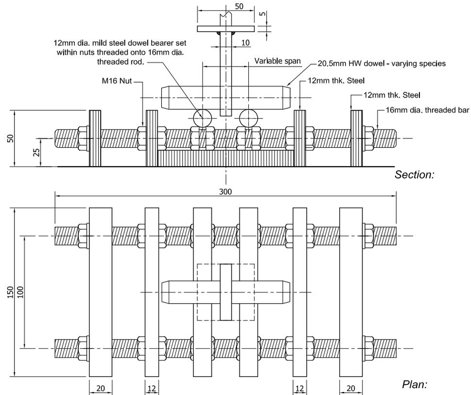
**Figure 6-12: Test rig for testing effective bending stiffness of hardwood dowels.**
