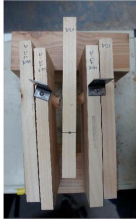
**Figure 7-35: Shear failure of dowel following large rotation.**
