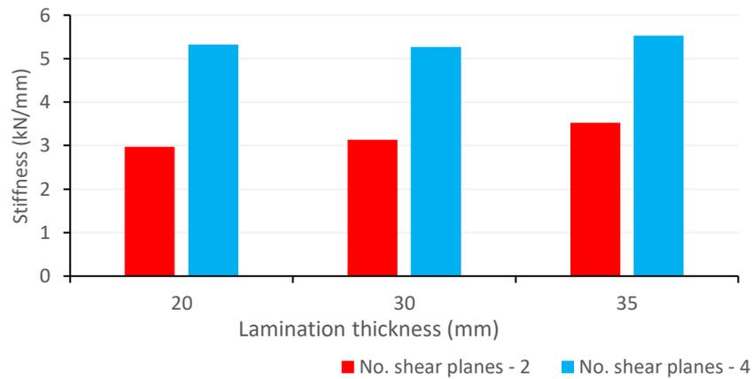
**Figure 7-50: Comparison between the ultimate load of two and four shear plane connections loaded perpendicular to the grain using 20.50mm diameter beech dowels and UK Sitka spruce**
