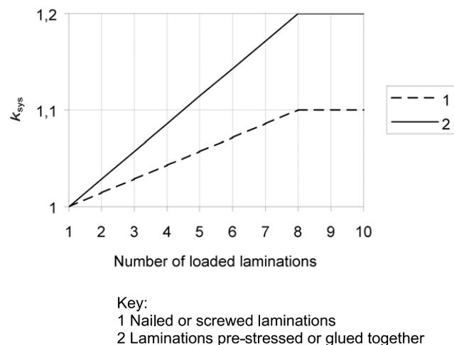
Figure 4-2: System strength factor,  $k_{sys}$  (Figure 6.12, BS EN 1995-1-1, 2004).
