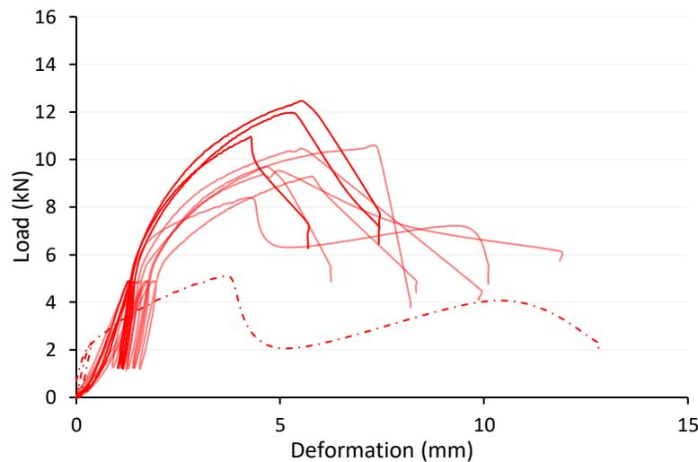
**Figure 7-14: Load deformation curve from testing of B20<sub>par</sub>SS20, illustrating III<sub>m</sub> failure response.**
