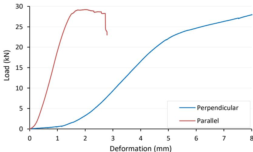
Figure 6-22: Typical load deformation curve for timber embedment.
