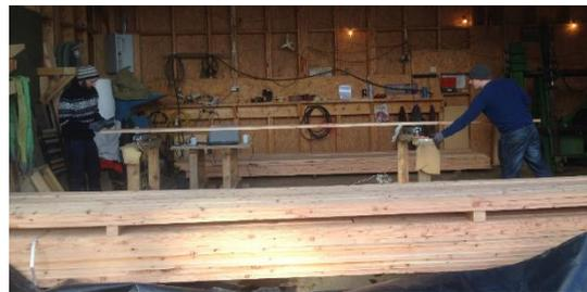
**Figure 8-1: Acoustic grading in progress.**
