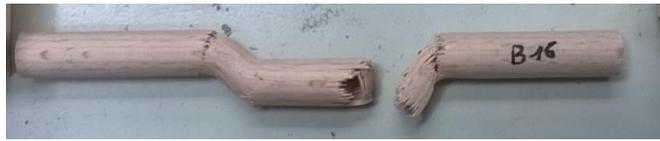
Figure 7-18: Formation of two hinges per shear plane within a dowel during mode IV failure.
