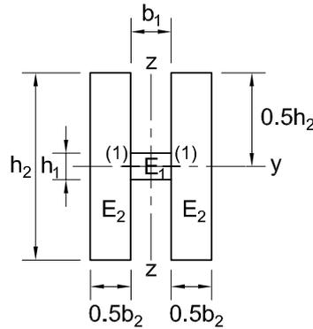
**Figure 4-5: Idealised effective section based on a portion of a DLT panel.**
