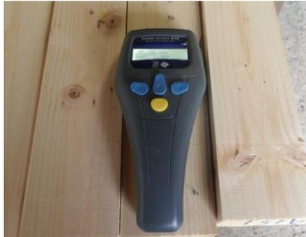
Figure 3-6: Brookhuis Micro-Electronics MTG 960 acoustic grader.
