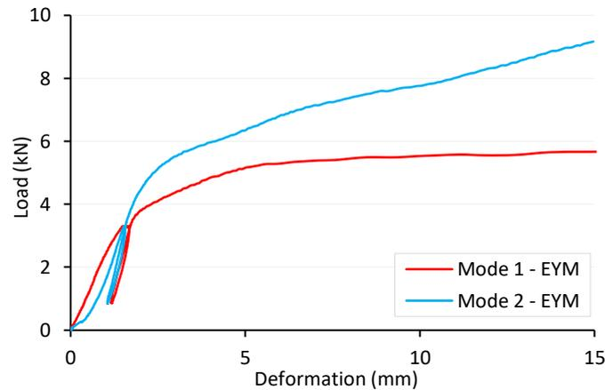
**Figure 7-32: Typical load deformation curves for perpendicular to the grain connection tests using steel dowels - depicting EYM mode 1 & 2 failures.**
