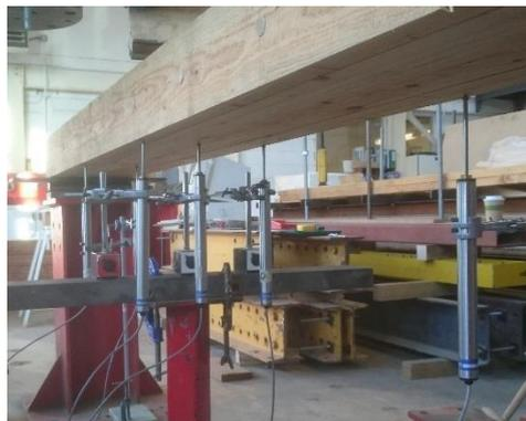
**Figure 8-6: Positioning transducers for three-point bending test.**
