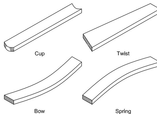
**Figure 3-5: Common distortion types in dried timber**
