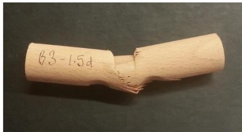
**Figure 6-21: Crushing and bearing failure of a dowel accompanied with brittle tensile failure.**
