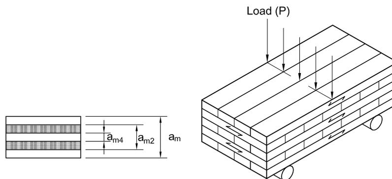
**Figure 4-7: Derivation of composition factor perpendicular to the grain for a 5-layered panel, adapted from Fellmoser and Blass (2004).**
