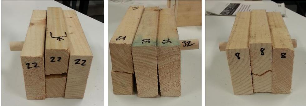
**Figure 7-4: Examples of brittle failure occurring in preliminary testing.**
