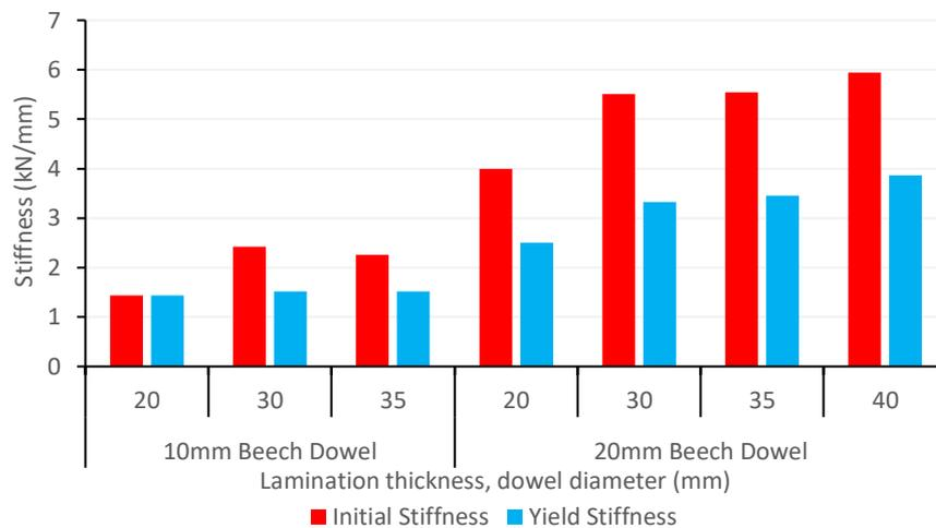
**Figure 7-13: Comparison between the mean yield stiffness and the initial stiffness of beech dowels in Sitka spruce.**
