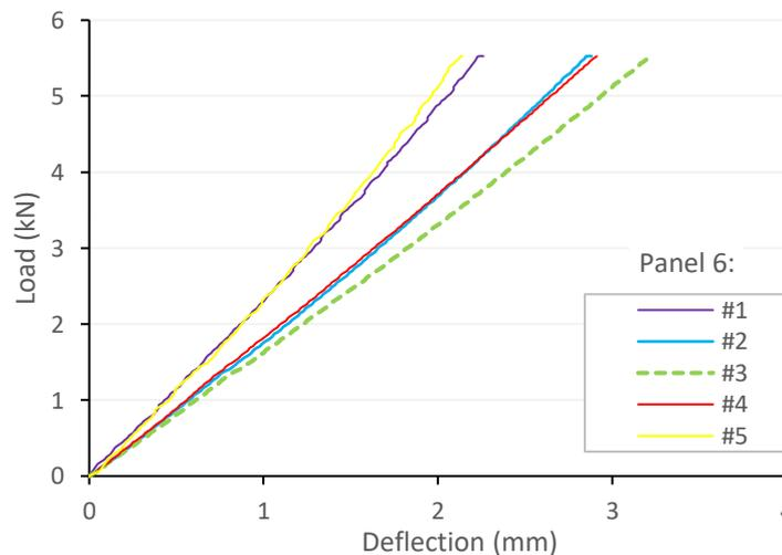
**Figure 8-14: Load deflection curve at differing points of a DLT panel in the elastic range.**
