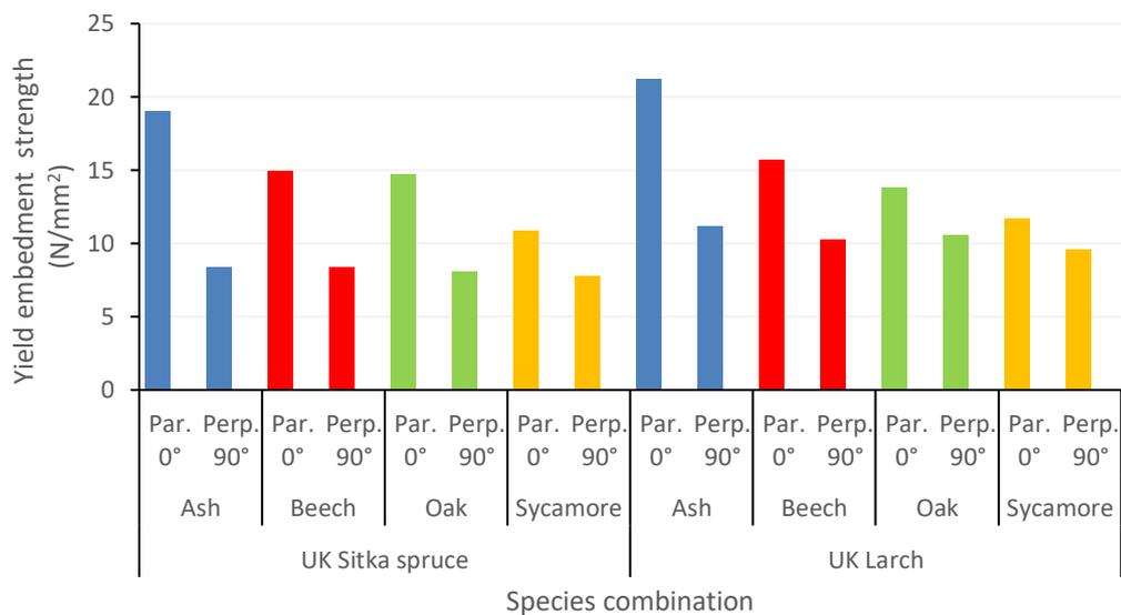
**Figure 6-42: Comparison of the mean yield embedment strength of combined embedment test.**
