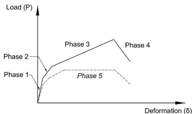
Figure 5-10: Typical load deformation of a mortice and tenon timber dowelled joint, adapted from Shanks, Walker & Harris (2006).
