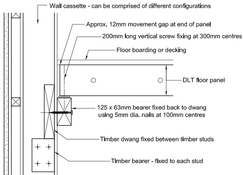
**Figure 9-4: DLT floor panel to wall panel, example detail.**
