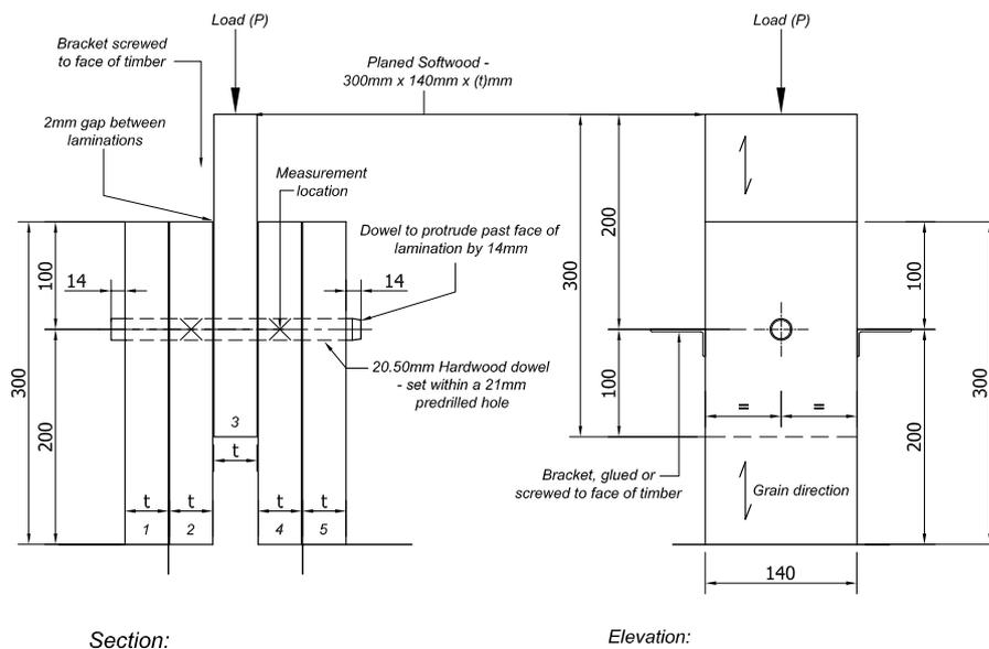
Figure 7-33: Additional shear plane tests parallel to the grain.
