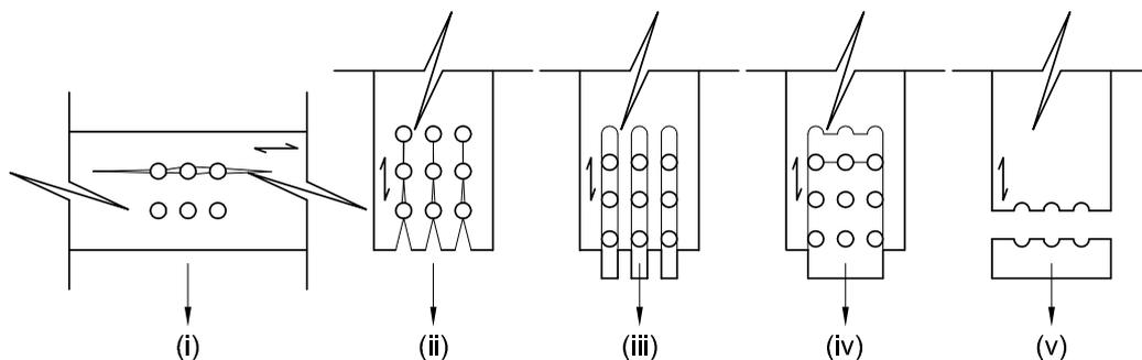
**Figure 5-6: Brittle connection failure, i) perpendicular splitting, ii) in-line splitting, iii) plug shear, iv) group tear-out, v) net tension**
