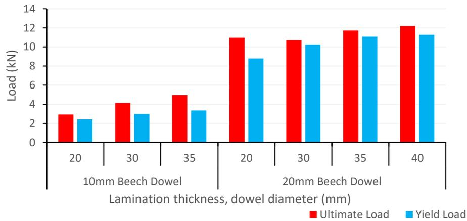
**Figure 7-25: Comparison of the mean ultimate and yield load of beech dowels in UK Sitka spruce perpendicular to the grain.**
