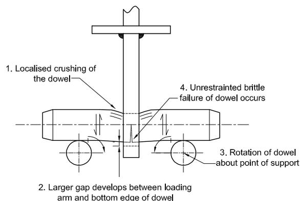
**Figure 6-20: Dowel constraint during loading using bespoke loading arm.**
