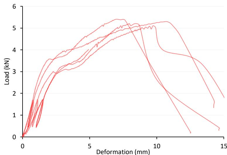
Figure 7-31: Load deformation curve for perpendicular to the grain connection test series B10<sub>perp</sub>SS35 - depicting failure mode IV.
