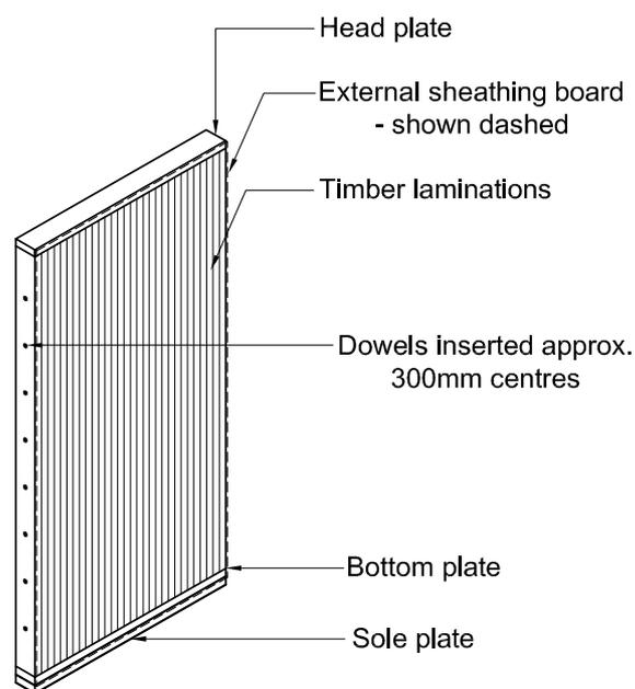
Figure 2-4: Isometric view of an isolated DLT wall panel.
