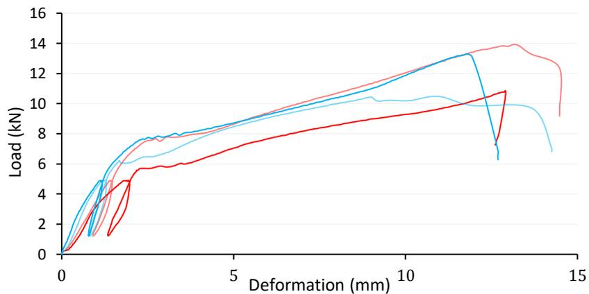
**Figure 7-38: Load deformation curve for 4 plane shear test using 30mm laminations parallel to the grain.**
