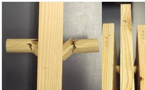
**Figure 7-44: Cross grain shear failure of hardwood dowels.**
