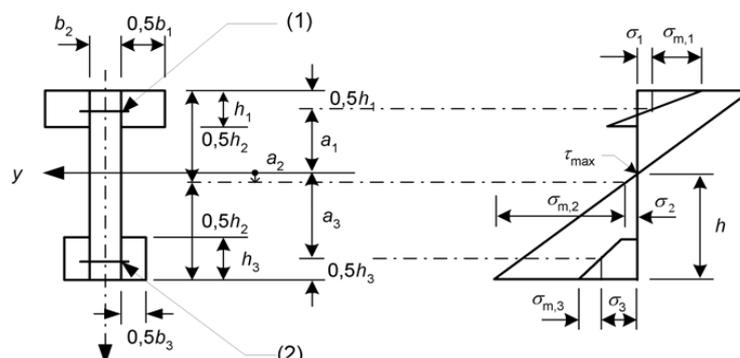
**Figure 4-4: An example compatible cross section, Figure B.1, BS EN 1995-1-1 (2004).**
