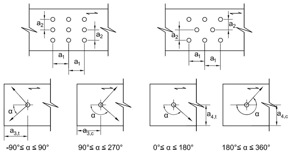
Figure 5-7: Spacing and end and edge distances from BS EN 1995-1-1 (2004).
