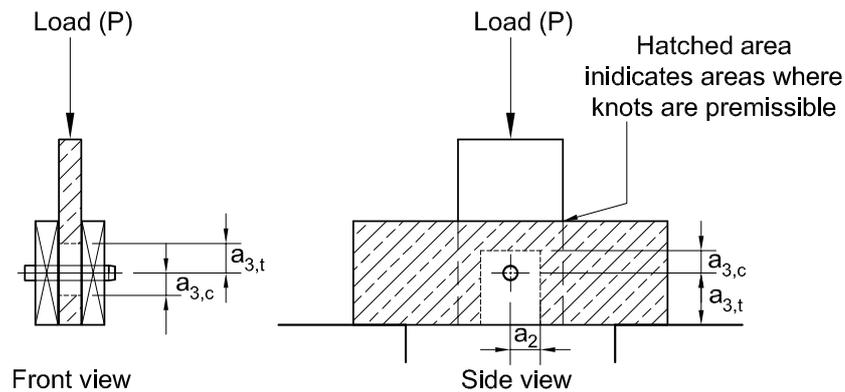
**Figure 7-2: Allowance of knots in perpendicular to grain tests.**
