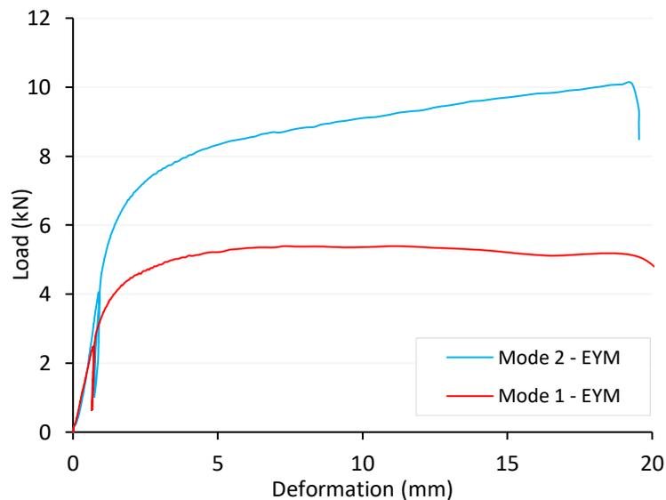
Figure 7-19: Typical load deformation curves from parallel to the grain connection tests using steel dowels - depicting EYM mode 1 & 2 failures.
