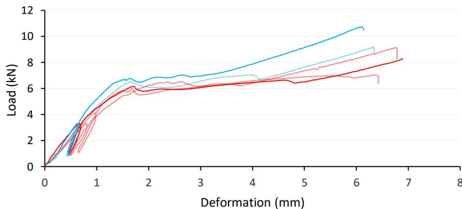
**Figure 7-41: Load deformation curve for 4 plane shear tests using 30m laminations perpendicular to the grain.**
