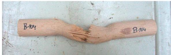
Figure 7-52: Cross grain shear failure of beech dowel.
