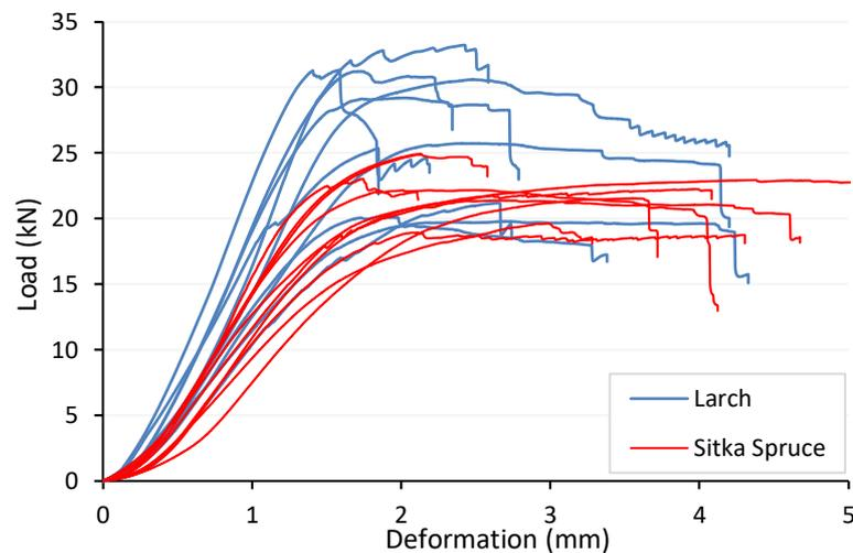
Figure 6-27: Load deformation graph for parallel to the grain embedment using a 20.50mm steel dowel.
