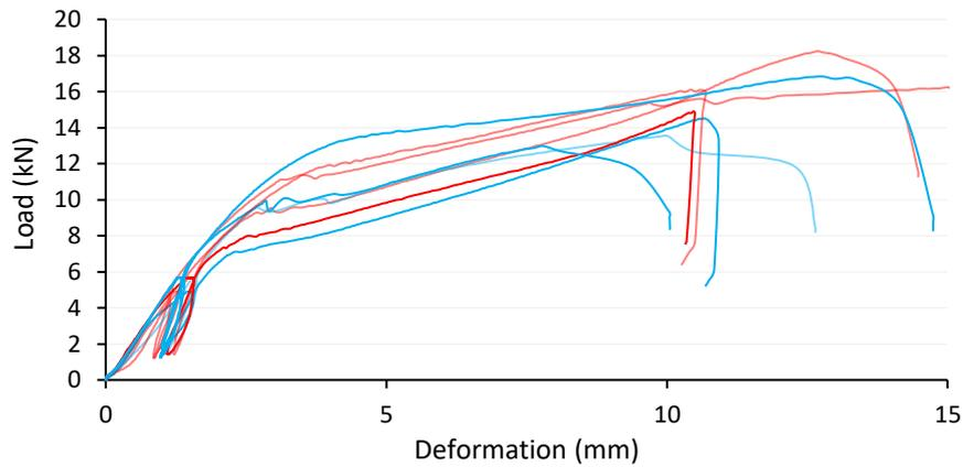
**Figure 7-39: Load deformation curve for 4 plane shear test using 35mm laminations parallel to the grain.**
