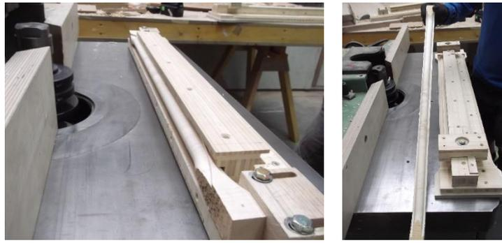
**Figure 3-3: Manufacture of UK hardwood dowel using spindle-moulder**
