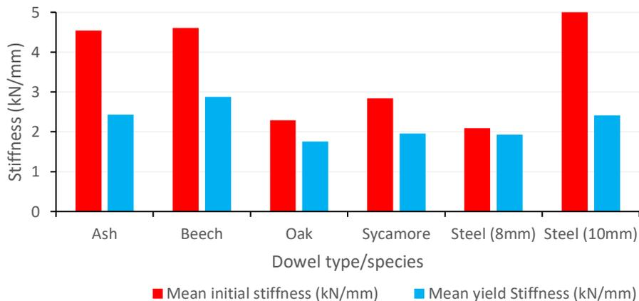
**Figure 7-23: Comparison between the initial and yield stiffness of UK larch in perpendicular to the grain connections.**
