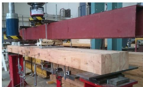
Figure 8-8: Four point bending set-up.
