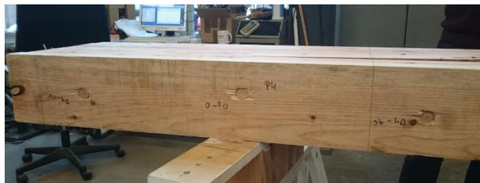
**Figure 8-17: Non-alignment of dowel insertion during production.**
