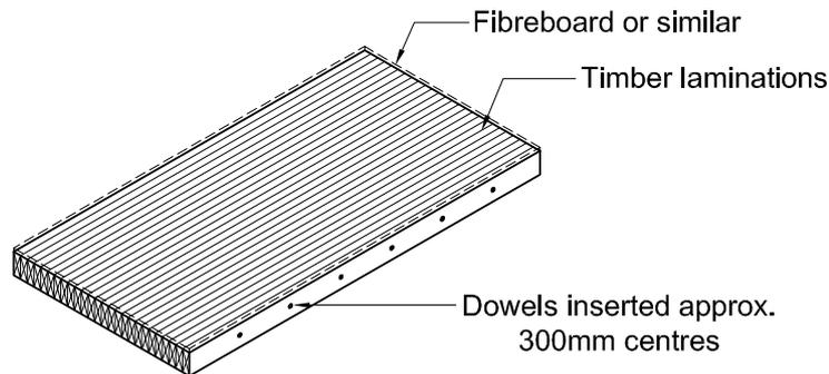
**Figure 2-5: Isometric view of a DLT floor panel.**
