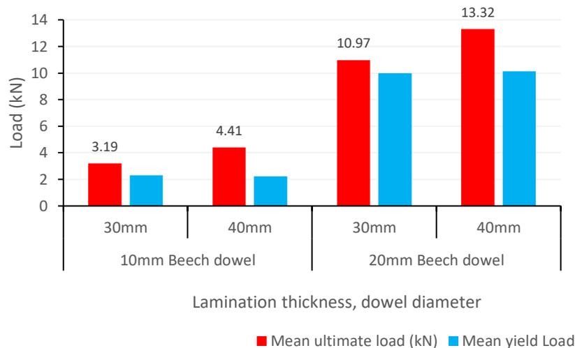
**Figure 7-24: Comparison of the mean yield and ultimate load of beech dowels in UK larch with varying diameter and thickness.**
