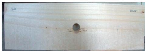
**Figure 7-30: Localised embedment failure in a side lamination.**
