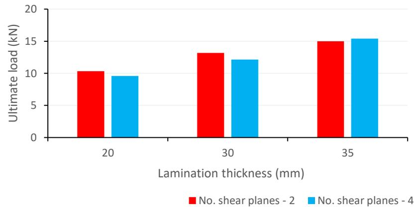
**Figure 7-49: Comparison between the ultimate load of two and four shear plane connections loaded parallel to the grain using 20.50mm diameter beech dowels and UK Sitka spruce.**
