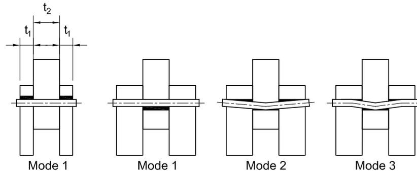
**Figure 5-3: Failure modes for a dowel-type fastener in a double shear arrangement according to BS EN 1995-1-1 (2004).**
