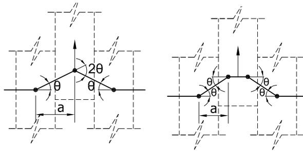
**Figure 5-11: Development of 3 or 4 plastic hinges in a timber dowel connection.**
