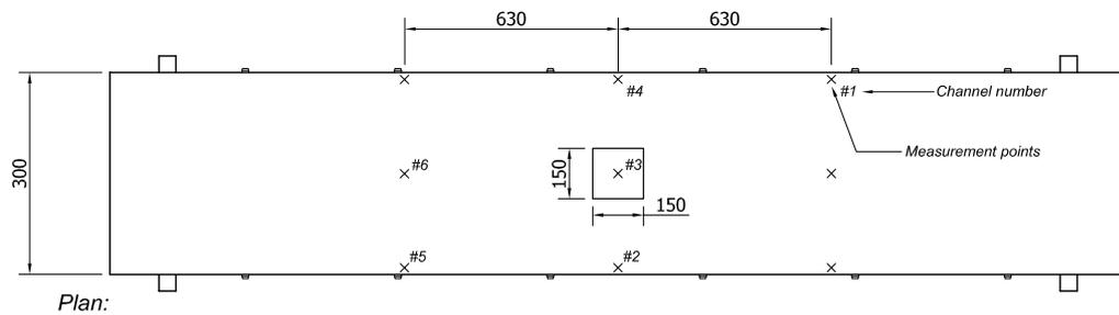
**Figure 8-9: LVDT location on three-point load test.**
