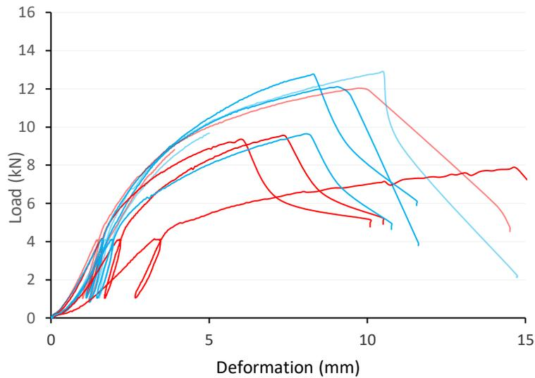
**Figure 7-28: Load slip response curves from perpendicular to the grain testing of series B20<sub>perp</sub>SS20 illustrating failure mode I<sub>m</sub>.**
