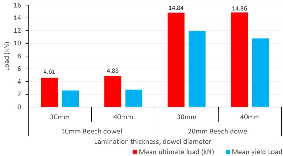
**Figure 7-10: Comparison of the mean yield and ultimate load of beech dowels in UK larch with varying diameter and thickness.**
