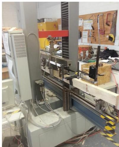
Figure 6-1: Four-point bending test on UK Sitka spruce.
