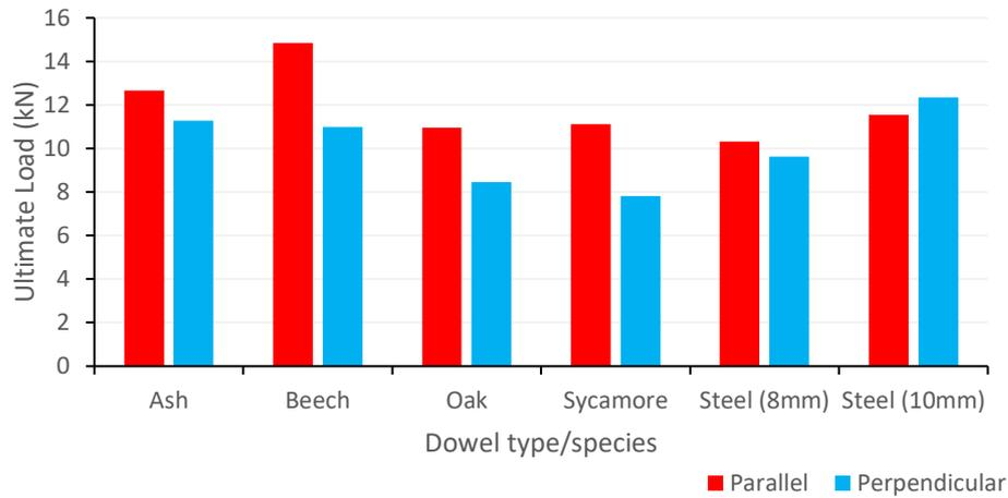
**Figure 7-22: Comparison between the ultimate load capacity of 20.5mm diameter hardwood dowels and mild steel dowels in both the parallel and perpendicular to grain orientation.**
