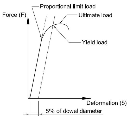
**Figure 6-15: Determination of the yield load using the 5% dowel diameter offset method.**
