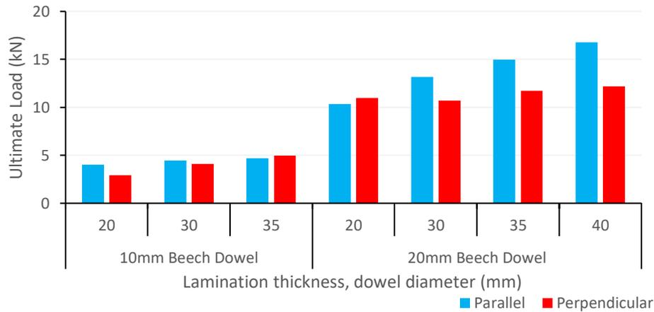
**Figure 7-27: Comparison between parallel to grain connections and perpendicular to grain connections using UK Sitka spruce.**
