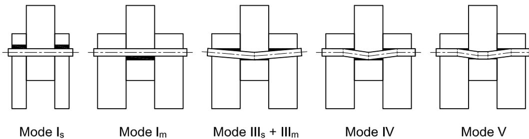
**Figure 5-9: Failure modes of double shear plane connections using timber dowels.**
