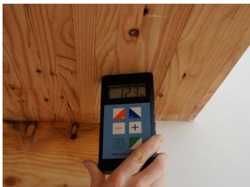
**Figure 9-3: Handheld moisture content reading of DLT panel in-situ.**
