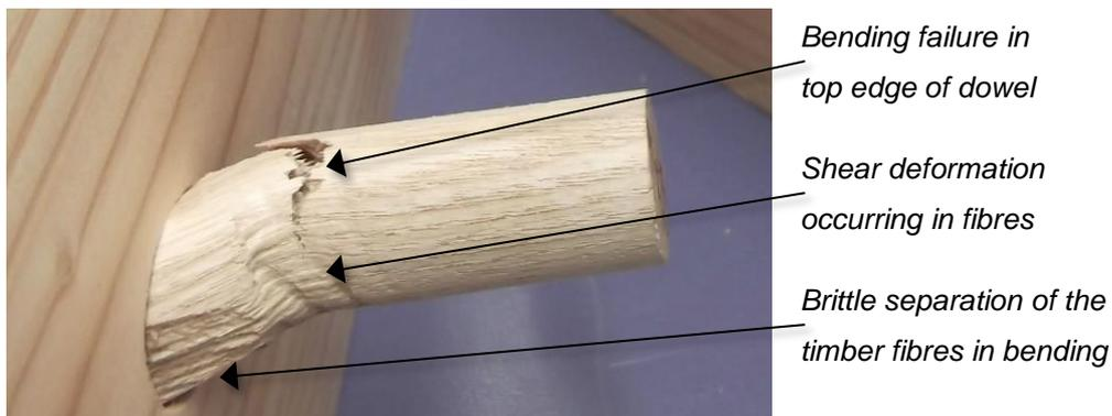
**Figure 7-47: Failure of a timber dowel.**
