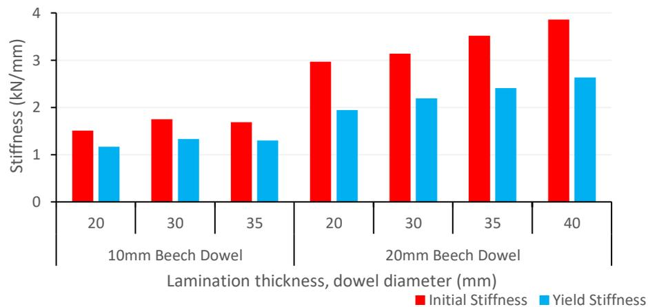
**Figure 7-26: Comparison between the mean yield stiffness and the initial stiffness of beech dowels in Sitka spruce perpendicular to the grain.**
