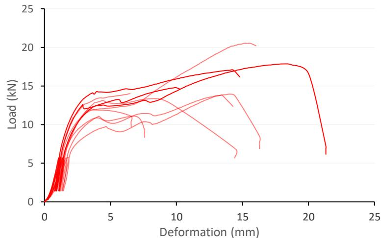
**Figure 7-15: Load deformation curve from testing of B20<sub>par</sub>SS35 illustrating  $V_d$  failure response.**
