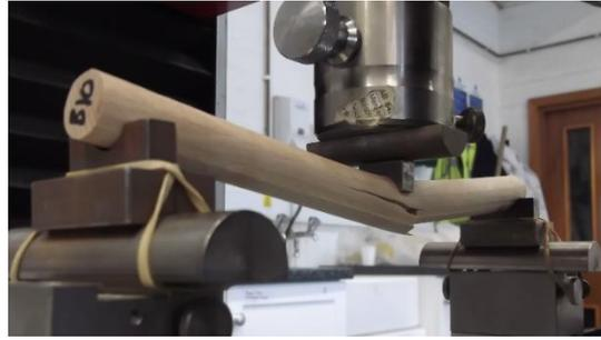
**Figure 5-12: Typical brittle tensile failure experienced by timber dowel undergoing three-point bending**
