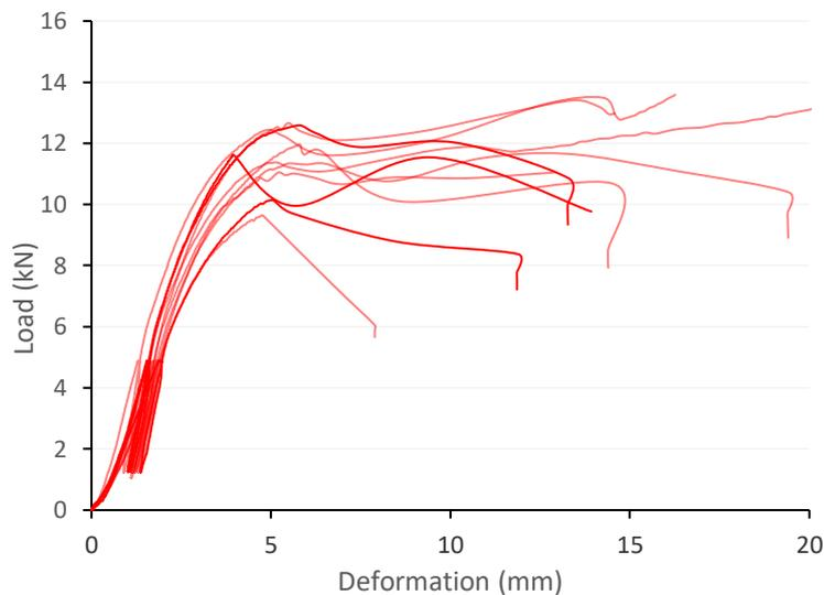
**Figure 7-29: Load deformation curves from perpendicular to the grain testing of B20<sub>perp</sub>SS35 illustrating III<sub>m</sub> failure.**
