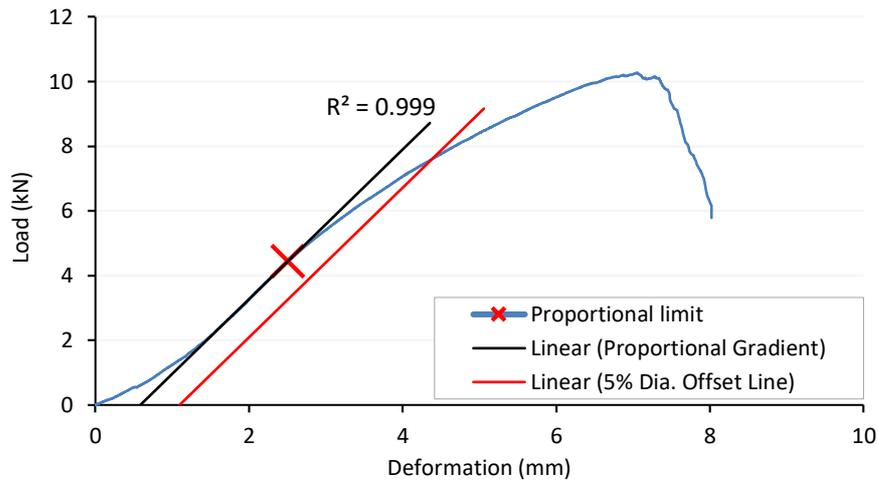
**Figure 6-18: Load deformation curve of an ash dowel, with a shear span (a) of 0.5D illustrating early signs of crushing and embedment at supports.**
