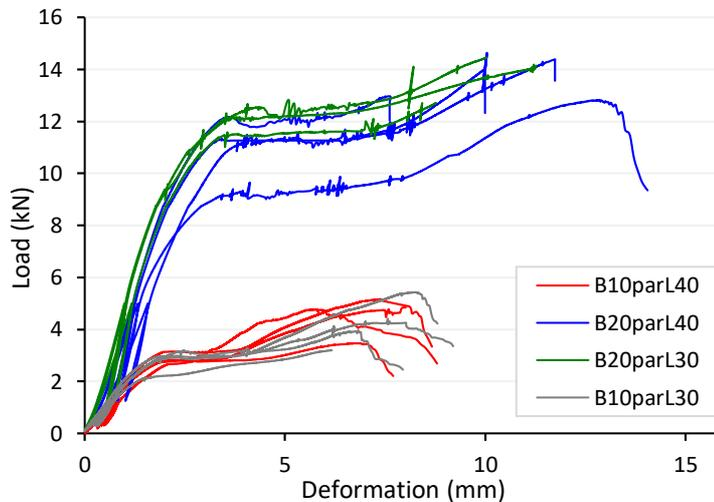
**Figure 7-11: Load deformation curves for parallel to grain double shear plane connection tests using beech dowels and UK larch.**
