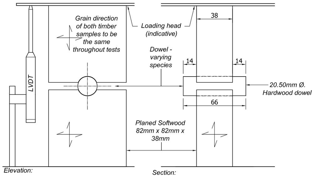
**Figure 6-31: Combined embedment test setup (adapted from Church and Tew, 1997).**
