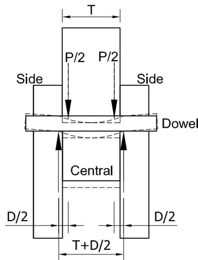
Figure 5-15: Dowel modelled as a simply supported beam, adapted from Sandberg Bulleit & Reid (2000).
