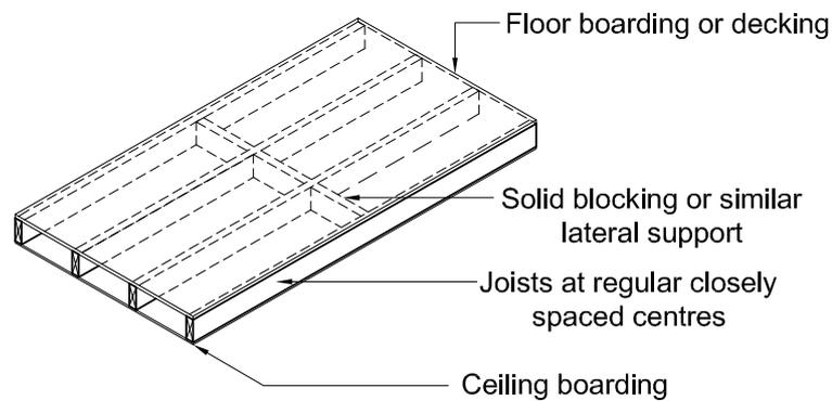
Figure 4-1: Typical suspended timber floor
