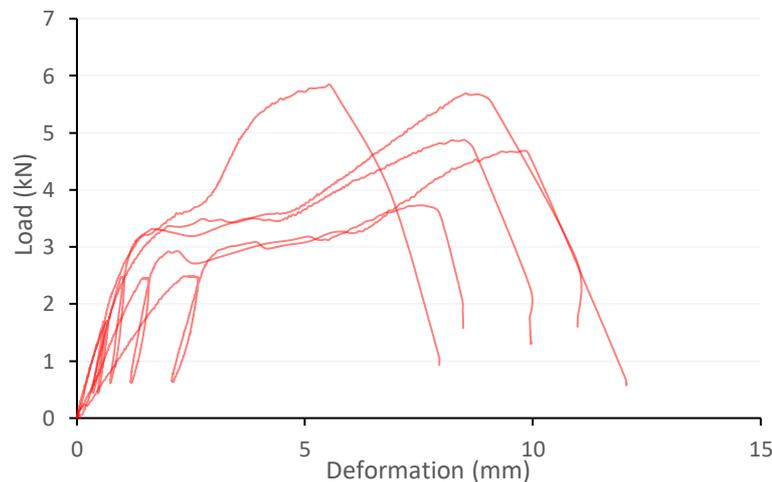
Figure 7-17: Load deformation curve from testing of  $B_{10\text{par}}SS35$  illustrating IV failure.
