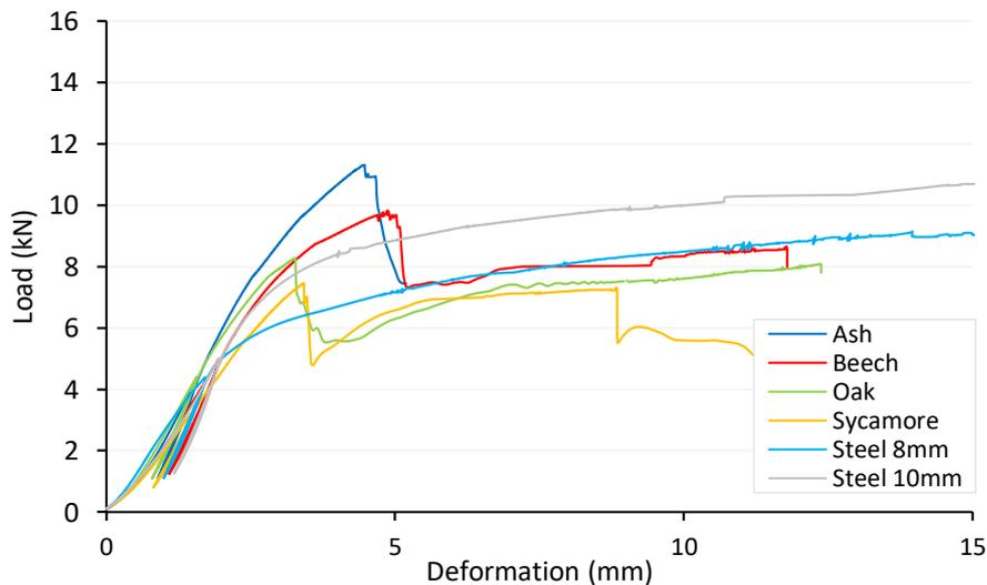
Figure 7-20: Typical load slip response of selected 20.50mm diameter hardwood dowel and mild steel dowel fasteners in perpendicular to the grain double shear connection tests using UK larch.
