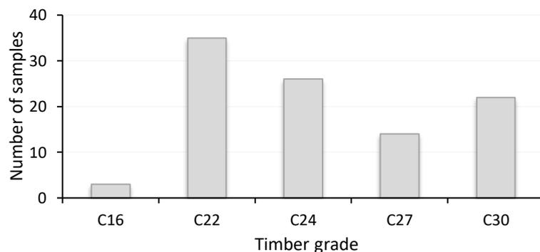
**Figure 8-2: Results of acoustic grading on subset of the UK larch provided.**
