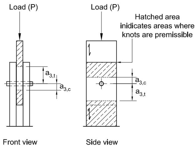
**Figure 7-3: Allowance of knots in the parallel to grain tests.**
