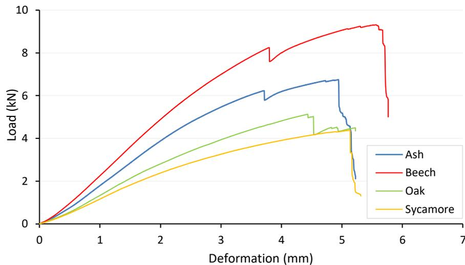
**Figure 6-16: Typical load deformation plots for select hardwood dowels at 2.5D span under three-point bending**
