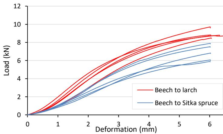
**Figure 6-39: Combined perpendicular embedment – Beech**
