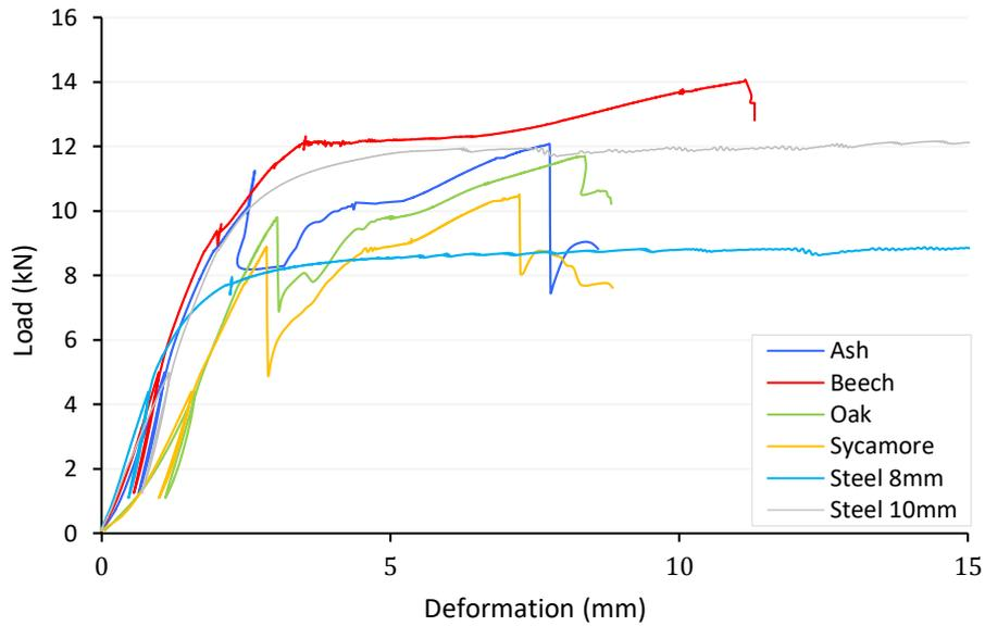
**Figure 7-8: Typical load slip response of selected 20.50mm diameter hardwood dowel and mild steel dowel fasteners in parallel to the grain double shear connection tests using UK larch.**
