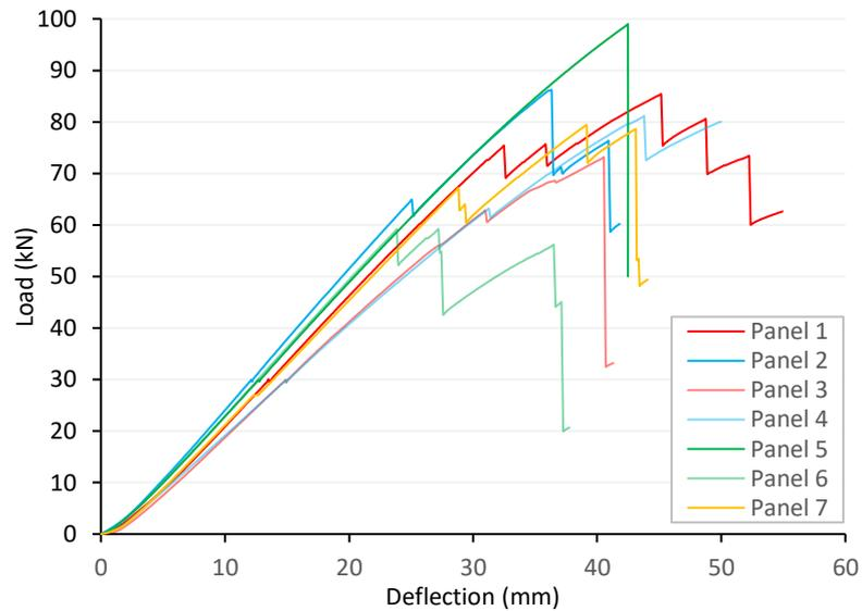
**Figure 8-10: Load deformation plot of UK larch DLT panels under four-point bending.**
