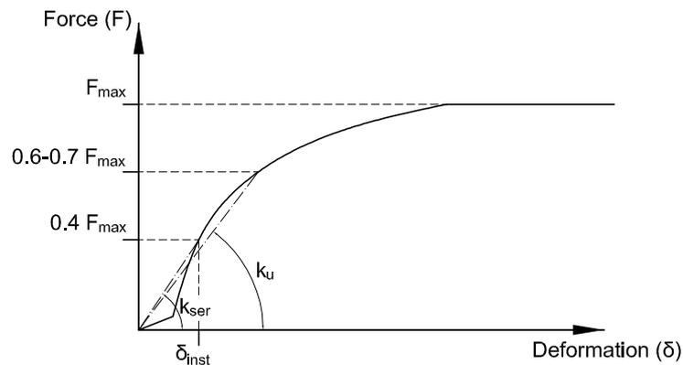
**Figure 5-13: Typical load slip curve for a bolted connection.**
