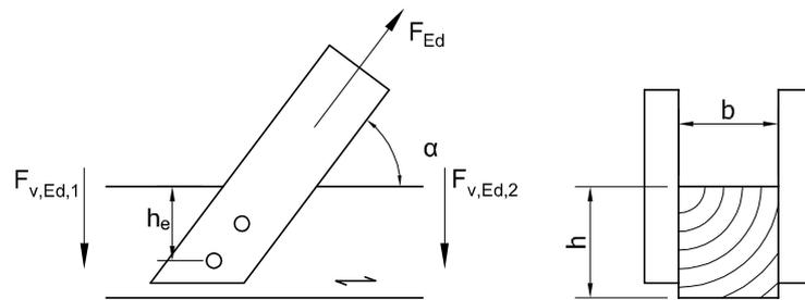
**Figure 5-8: Perpendicular to grain geometry, BS EN 1995-1-1 (2004).**
