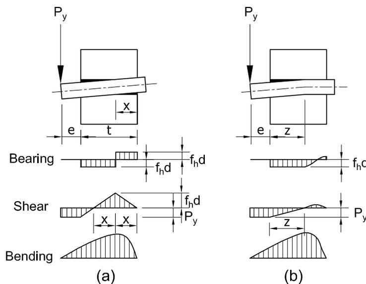
**Figure 5-1: General modes of failure of metallic dowels (Larsen, 1979).**
