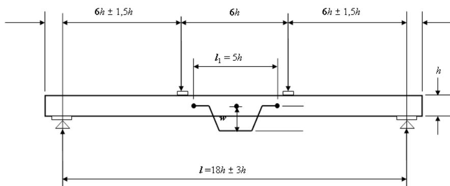
Figure 6-2: Testing arrangement for measuring the local modulus of elasticity in bending (Figure 1, BS EN 408, 2010, p.9).
