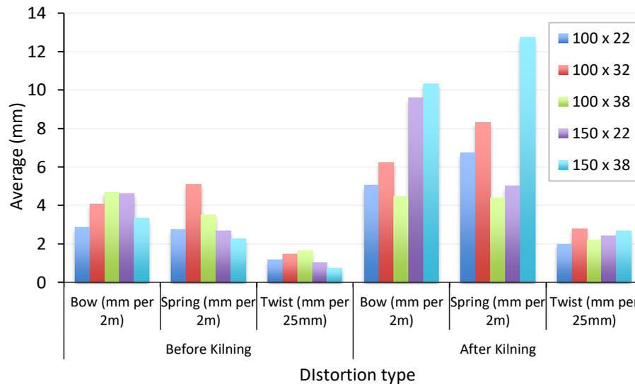
**Figure 6-9: Mean distortion of Scottish Sitka spruce before and after kilning.**
