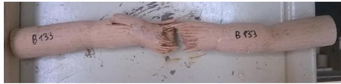
**Figure 7-37: Shear failure of beech dowel with accompanying embedment.**
