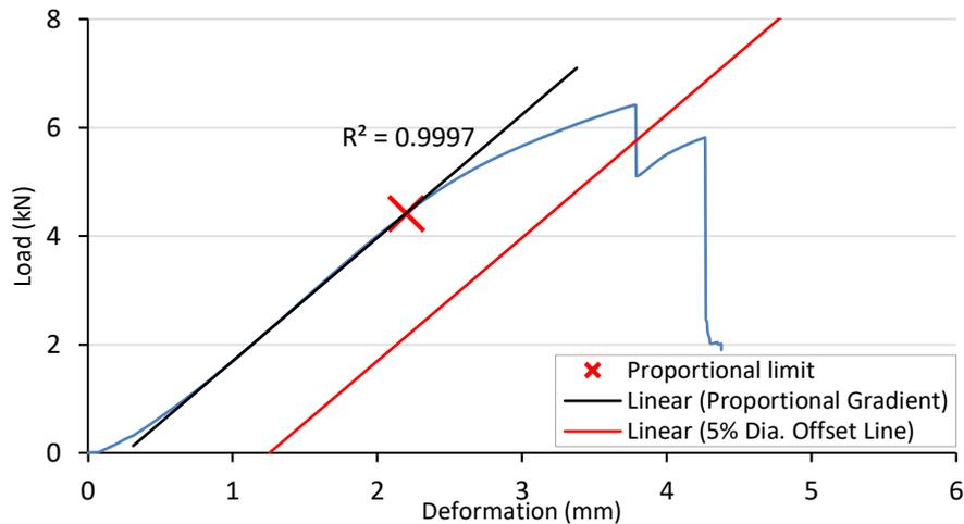
**Figure 6-19: Load deformation curve of an ash dowel, with a shear span (a) of 1.25D, illustrating wedging occurring after the ultimate load is reached.**
