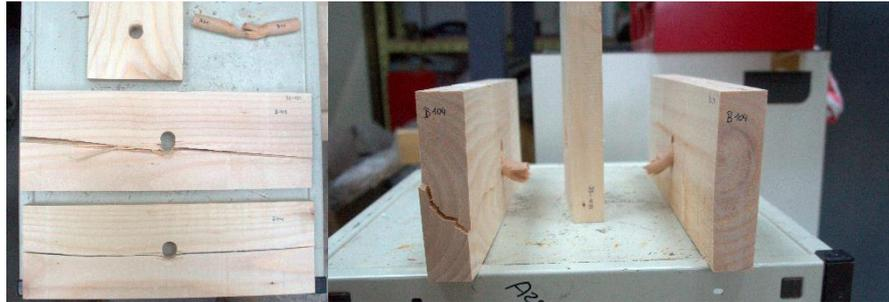
**Figure 7-51: Perpendicular to the grain splitting of the side members.**
