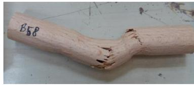
Figure 7-16: Irregular formation of hinges within in Beech dowel during  $V_d$  failure.
