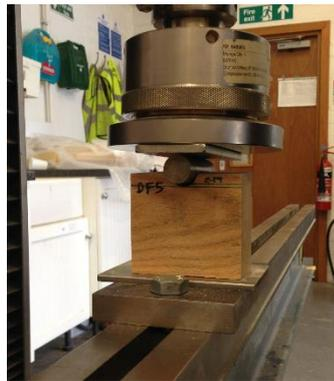
**Figure 6-26 Perpendicular to grain embedment testing**
