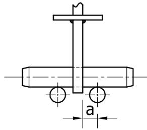
Figure 6-13: Shear span of dowel.
