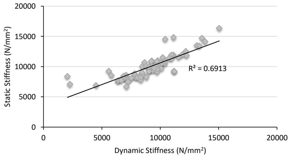
**Figure 6-5: Dynamic Elastic Modulus Vs. Static Elastic Modulus of UK Sitka spruce.**
