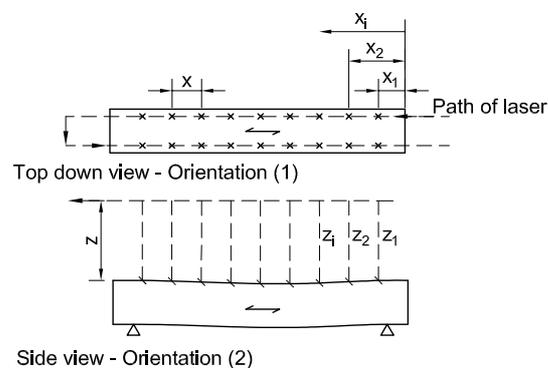
**Figure 6-7: Process of measuring deformation using a FRITS frame.**
