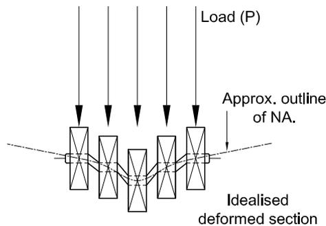
**Figure 4-6: Deformed idealised section.**
