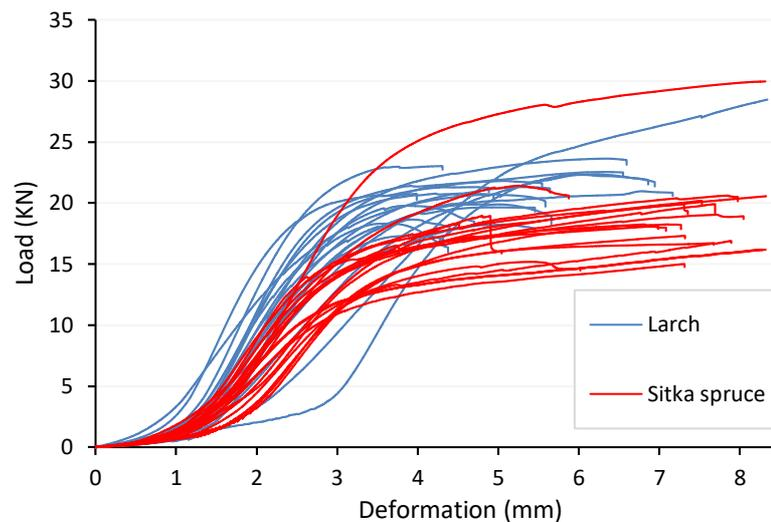
**Figure 6-28: Load deformation curves for perpendicular to the grain embedment using a 20.50mm steel dowel.**
