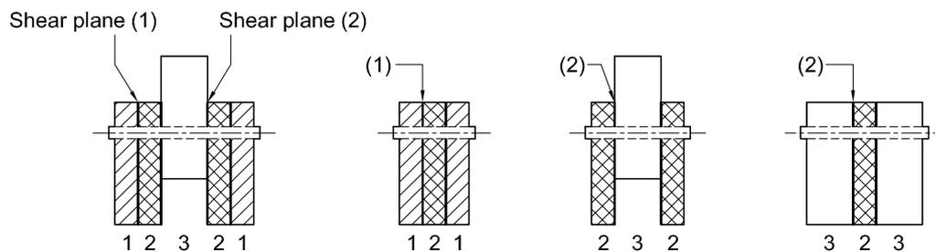
**Figure 5-5: Formation of symmetrical three-member connection assemblies (adapted from Porteous and Kermani, 2013).**
