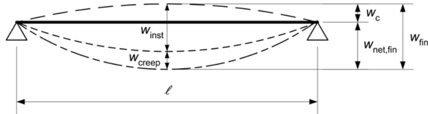
Figure 4-3: Components of deflection, Figure 7.1, BS EN 1995-1-1 (2004).
