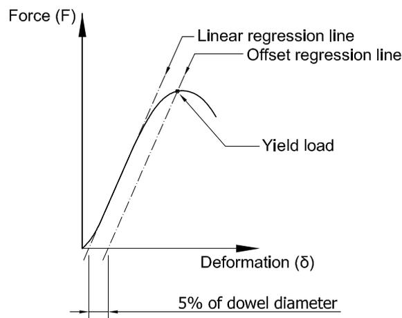
Figure 6-23: Derivation of yield load from load deformation plot.
