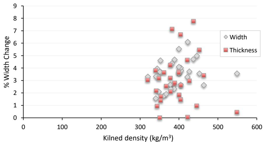
**Figure 6-8: Relationship between density and % change of width of South Scotland Sitka spruce during kilning.**
