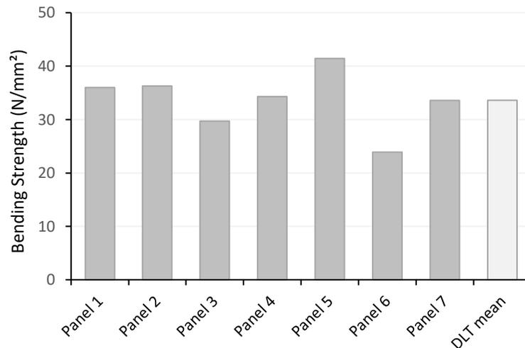
**Figure 8-12: Comparison between bending strength of DLT.**
