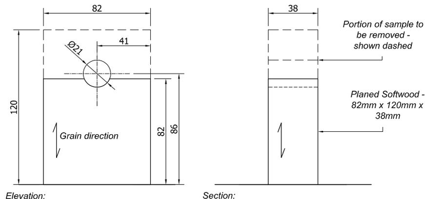
**Figure 6-24: Schematic view of sample preparation**
