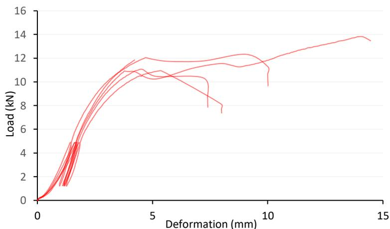
**Figure 7-48: Load deformation curve from perpendicular to the grain connection tests series B20<sub>perp</sub>SS40.**
