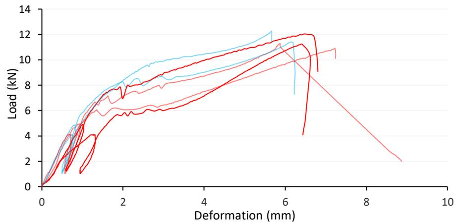
**Figure 7-42: Load deformation curve for 4 plane shear tests using 35mm laminations perpendicular to the grain.**
