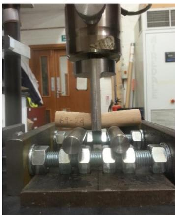
**Figure 6-14: Adapted three-point bending test in operation**
