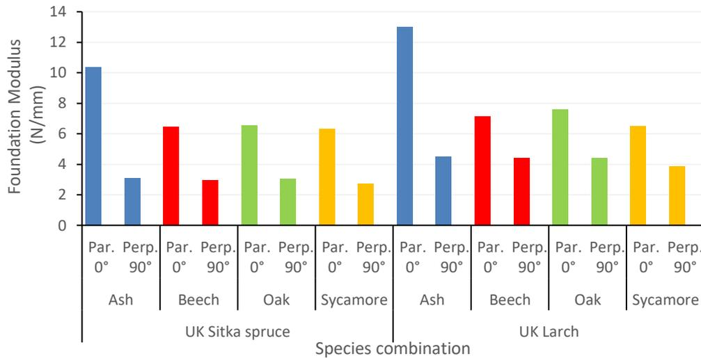
**Figure 6-43: Comparison of the mean foundation moduli of combined embedment tests.**
