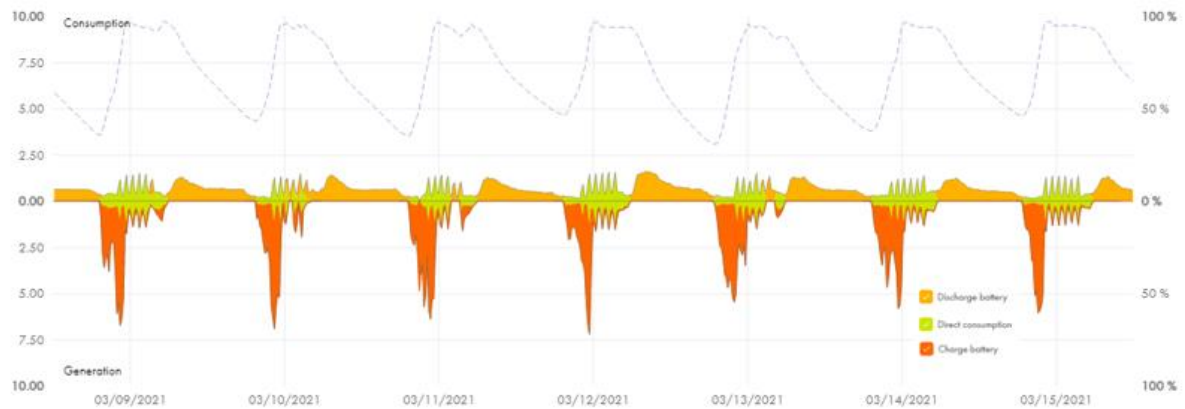
Figure 49 Battery state of charge and power drawn by battery, week beginning 09/03/21
