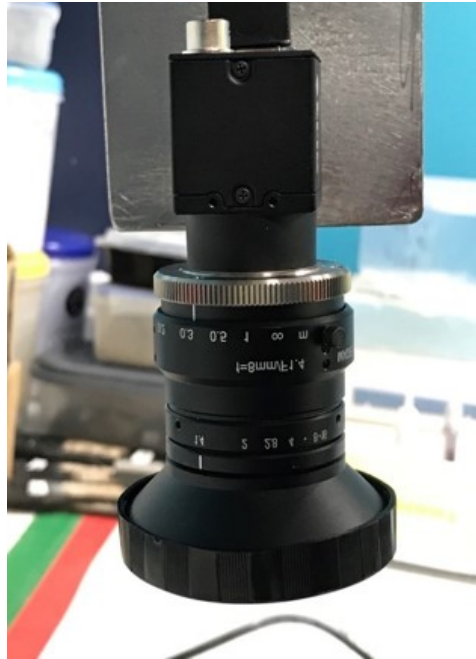
Figure 4.4: FLIR Blackfly 1" sensor machine vision camera.
