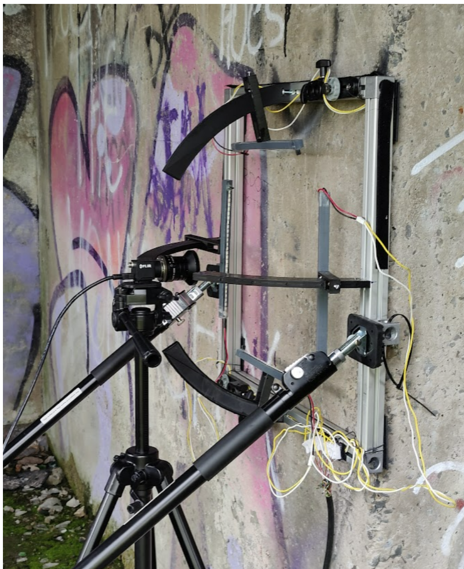
Figure 1: First Iteration of Handheld and Portable ALICS Hardware. Captures images of size 5429 \times 3458 pixels.
