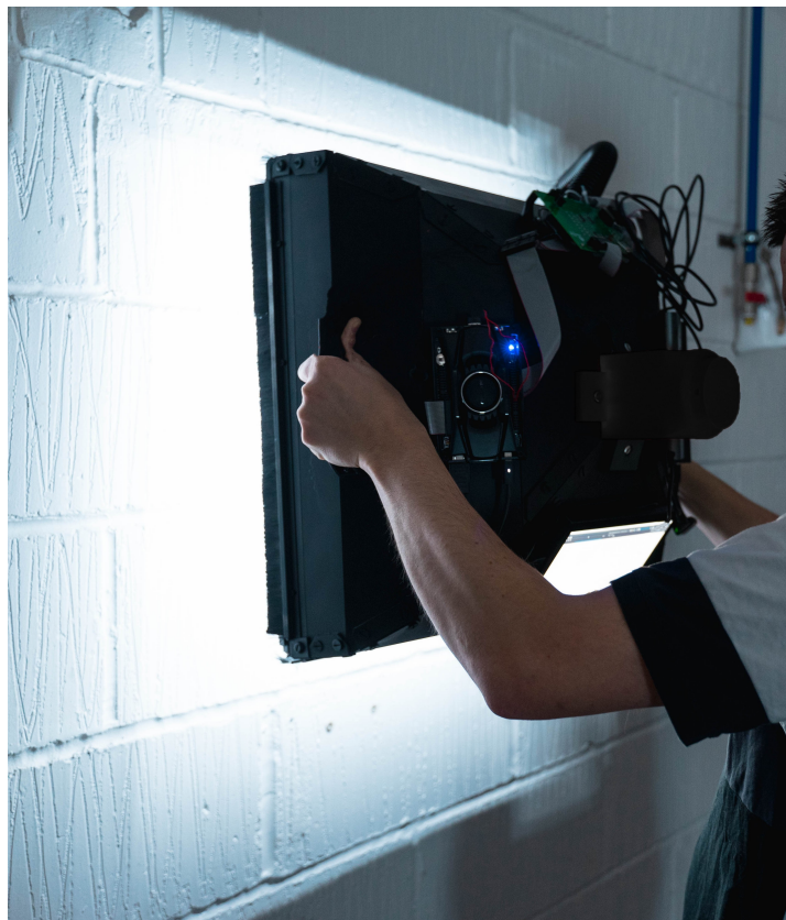
Figure 3: Second iteration of ALICS's hardware, along with the directional lighting prototype, demonstrates its utility as a handheld device designed for manual inspection. Captures images of size 5429 \times 3458 pixels.
