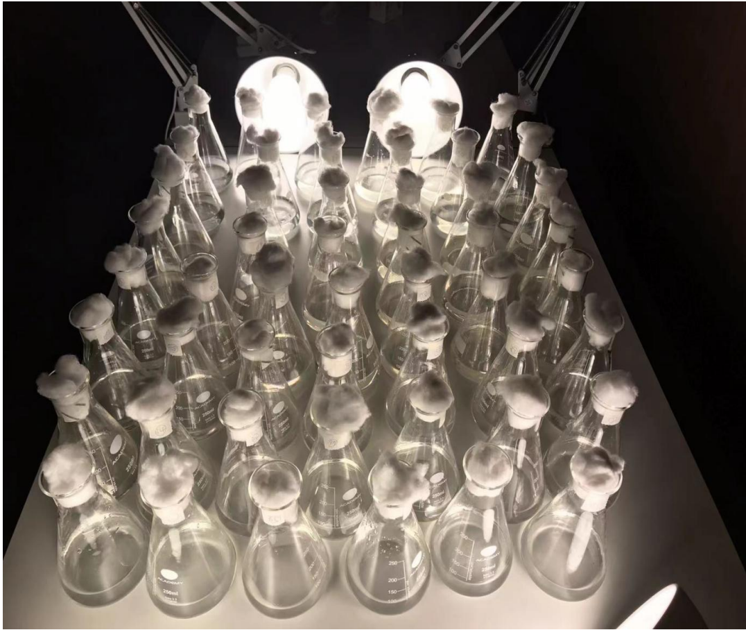
Figure I. Growing flasks of experiments in Section 6.7.1 at Day 0. The light intensity was not measured in this experiment, however, there are gaps between these flasks and the parameters of lamps are the same, thus the light intensity could be considered as the same.
