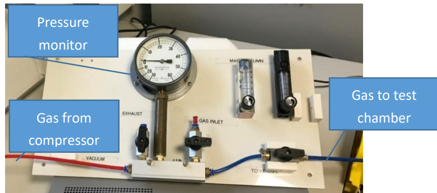
Figure (6.5.4) Air Compressor from ThorLab and gas monitoring board
