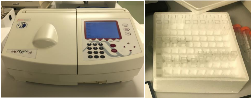
Figure (6.5.6) Thermo Spectronic Biomate 5 spectrometer and 5 mL measurement cuvettes.
