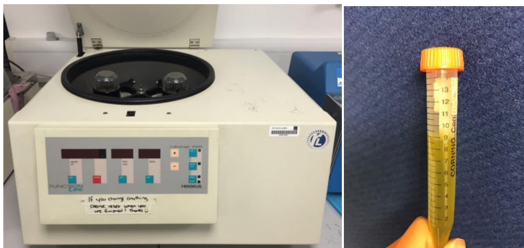
Figure (6.6.2) Heraeus Labofuge 400R centrifuge and centrifuged sample
