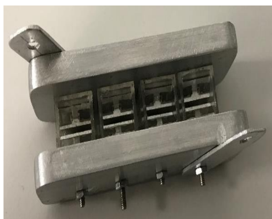
Figure (6.2.1.2) Modified electroporation cuvette and 4-parallel cuvettes.
