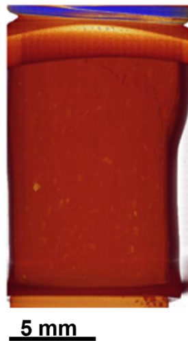
Figure 11: Shear band formation: mica marker configuration, a) before shear b) after shear c) image of sample 4MV after scan
