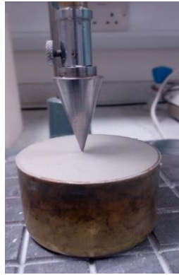
Figure 8: a) Convex muscovite silt surface (pH 8) in a penetrometer cup b) silt sized muscovite mixed with acidified water (pH 5) with flat surface in a penetrometer cup.
