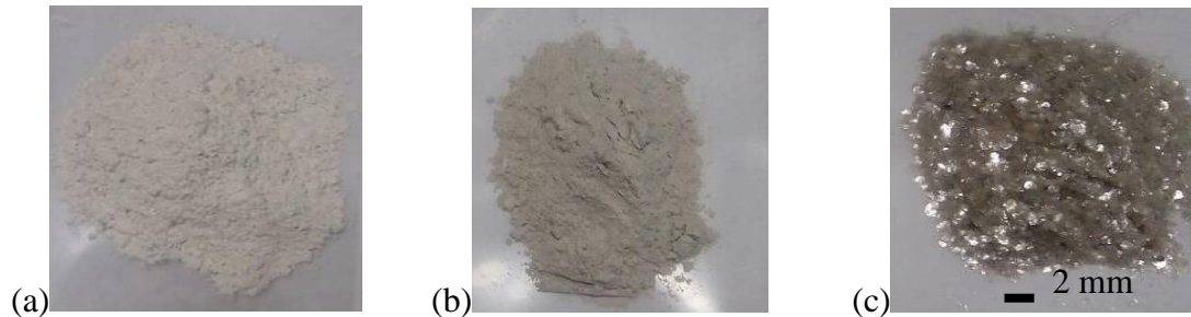
Figure 1. Images of (from left to right) kaolin, muscovite silt and muscovite sand used in this study.
