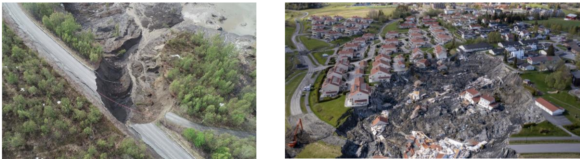
Figure 1: a) Alta Landslide which occurred on the 3 rd of June 2020 in a body of clay, destroys road in Northern Norway (adapted from www.lifeinnorway.net on the 30 th of May 2021) b) Drone image showing the landslide site at Ask in Gjerdrum municipality, Norway after a deadly landslide on the 30 th of December 2020 (adapted form www.world-today-news.com on the 30 th of May 2021).
