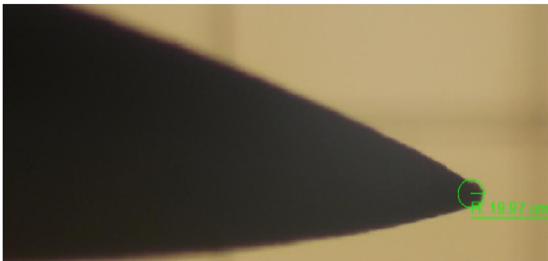
Figure 4-14 Sharpened tip of the gramophone needle used as the HV electrode
