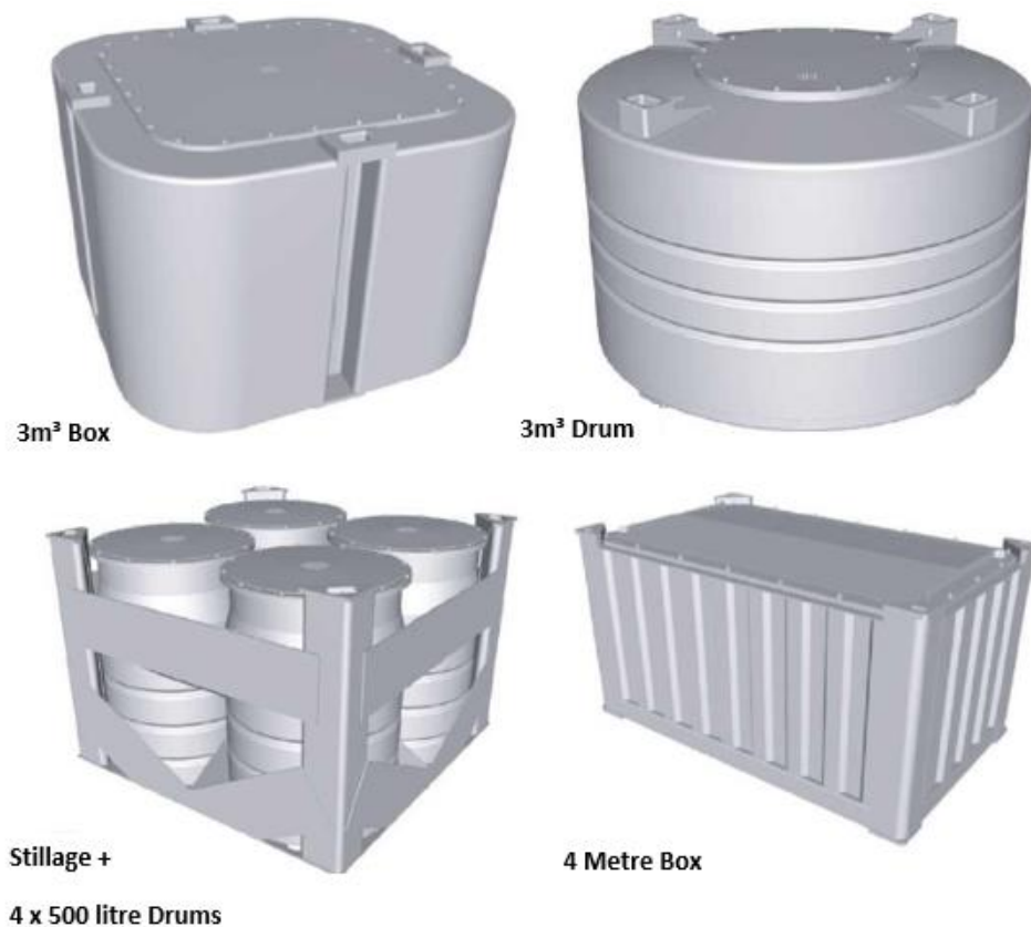
Figure 3: NIREX ILW standard containers[11].
