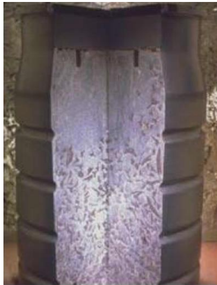
Figure 23:ILW immobilising cementitious matrix [16].
