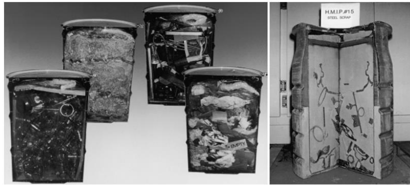
Figure 131: Left-Cut views of nuclear waste drums containing different types and layouts and of nuclear decommissioning products [132]. Right- Metallic scrap material embedded in immobilising cementitious matrix inside an ILW 500 L drum [132]
