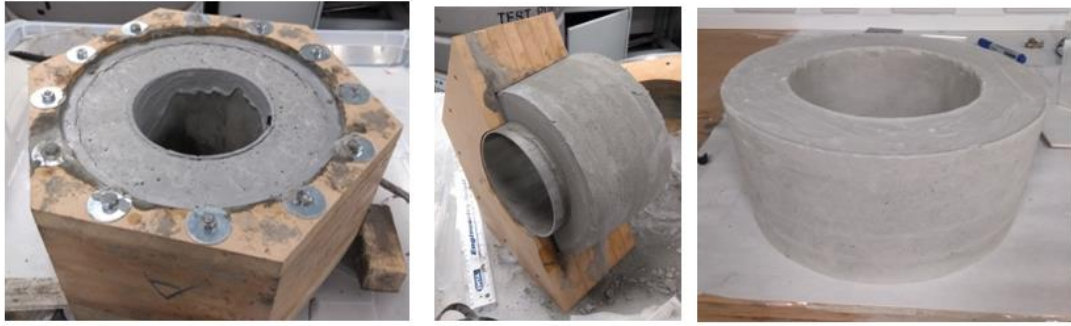
Figure 159: 7 piece wooden mould and cement moulding release.
