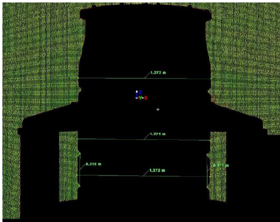
Figure 22: Measurements from the drum silhouette shadow metrology [6].
