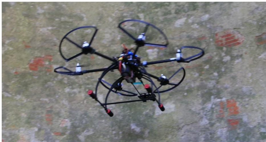
Figure 64: Dexterous Hexrotor with sampling arm for physical samples from inside a cylindrical grain silo in a mock-up of the WIPP exhaust shaft [83].
