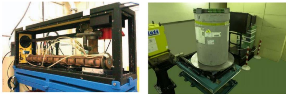
Figure 40: (Left) Linac Mini-Linatron Varian. Electrons are accelerated from the left (electron gun side) to the right (target side). The length of accelerating cavity is 1.2 m [30]. (Right) Example of waste drum in concrete package in front of an X-ray detector [31].
