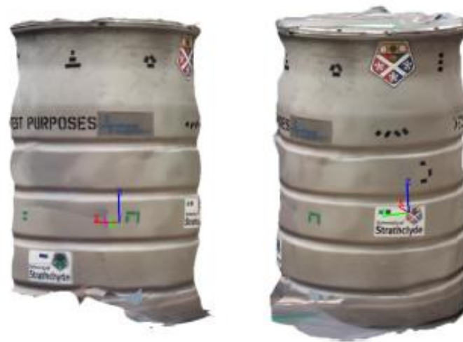
Figure 45: Three-dimensional surface-mesh of a 500 L ILW drum created using from UAV deployed camera photogrammetry [83].
