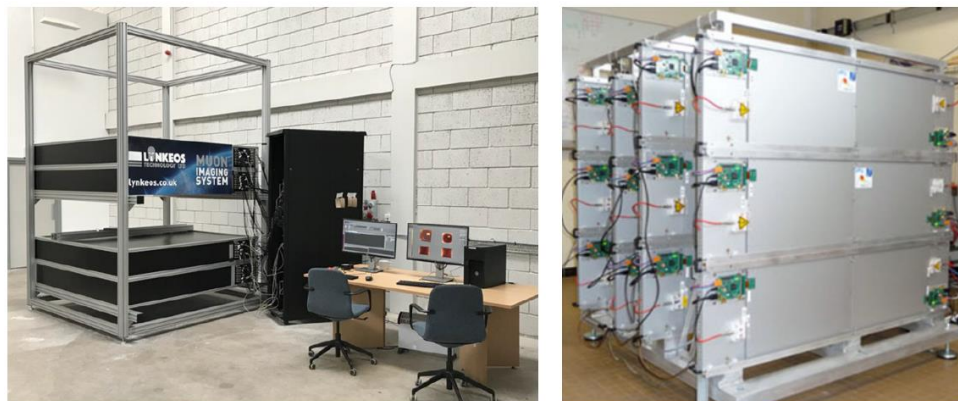
Figure 41: (Left) The Lynkeos Muon static Imaging System installed at the Lynkeos Technology fabrication facility, used to scan ILW containers [64]. (Right) MURAY mobile muon telescope [63].
