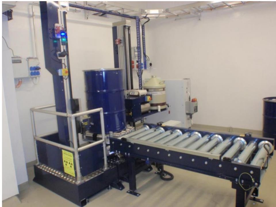
Figure 18: WR-SGS, Model G3250-200) machine used to inspect medium size nuclear waste containers for external damage and radiation levels [29].
