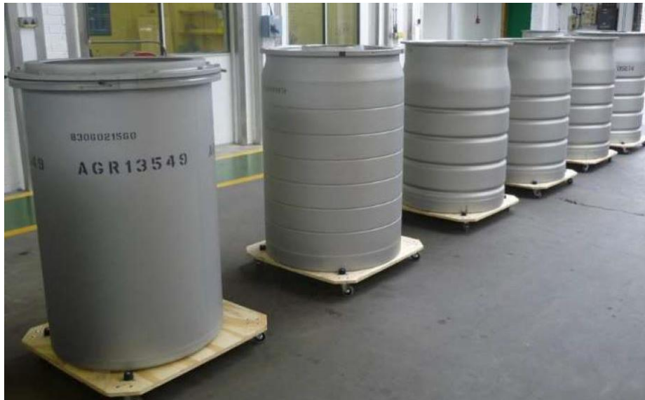
Figure 4: Different designs of ILW 500 L drums[16].
