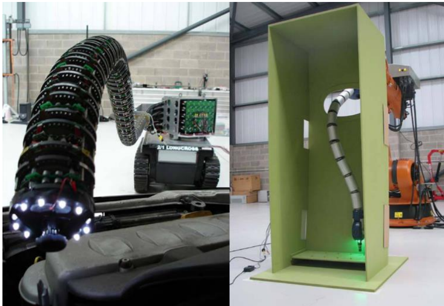
Figure 59: (Left) OCRobotics snake like arm anchored onto a tractor transport system [91]. (Right) OCRobotics robot arm anchored onto a KUKA robot arm, accessing a point of interest through a small gap [91].
