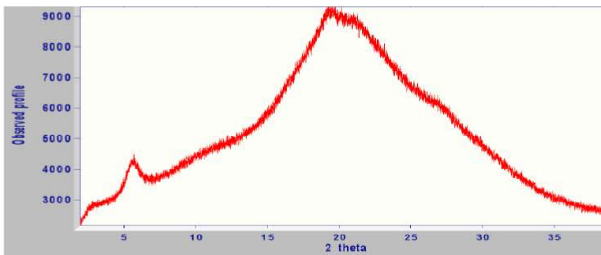
Figure 6.3 amorphous ‘haloes’ observed in laboratory XRPD experiments at 100K Top: amorphous CBZ, Bottom: amorphous IND. The only information immediately obtainable from laboratory XRPD is that the local packing in CBZ is different to that in IND, which is unsurprising. The peak at ca. 6^\circ 2\theta which is present in both the IND and CBZ patterns is due to the Kapton capillary.
