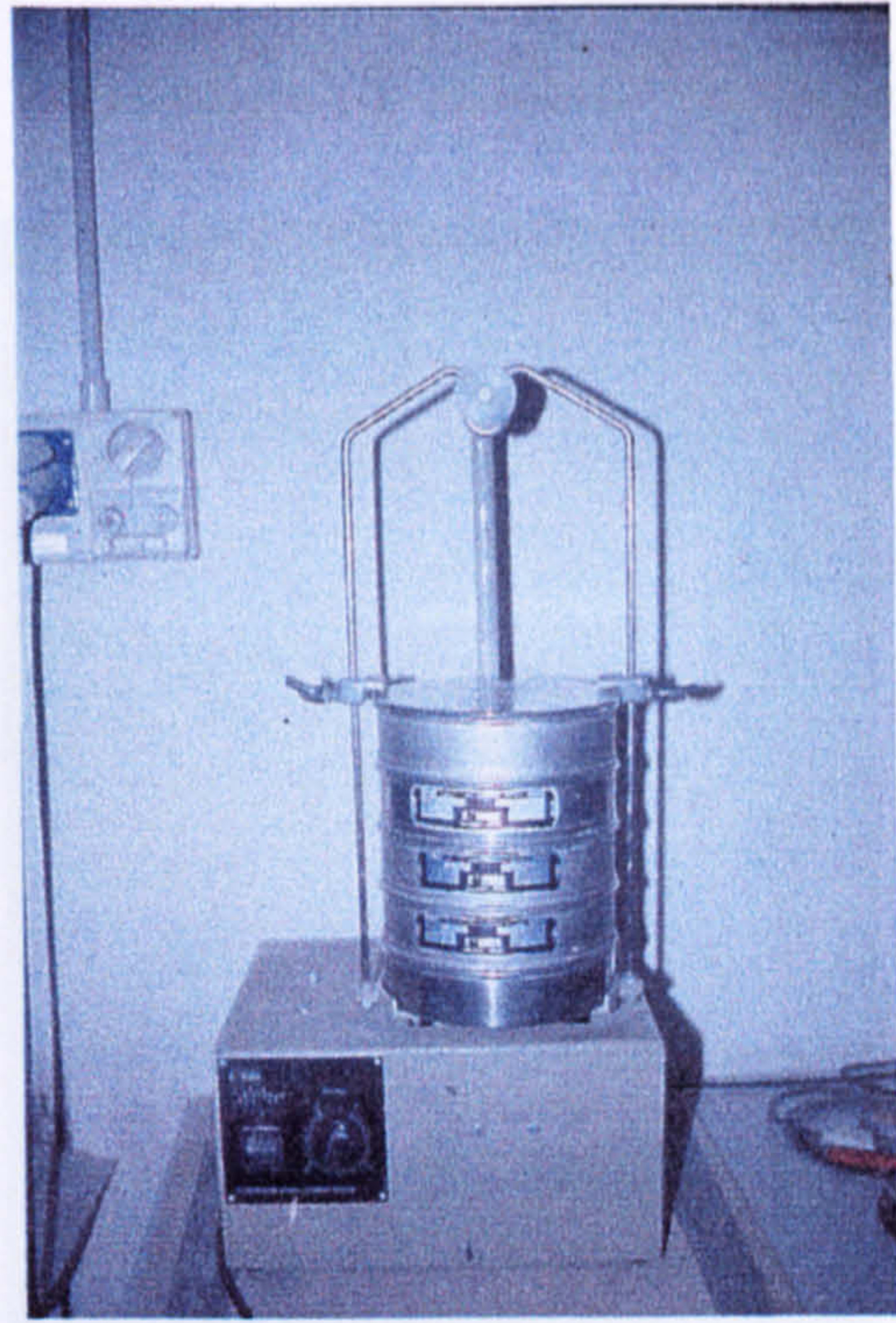
Fig. 3.10 Recycled aggregate stoked in a production plant and a sieve shaker used for the sieve analysis.
