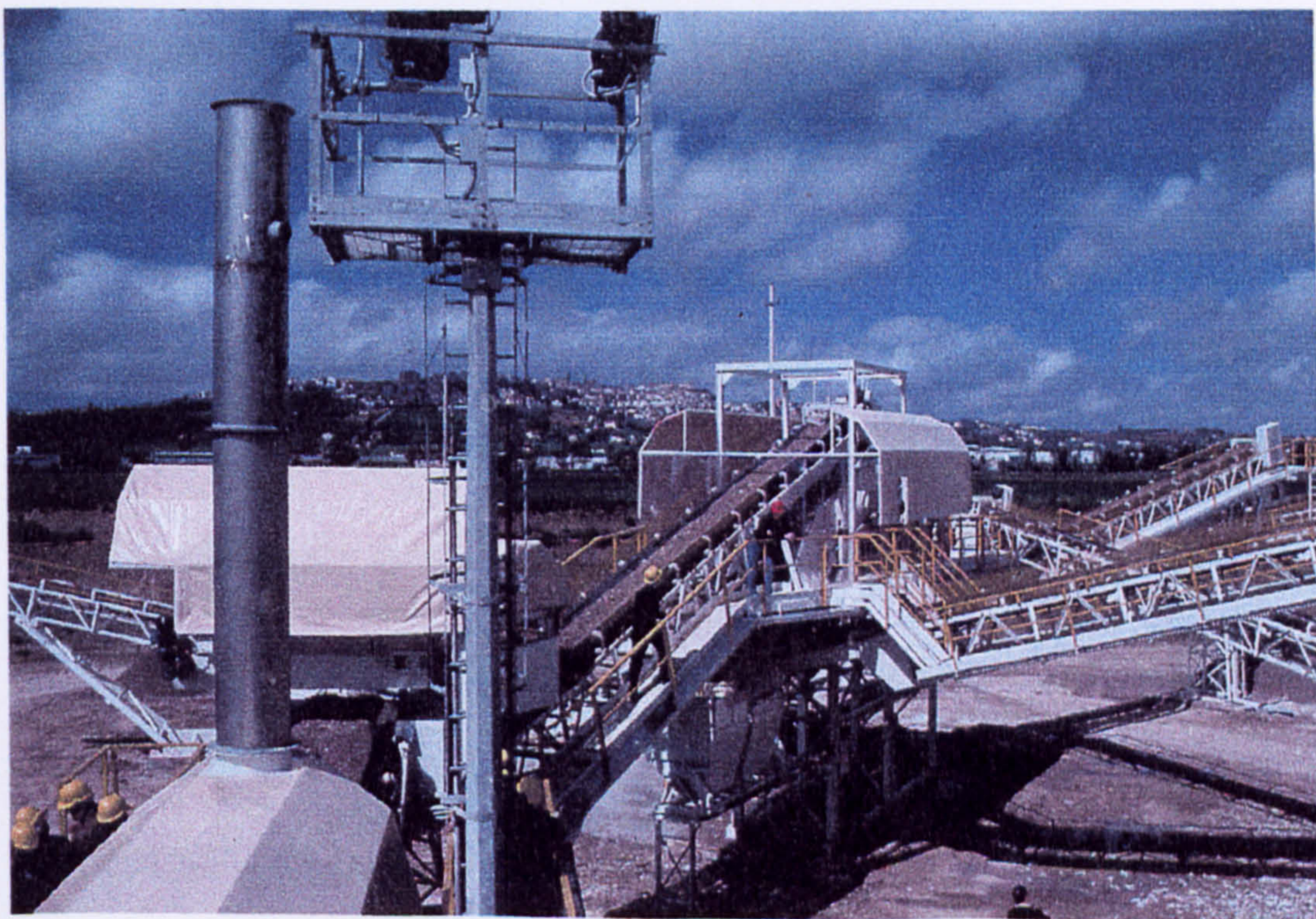
Fig. 3.8 Dust control system.
