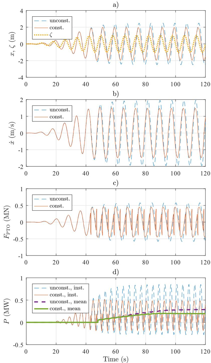
**Figure 6.36:** Response of the device in both constrained and unconstrained conditions in regular waves with  $H = 2$  m and  $T = 8$  s, including plots of the displacement, velocity, PTO force and generated power.
