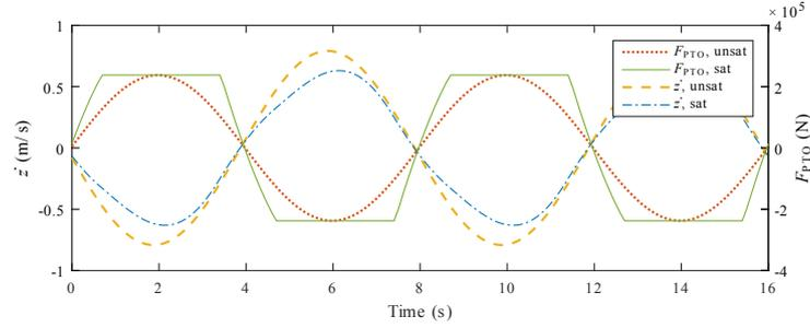
**Figure 6.15:** PTO velocity and force over two wave periods in regular waves with  $H_s = 2$  m and  $T_z = 8$  s for the cases of unsaturated ( $B_{\text{PTO}} = 300$  kNs/m) and saturated ( $B_{\text{PTO}} = 800$  kNs/m) PTO force, when  $F_{\text{Max}} = 237.910$  kN.
