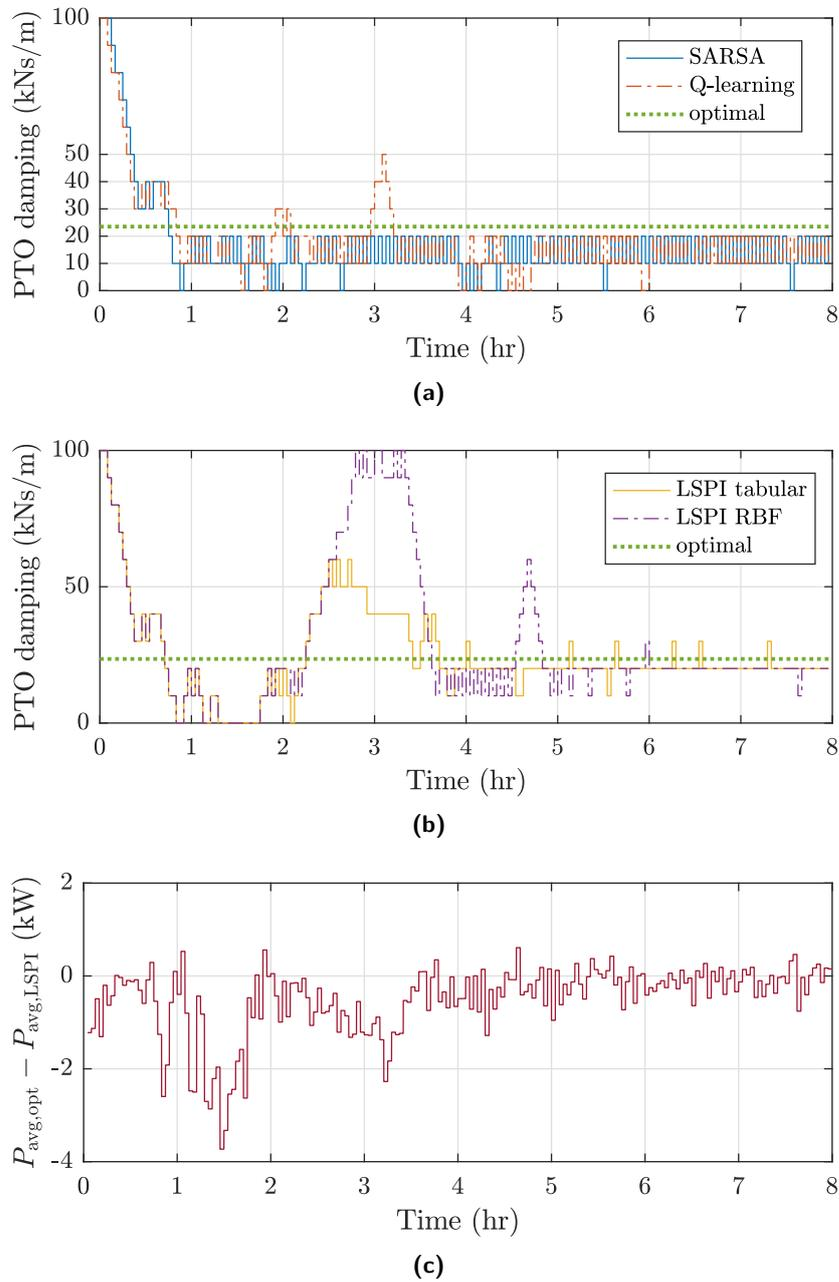
**Figure 6.24:** PTO damping coefficient selected by different reinforcement learning control strategies as compared with the optimal value in irregular waves with  $H_s = 2$  m and  $T_e = 6$  s and a JONSWAP spectrum starting from  $B_{\text{PTO}} = 100$  kNs/m (a-b). (c) shows the difference in the mean generated power for the optimum ( $P_{\text{avg,opt}}$ ) and the case of LSPI with RBFs ( $P_{\text{avg,LSPI}}$ ).
