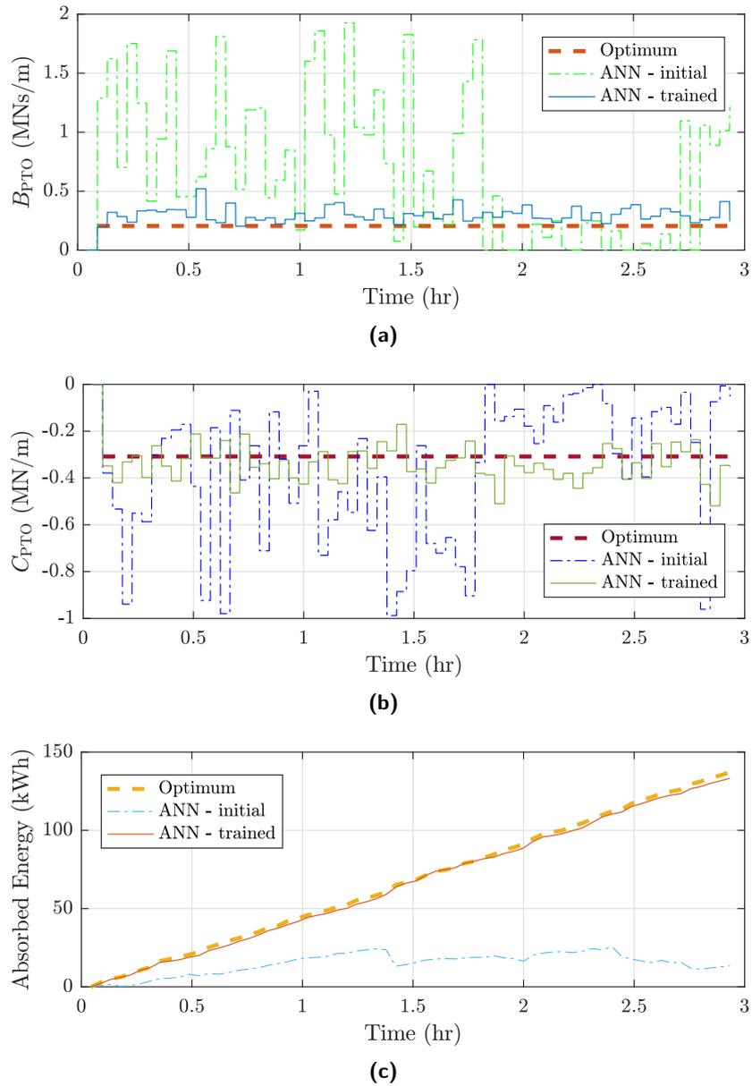
**Figure 5.7:** PTO damping (a) and stiffness (b) coefficients adopted by the ANN-based control at the start and after 54-hours of training in the wave conditions shown in Table 5.1 in irregular waves with  $H_s = 2$  m and  $T_e = 8$  s. Additionally, (a) and (b) display the optimal coefficients computed from a time-domain simulation in a 20-minute-long wave trace. The corresponding curves for the absorbed energy are plotted in (c).
