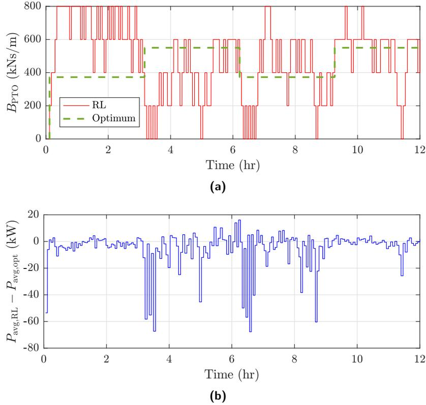
**Figure 6.18:** Optimal and control-selected ( $I = 1$ ,  $K = 4$ ,  $L = 5$ ) PTO damping coefficient (a) and corresponding mean absorbed power (b) in irregular waves with four sea states, generated from the combination of  $H_s = 2, 3$  m and  $T_z = 7, 8$  s.
