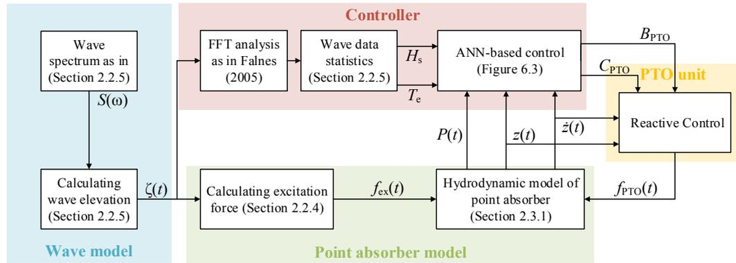
**Figure 5.5:** Flow chart of the program used in the simulations of the point absorber with ANN reactive control.
