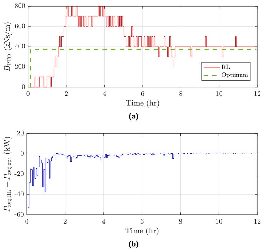
**Figure 6.16:** Optimal and reinforcement-learning-selected PTO damping coefficient (a) and corresponding mean absorbed power (b) in irregular waves with  $H_s = 2$  m and  $T_z = 7$  s, generated using a JONSWAP spectrum.
