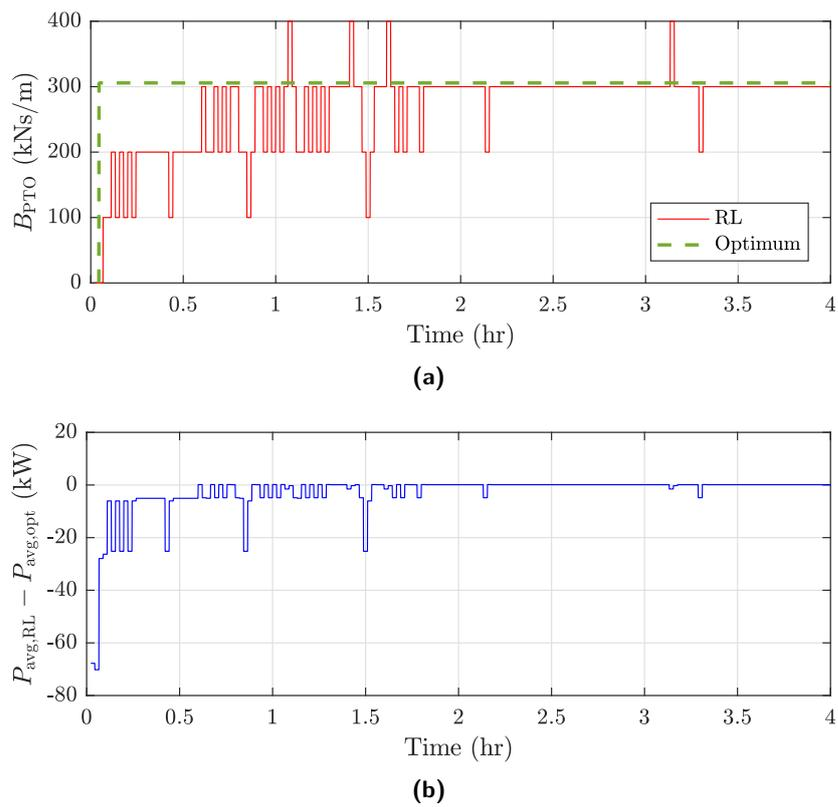
**Figure 6.13:** Optimal and reinforcement-learning-selected PTO damping coefficient (a) and corresponding mean absorbed power (b) in regular waves of unit amplitude and a wave period of 8 s.
