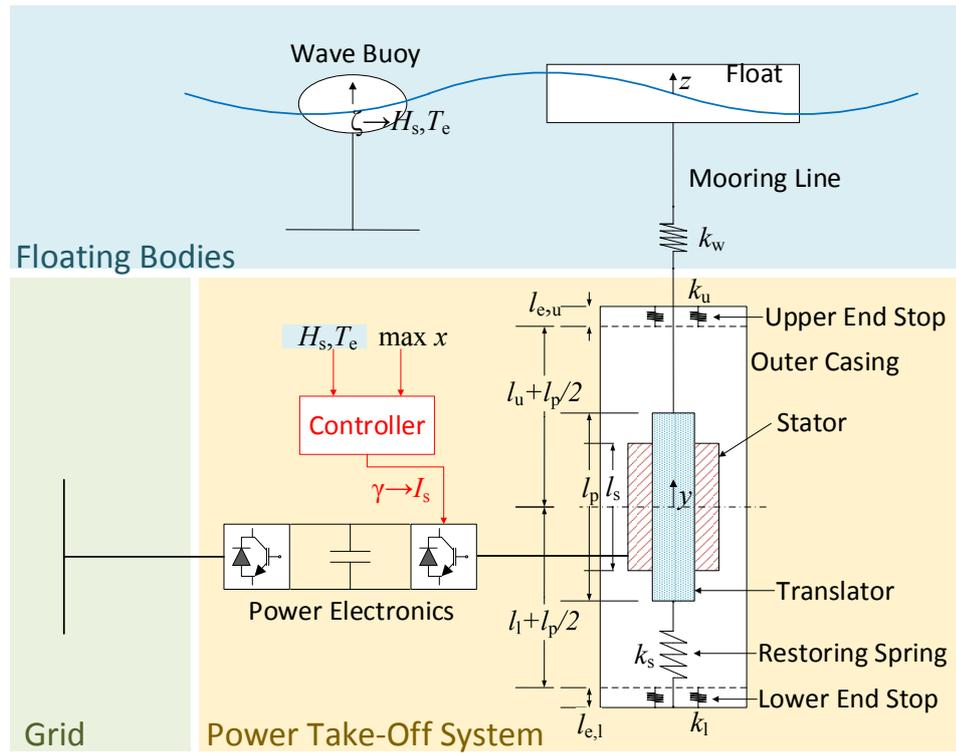
**Figure 2.20:** Diagram of the prototype Seabased WEC.
