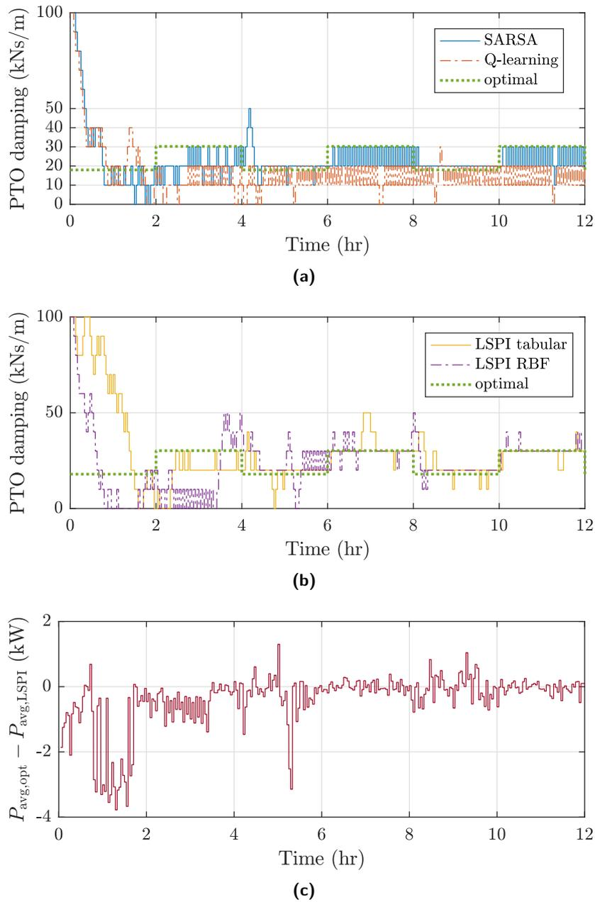
**Figure 6.25:** PTO damping coefficient selected by different reinforcement learning control strategies as compared with the optimal value in irregular waves with two alternating sea states (JONSWAP spectra with  $H_s = 2$  m and  $T_e = 5$  s, and  $H_s = 1$  m and  $T_e = 6$  s) starting from  $B_{\text{PTO}} = 100$  kNs/m (a-b). (c) shows the difference in the mean generated power for the optimum ( $P_{\text{avg,opt}}$ ) and the case of LSPI with RBFs ( $P_{\text{avg,LSPI}}$ ).
