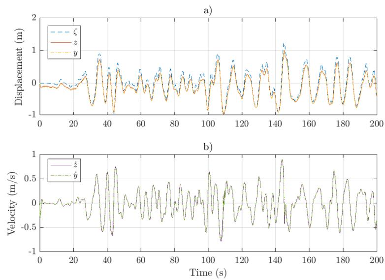
**Figure 2.25:** Wave elevation, heave displacement (a) and velocity (b) of the float ( $z$ ) and translator ( $y$ ) in irregular waves with a Bretschneider spectrum with  $H_s = 2$  m and  $T_p = 9.25$  s (corresponding to  $T_e = 8$  s) with no control force being applied.
