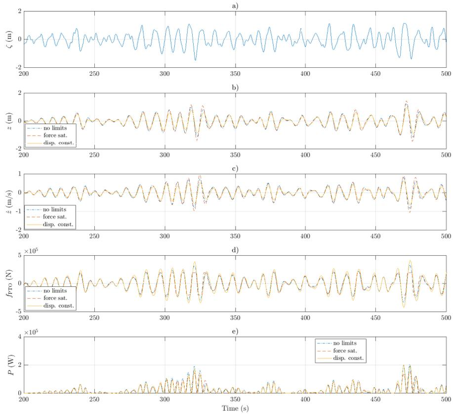
**Figure 3.4:** Wave elevation (a), body vertical displacement (b) and velocity (c), PTO force (d) and corresponding absorbed power (e) when the WEC is passively controlled in irregular waves with a JONSWAP spectrum,  $H_s = 2$  m and  $T_e = 8$  s. The PTO damping coefficient and the force and displacement limits shown in Table 3.1 are used.
