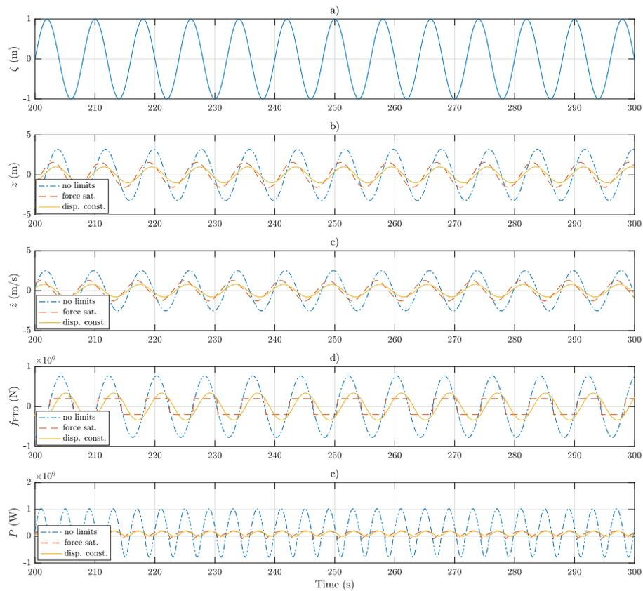
**Figure 3.3:** Wave elevation (a), body vertical displacement (b) and velocity (c), PTO force (d) and corresponding absorbed power (e) when the WEC is actively controlled in regular waves of unit amplitude and a period of 8 s. The PTO damping and stiffness coefficients and the force and displacement limits shown in Table 3.1 are used.
