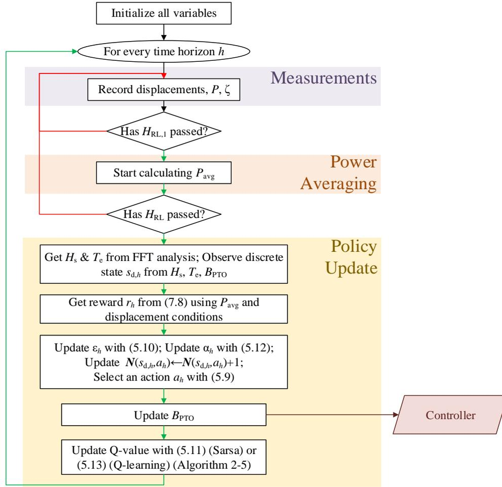
**Figure 6.10:** Flowchart of the Q-learning or Sarsa algorithm for the resistive control of the point absorber.
