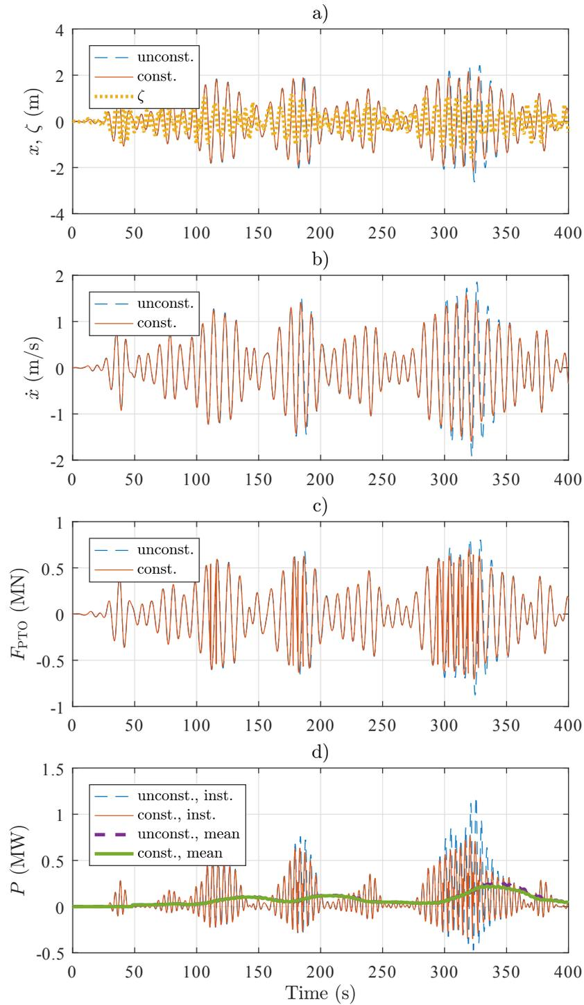
**Figure 6.37:** Response of the device in both constrained and unconstrained conditions in irregular waves with  $H_s = 2$  m and  $T_e = 8$  s, including plots of the displacement, velocity, PTO force and generated power.
