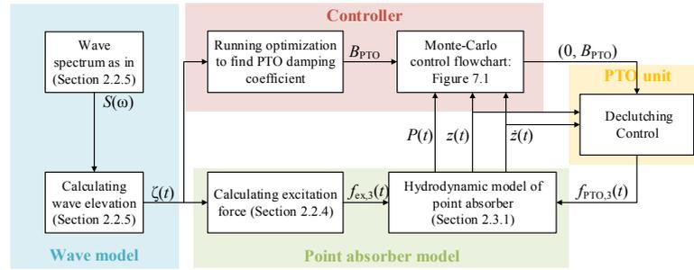
**Figure 6.3:** Work-flow diagram of the program used to simulate the point absorber.
