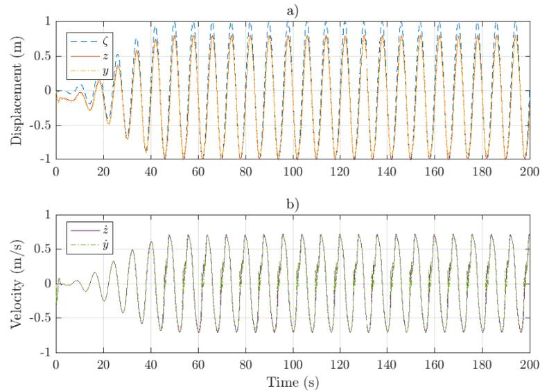
**Figure 2.24:** Wave elevation, heave displacement (a) and velocity (b) of the float ( $z$ ) and translator ( $y$ ) in regular waves of unit amplitude and a period of 8 s with no control force being applied.
