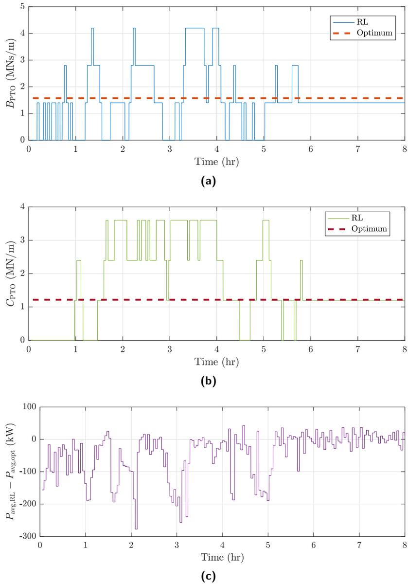
**Figure 6.32:** Time variation of the PTO damping (a) and stiffness (b) coefficients chosen by the reinforcement learning control as compared with the respective optimal values in irregular waves with  $H_s = 2$  m and  $T_e = 8$  s. (c) shows the difference between the corresponding mean generated power and the optimal mean generated power.
