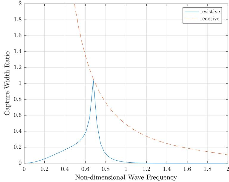
**Figure 3.1:** Variation in the capture width ratio of the analysed point absorber with non-dimensional wave frequency. The curves for both resistive and reactive control are applied.
