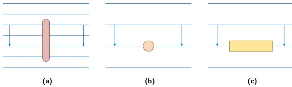
**Figure 2.2:** Three main categories of wave energy technologies: attenuator (a), point absorber (b) and terminator (c) in planar waves. Waves radiated by the WEC are not shown in this diagram for simplicity.
