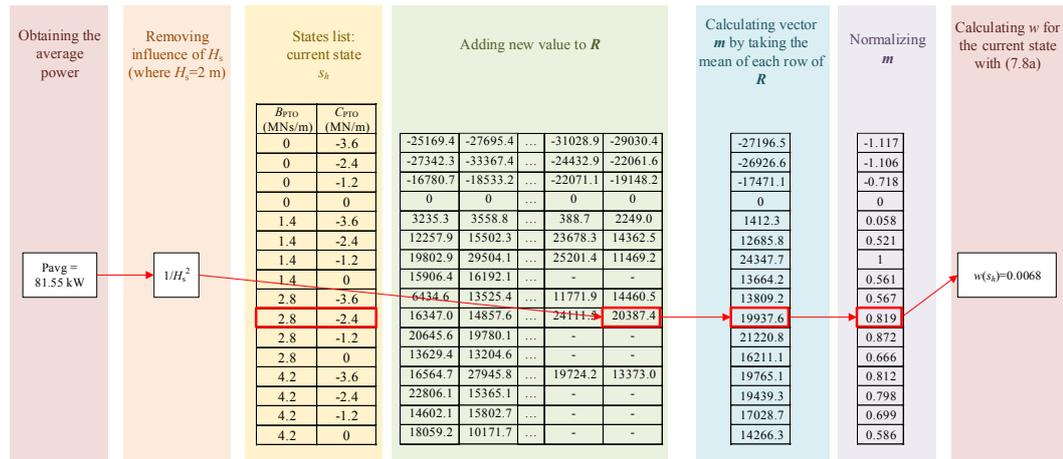
**Figure 6.27:** Calculating the reward  $w$  (excluding penalties for large motions) at one step of the reinforcement learning algorithm in irregular waves. This corresponds to the last step in Figure 6.32 in Section 6.3.7.2.
