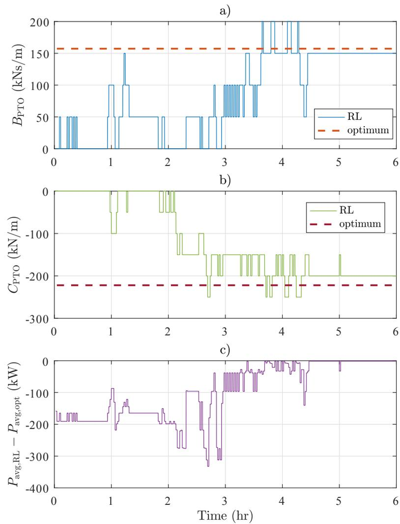
**Figure 6.33:** Selection of the PTO damping (a) and stiffness (b) coefficients by the reinforcement learning control as compared with the respective optimal values in regular waves with  $H = 2$  m and  $T = 8$  s and a maximum allowable displacement of 5 m. The difference in the corresponding mean generated power can be seen in (c).
