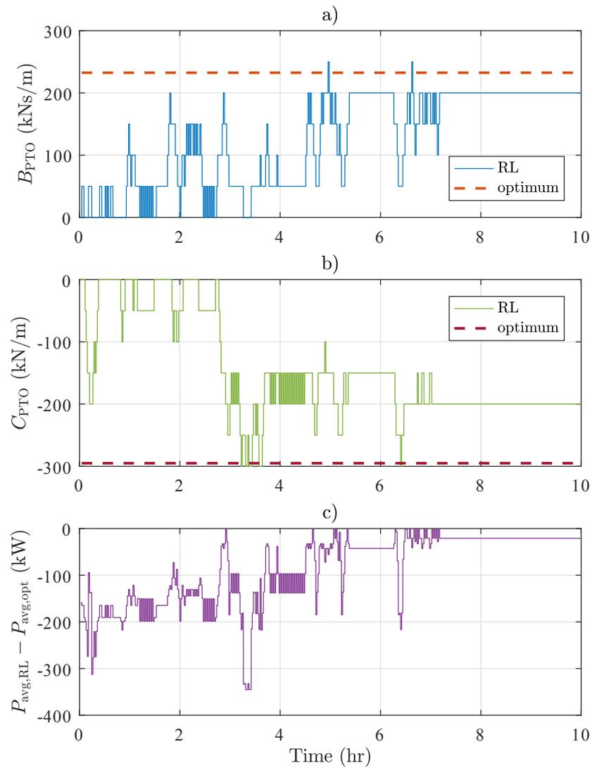
**Figure 6.35:** Time variation of the PTO damping (a) and stiffness (b) coefficients chosen by the reinforcement learning control as compared with the respective optimal values in regular waves with  $H = 2$  m and  $T = 8$  s and a maximum allowable displacement of 2 m. (c) shows the difference between the corresponding and the optimal mean generated power.
