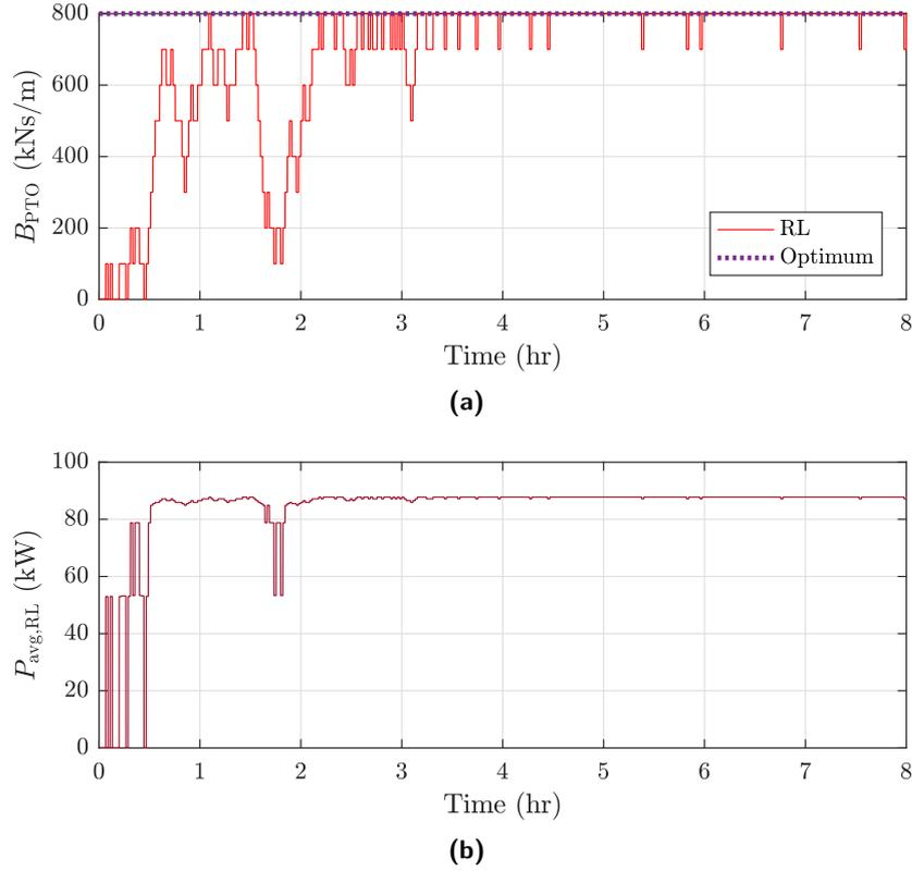
**Figure 6.14:** PTO damping coefficient selected by the Q-learning algorithm (a) and corresponding mean generated power (b) in regular waves with  $H_s = 2.2$  m and  $T_z = 8$  s, when  $F_{Max} = 237.910$  kN.
