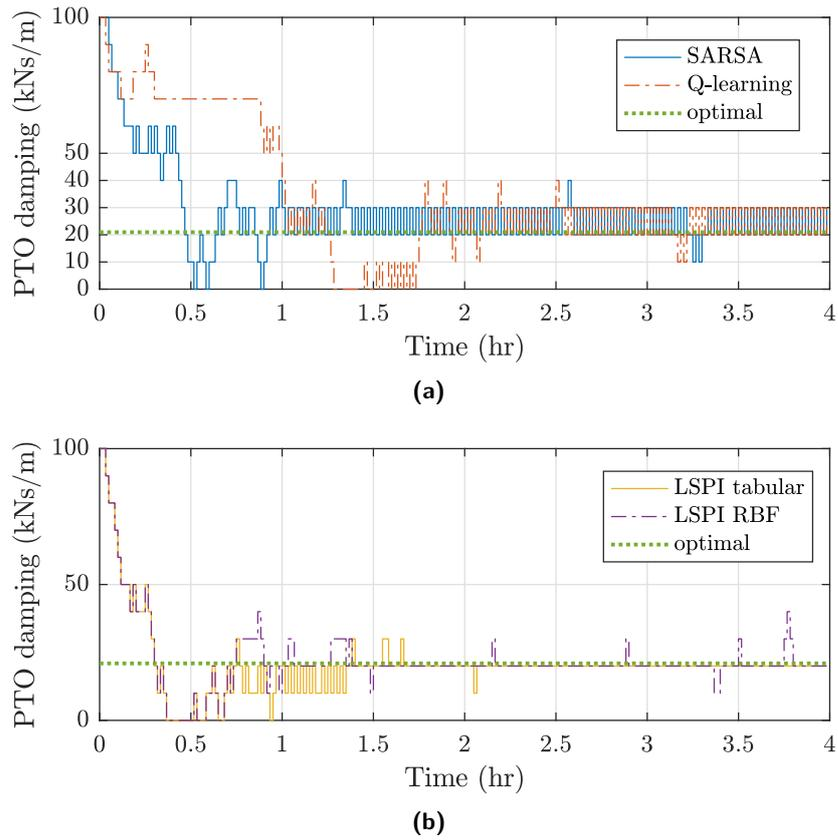
**Figure 6.21:** PTO damping coefficient selected by different reinforcement learning control strategies as compared with the optimal value in regular waves with unit amplitude and  $T = 6$  s starting from  $B_{\text{PTO}} = 100$  kNs/m.
