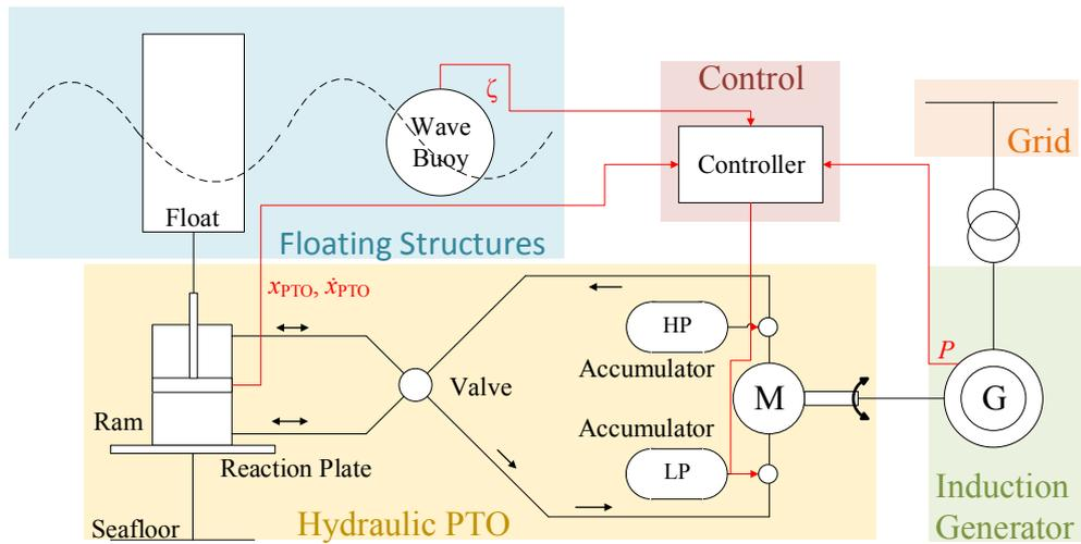
Figure 2.13: Diagram of the two-body point absorber with a hydraulic PTO system.
