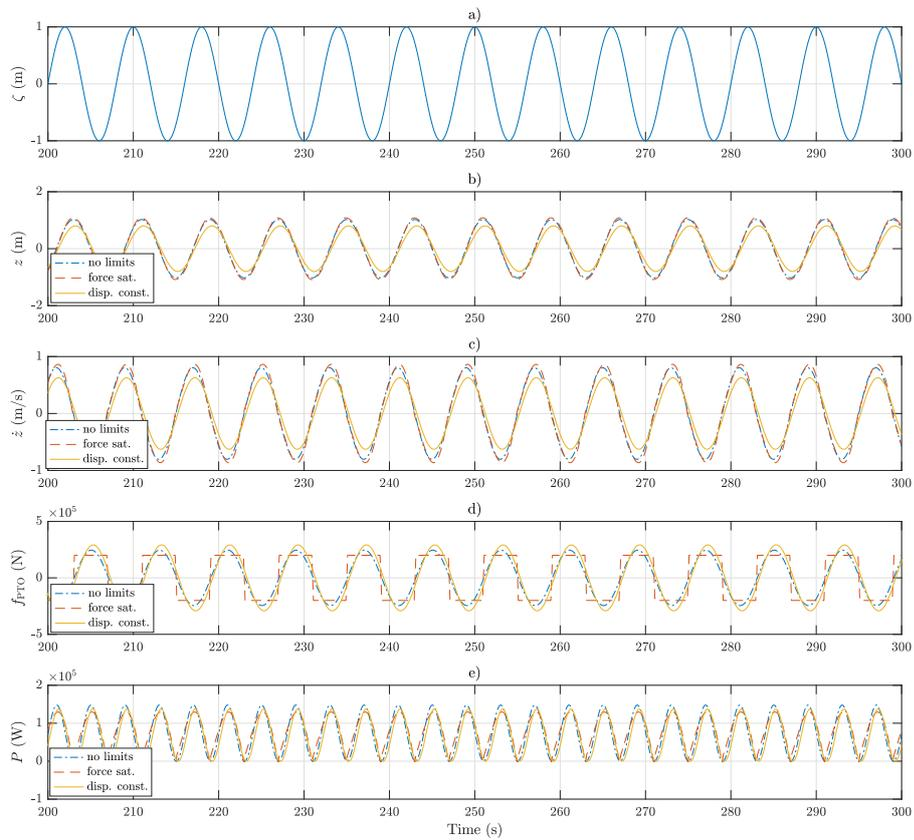
**Figure 3.2:** Wave elevation (a), body vertical displacement (b) and velocity (c), PTO force (d) and corresponding absorbed power (e) when the WEC is passively controlled in regular waves of unit amplitude and a period of 8 s. The PTO damping coefficient and the force and displacement limits shown in Table 3.1 are used.
