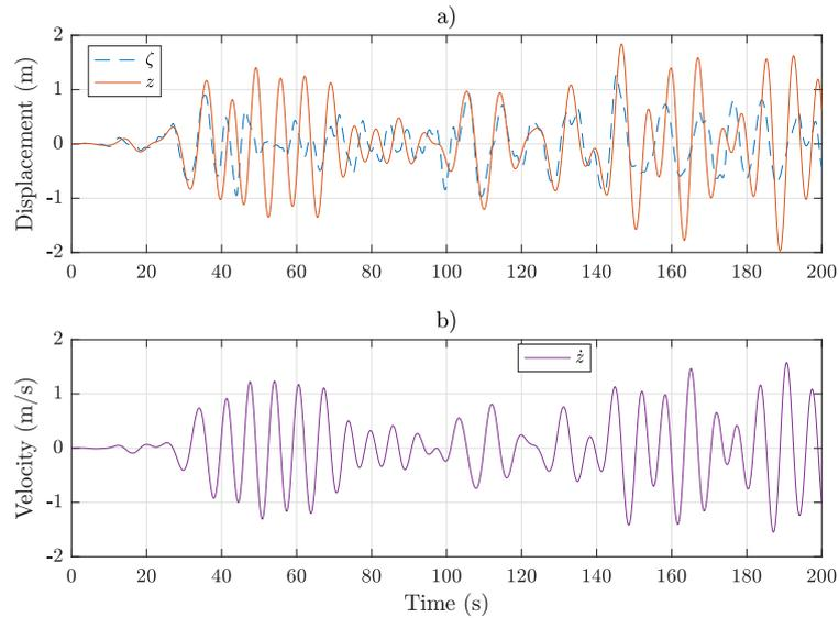
**Figure 2.12:** Wave elevation, float displacement (a) and velocity (b) in irregular waves with a Bretschneider spectrum with  $H_s = 2$  m and  $T_p = 9.25$  s (corresponding to  $T_e = 8$  s) with no control force being applied.
