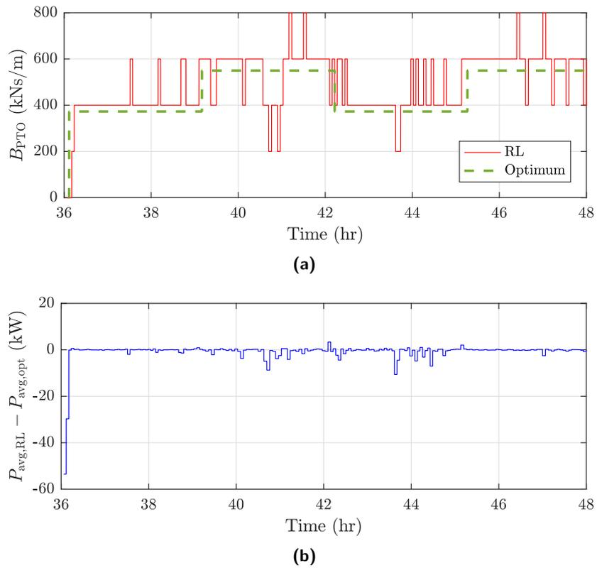
**Figure 6.19:** Optimal and control-selected ( $I = 1$ ,  $K = 4$ ,  $L = 5$ ) PTO damping coefficient (a) and corresponding mean absorbed power (b) in irregular waves with four sea states, generated from the combination of  $H_s = 2, 3$  m and  $T_z = 7, 8$  s (Continuation of Figure 6.18).
