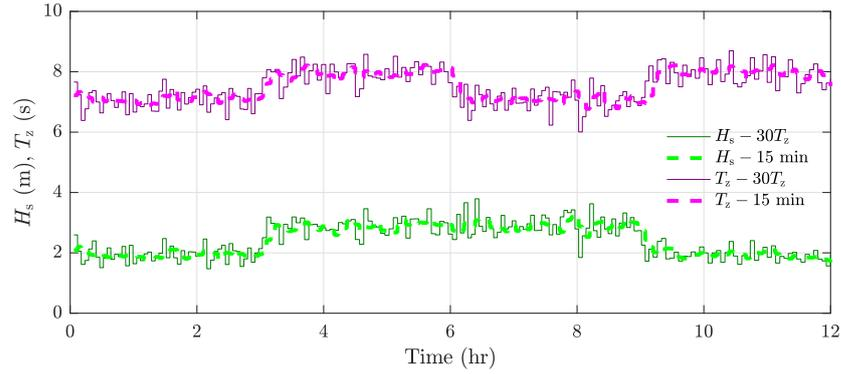
**Figure 6.17:** Significant wave height and mean zero-crossing period calculated over each horizon (continuous lines) and over overlapping 15-minute windows every minute (dotted lines) for the multiple sea state wave trace.
