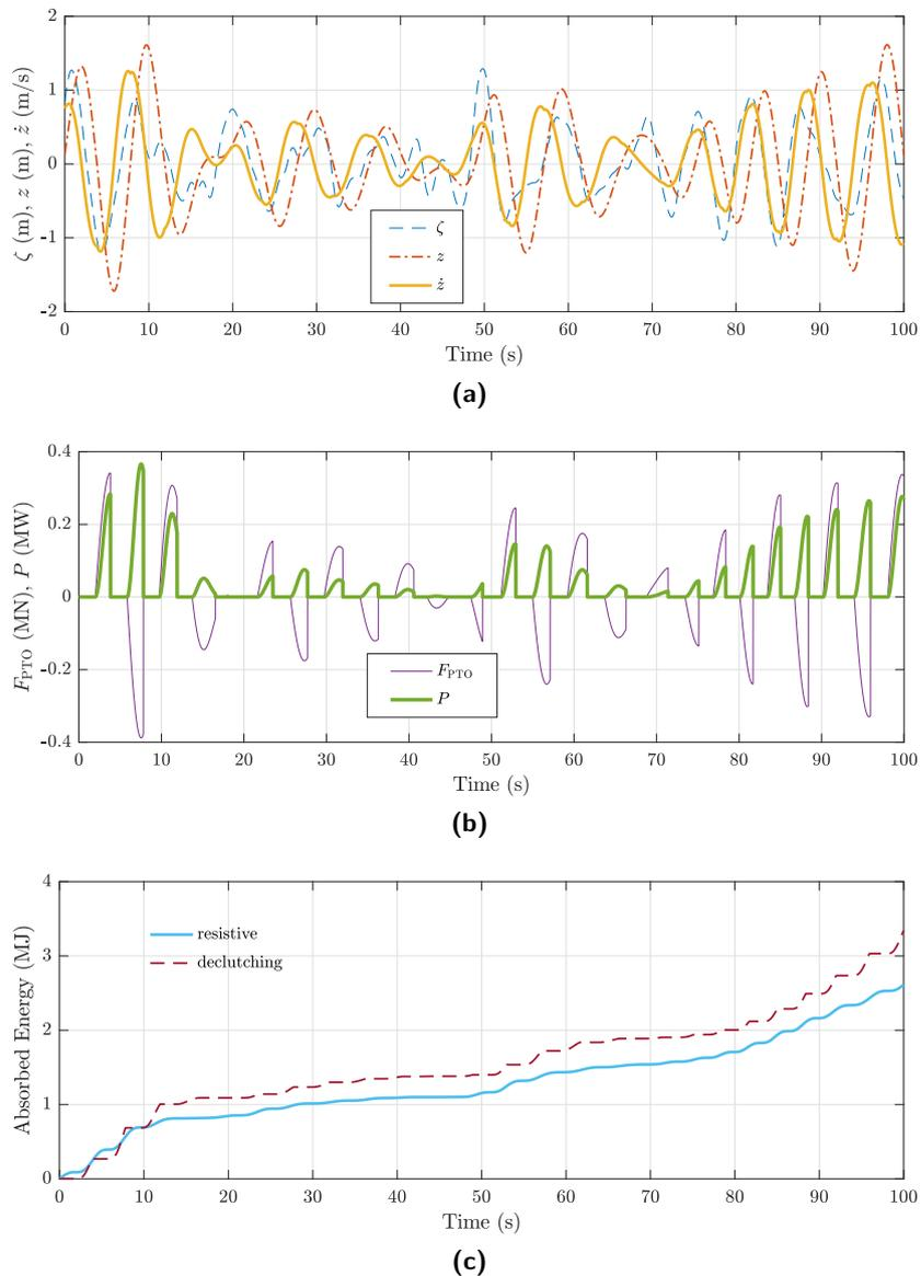
**Figure 6.8:** Time series of the (a) wave elevation  $\zeta$ , body vertical displacement  $z$  and velocity  $\dot{z}$ , (b) PTO force  $F_{PTO}$  and generated power  $P$  in irregular waves once the optimal policy has been found. Additionally, (c) shows the corresponding absorbed energy as compared with resistive control.
