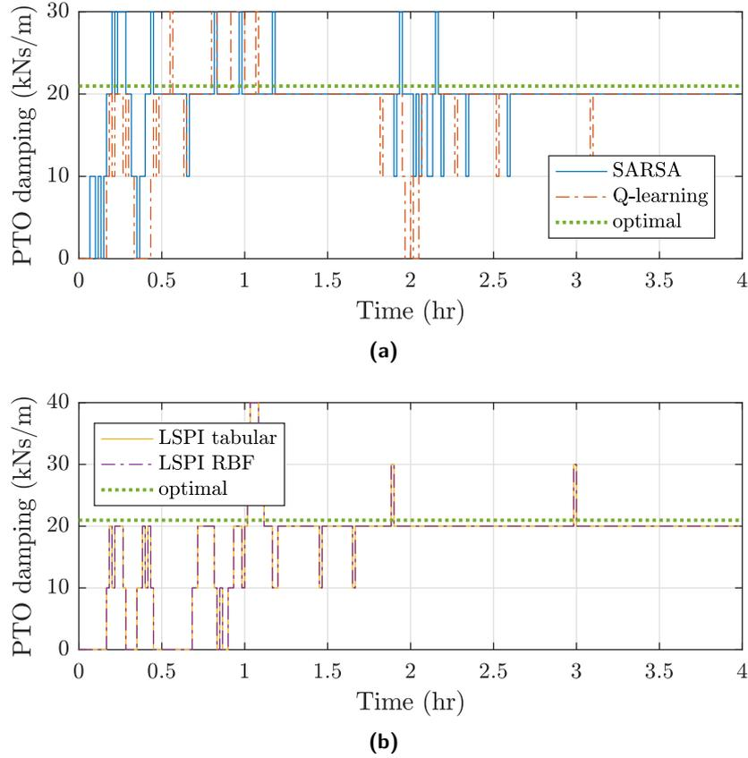
**Figure 6.20:** PTO damping coefficient selected by different reinforcement learning control strategies as compared with the optimal value in regular waves with unit amplitude and  $T = 6$  s starting from  $B_{PTO} = 0$  kNs/m.
