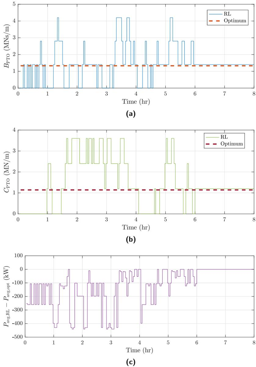
**Figure 6.31:** Time variation of the PTO damping (a) and stiffness (b) coefficients chosen by the Q-learning control as compared with the respective optimal values in regular waves of unit amplitude and a wave period of 8 s. (c) shows the difference between the corresponding mean generated power and the optimal mean generated power.
