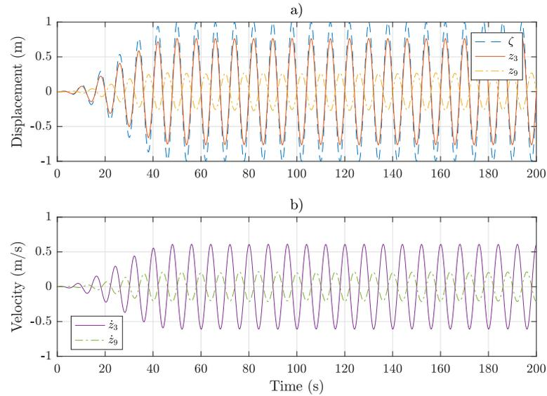
**Figure 2.18:** Wave elevation, heave displacement (a) and velocity (b) of the float (3) and reaction plate (9) in regular waves of unit amplitude and a period of 8 s with no control force being applied.
