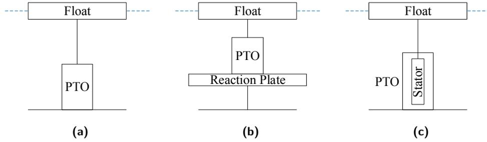
**Figure 2.6:** Diagram of the point absorbers simulated in this thesis.
