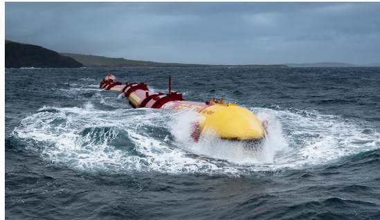
**Figure 2.1:** Pelamis P2 WEC in Orkney (with permission from Pelamis Wave Power Ltd.).
