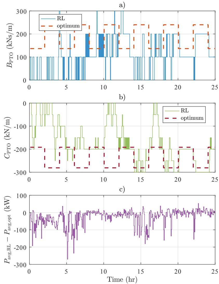
**Figure 6.34:** Time variation of the PTO damping (a) and stiffness (b) coefficients chosen by the reinforcement learning control as compared with the respective optimal values in irregular waves with two, alternating sea states. (c) shows the difference between the corresponding and the optimal mean generated power.
