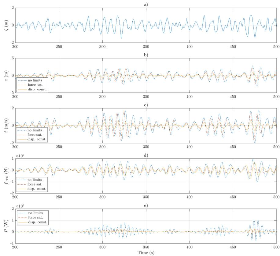
**Figure 3.5:** Wave elevation (a), body vertical displacement (b) and velocity (c), PTO force (d) and corresponding absorbed power (e) when the WEC is actively controlled in irregular waves with a JONSWAP spectrum,  $H_s = 2$  m and  $T_e = 8$  s. The PTO damping and stiffness coefficients and the force and displacement limits shown in Table 3.1 are used.
