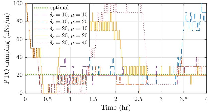
**Figure 6.22:** PTO damping coefficient selected by the LSPI algorithm with different RBF settings in regular waves with unit amplitude and  $T = 6$  s. The values of  $\delta_c$  and  $\mu$  are in kNs/m.
