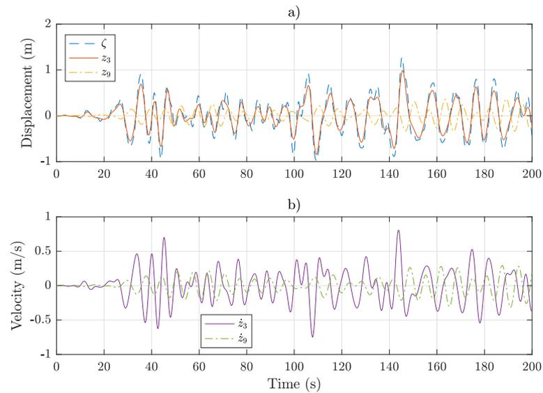
**Figure 2.19:** Wave elevation, heave displacement (a) and velocity (b) of the float (3) and reaction plate (9) in irregular waves with a Bretschneider spectrum with  $H_s = 2$  m and  $T_p = 9.25$  s (corresponding to  $T_e = 8$  s) with no control force being applied.
