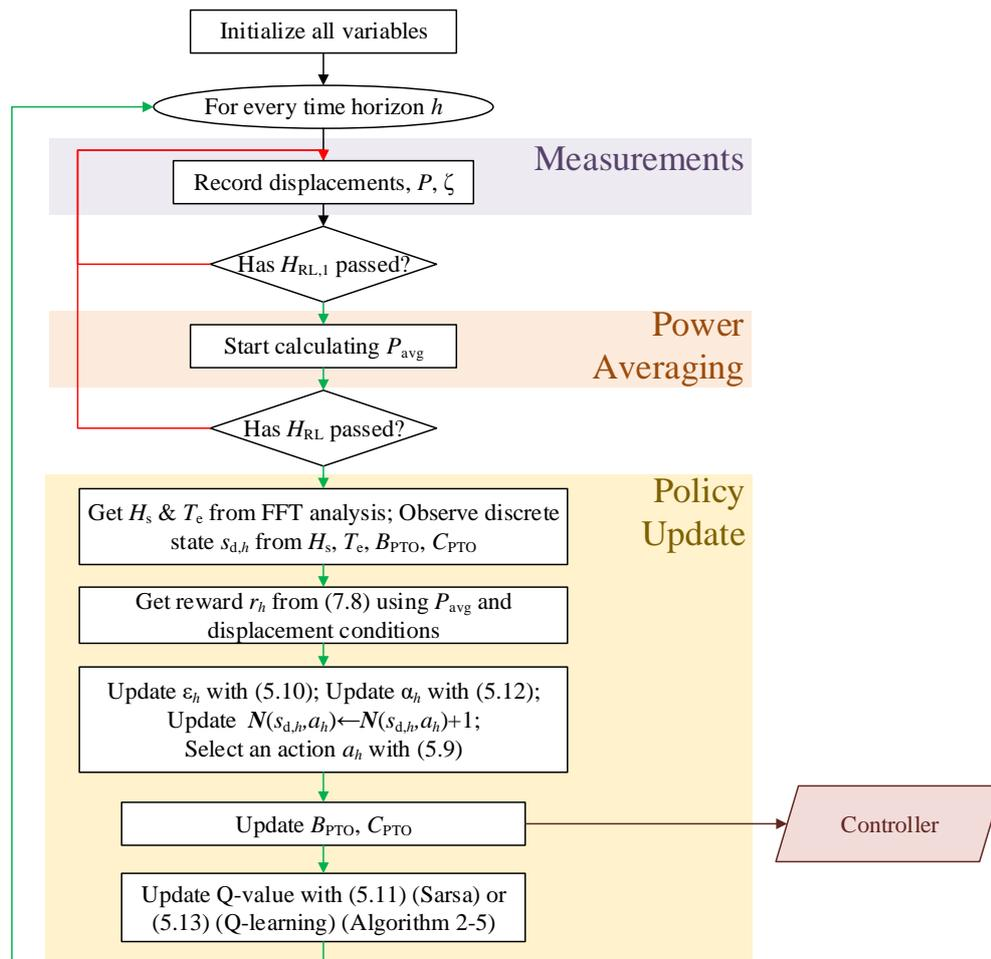
**Figure 6.28:** Flowchart of the Q-learning or Sarsa algorithm for the reactive control of a WEC.
