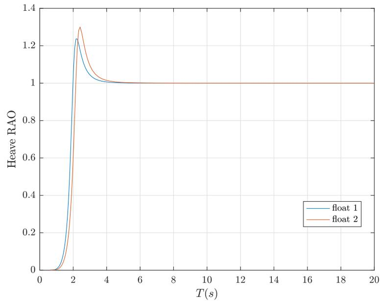
**Figure 2.22:** Magnitude of the response amplitude operator against wave period for the two floating vertical cylinders with a radius of 1.5 m and a draught of 0.4 m (original) and 1.75 m and 0.5 m (modified), respectively.
