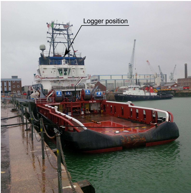
(a) View on logger position over aft deck of tug from quay
