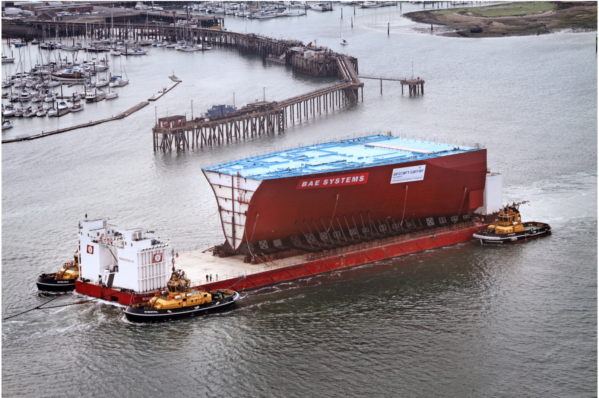
Figure 6.2.1: Lower block 02 @ ~6,500 Te on semisubmersible barge
