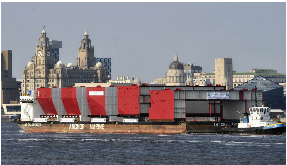
Figure 6.2.2: Forward flight deck sections, 5 off @ ~850 Te each
