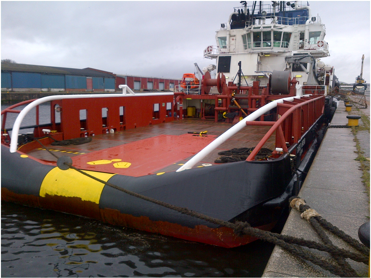
Figure 5.1.1: Typical aft deck of towing tug showing main and secondary towing winches
