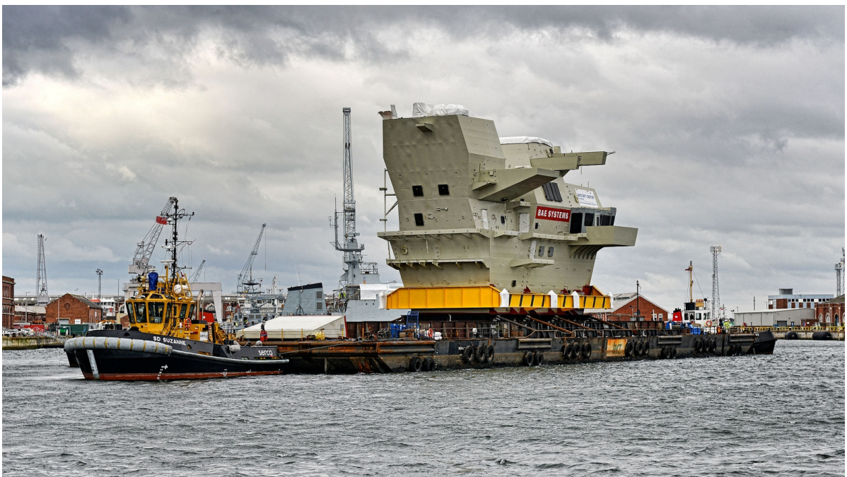
Figure 6.2.4: Bridge section @ ~850 Te
