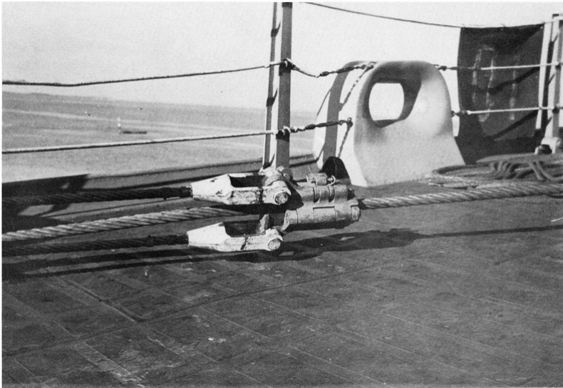
Figure 3.3.1: Example use of a “Carpenter Stopper” in a salvage operation (image credit www.maritime.org )
