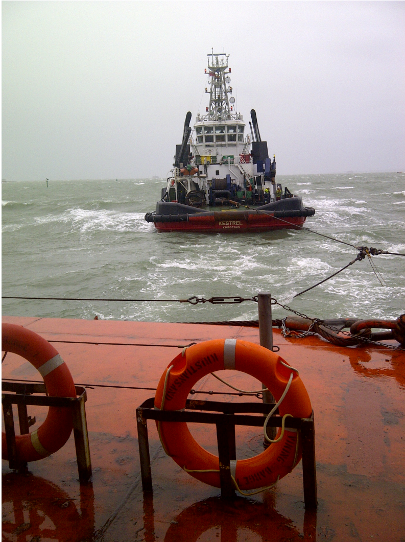
Figure 5.1.3: View on Towing Tug and Bridle at Sea
