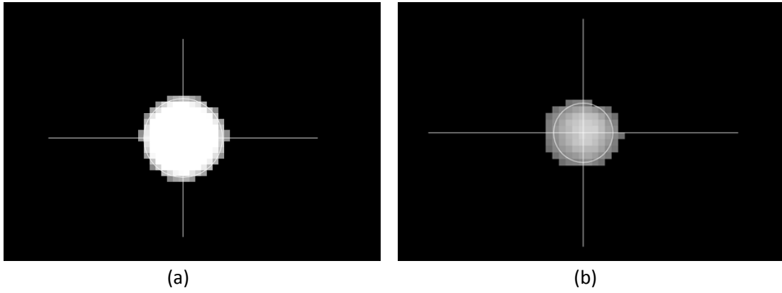
Figure 3.11: (a) Aperture fully open showing high intensity white pixels representing a marker (b) Aperture semi open resulting in low intensity pixels for a marker
