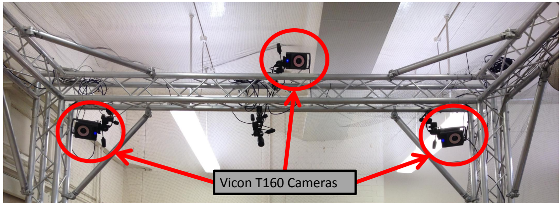
Figure 3.8: Camera arrangement on the right hand side of the frame in Figure 3.3. This arrangement was found to maximise coverage within the measurement volume.
