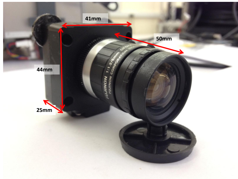
Figure 4.2: Point Grey Research Chameleon. Sony ICX445 1/3" CCD based camera of dimension 25.5 mm x 41 mm x 44 mm
