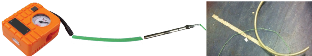
Figure 3:20 – Experimental setup with controllable changes to pressure over time: (a) the pump was connected to one end of a hose while the sensor inserted at the other; gaps were sealed, (b) a picture of the sensor inserted into the tube with the far end of the tube sealed on the floor of the engine room.
