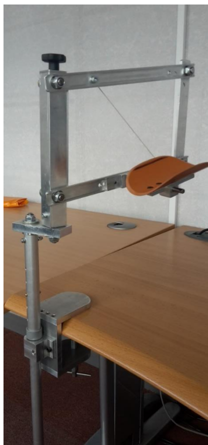
Figure 3.9 - Working prototype of the weight support device.
