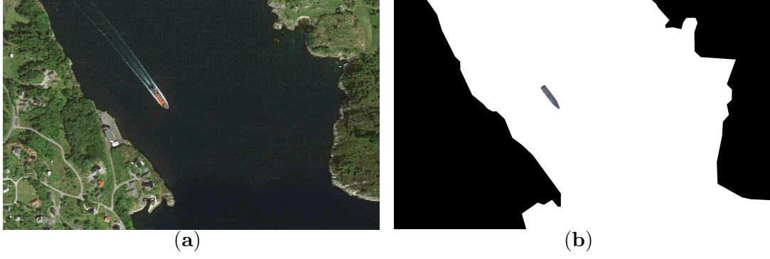
Figure 4.5 (a) Satellite image of a navigational area captured using Google Maps. (b) 2D occupancy grid map of the navigational area.
