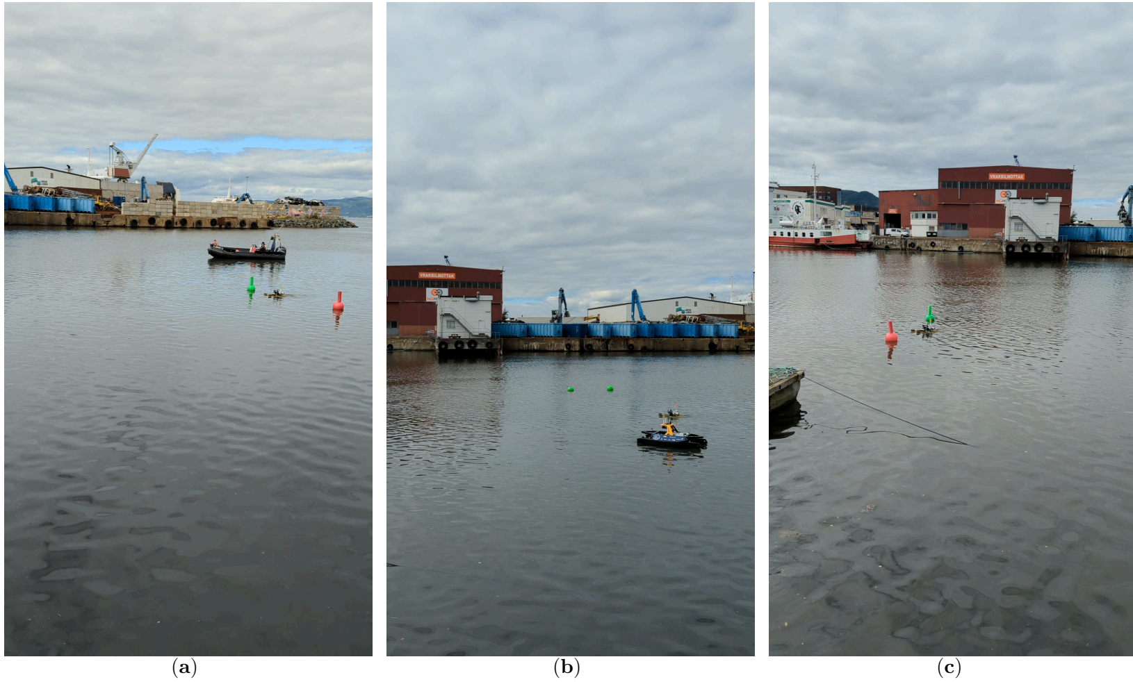
Figure 6.47 Timesteps of the experimental validation during (a) the initial position prior to detecting the obstacle, (b) the COLREG-compliant evasive manoeuvre, and (c) arrival to the final destination after path recovery.
