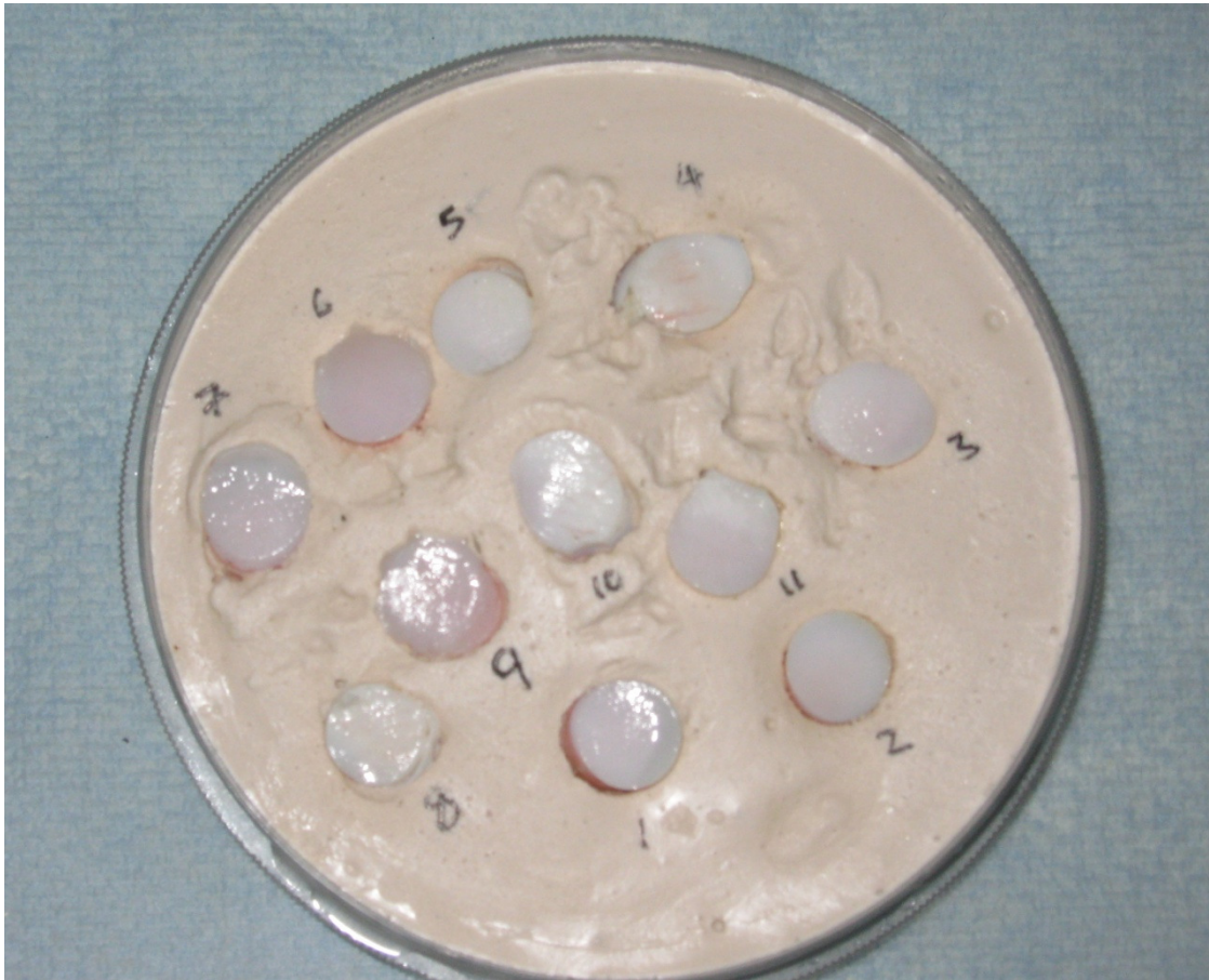
Figure 6.2: The osteochondral plugs are placed in plaster contained petri dish for measuring the creep properties of the cartilage.
