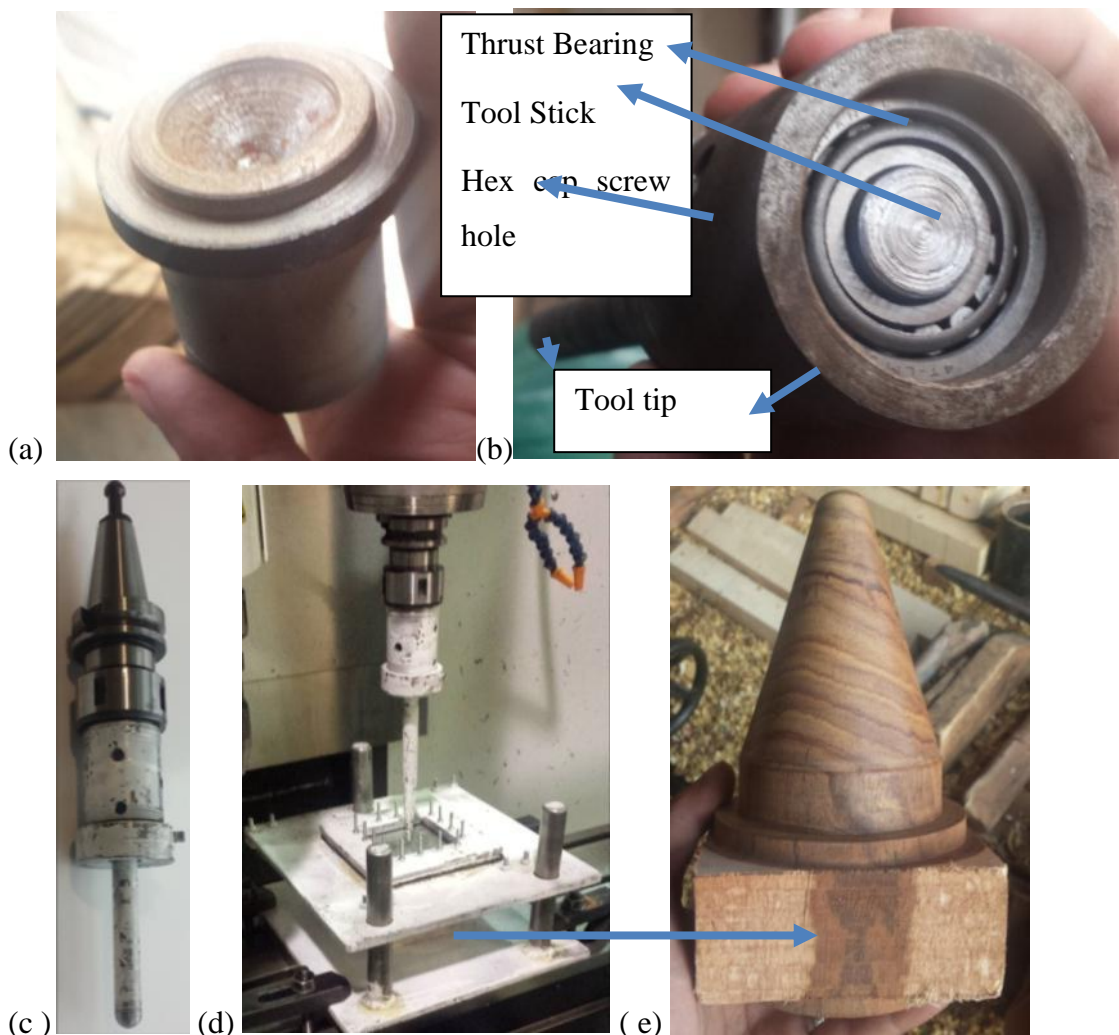
Figure 10-3 Manufacturing and commissioning of tool; (a) Block, (b) Thrust bearings in the tool, (c) Hemispherical tool, (d) Tool while performing ISf process, (e) Wooden die.
