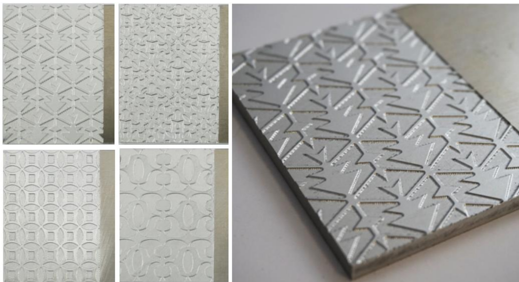
Figure 58: Machined aluminium plates for 'fear', 'surprise', 'trust' and 'joy' designs with perspective view of 'fear' plate
