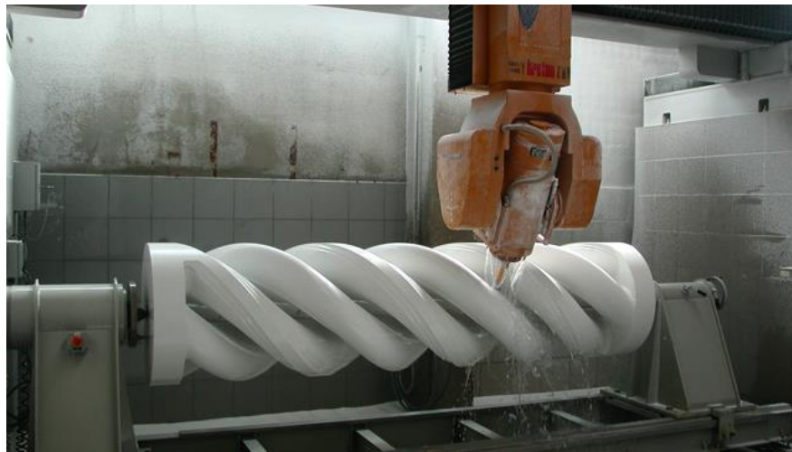
Figure 50 – Breton ShapeMill machining a stone column 18
