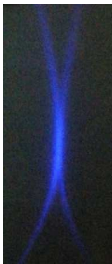
FIGURE 3.13: Photograph of the emission from a T3 DFB laser. Coherent laser emission is observed in the central section of the fan shaped beam with diffracted amplified spontaneous emission accounting for the four extended beams extending from the central region.
