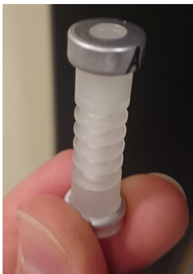
FIGURE 5.2: DNA is purchased in cartridges. A syringe can be inserted into the top (and bottom) of the cartridge to allow for functionalisation of the oligo within the cartridge.
