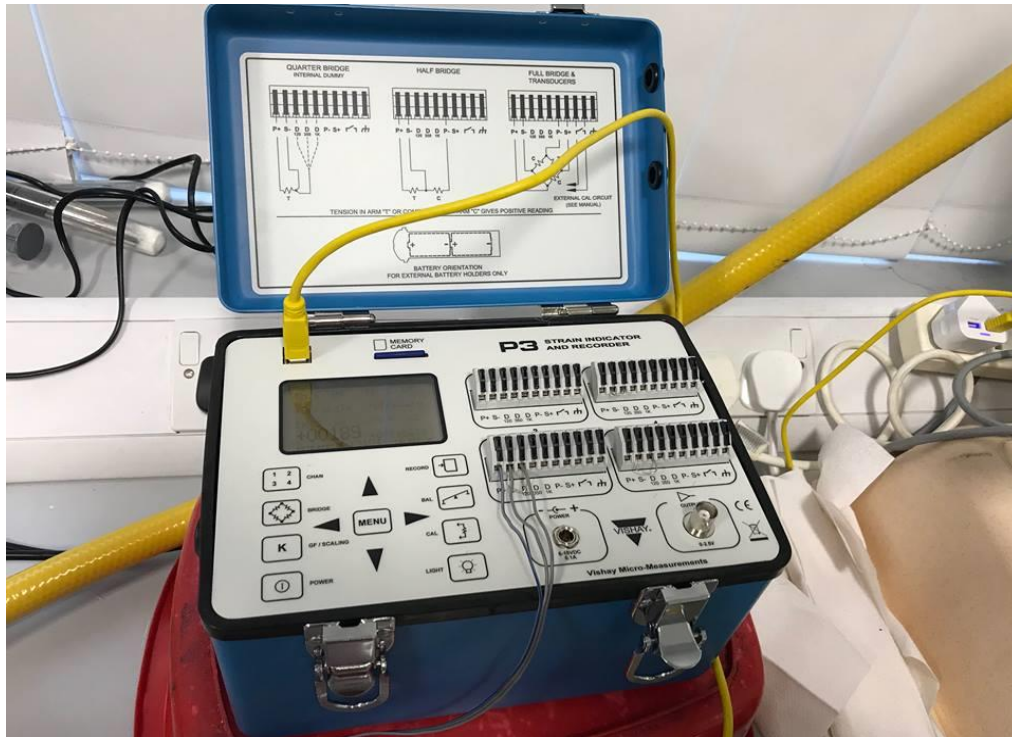
Figure 5.41. Model P3 strain gauge indicator and recorder with the 3 strain gauge lead wires connected in a quarter bridge configuration.
