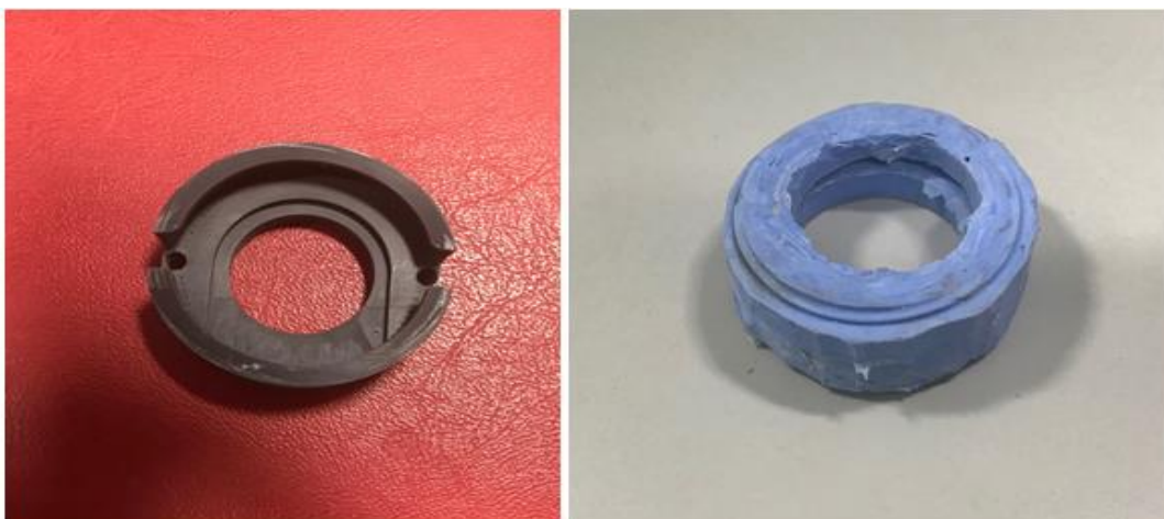
Figure 5.31. Left: 3D printed polymeric valve holder. Right: Clay mould
