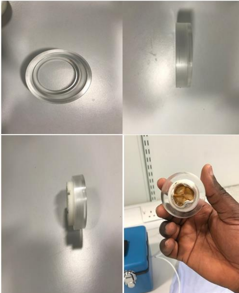
Figure 5.30. The valve holder for the bioprosthetic valve. Top left: Top view of bioprosthetic valve holder. Top right: Side view of the valve holder. Bottom left: Side view of the valve holder with threaded plastic male insert. Bottom right: Bioprosthetic valve inserted in the valve holder.
