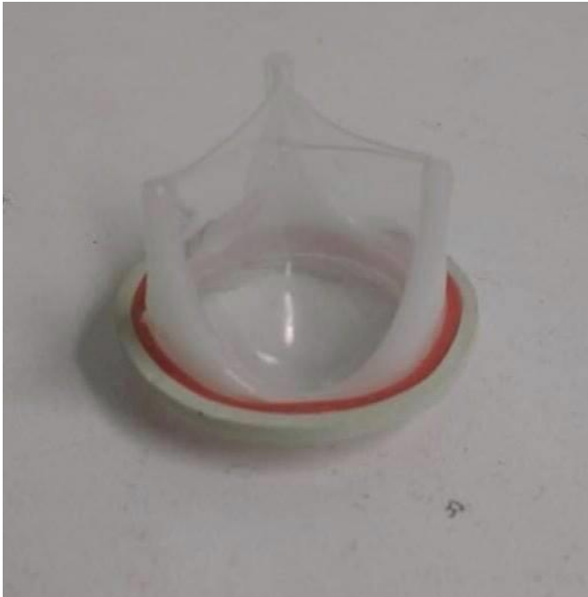
Figure 5.3. 22mm polymeric heart valve fabricated via dip coating.
