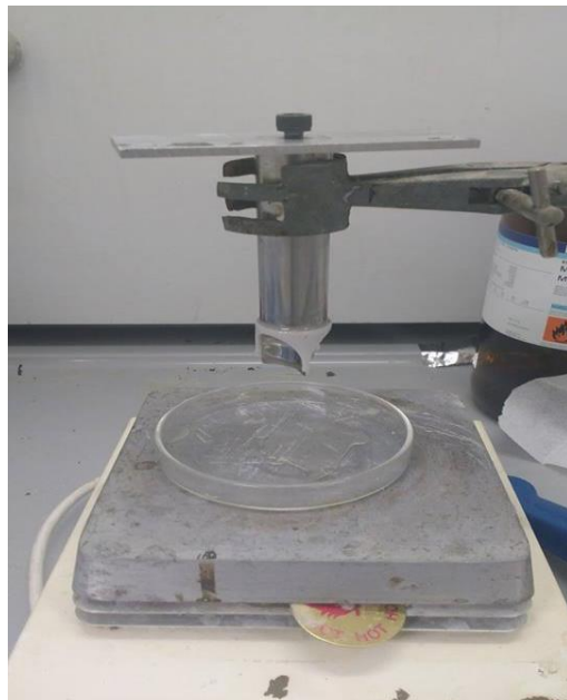
Figure 5.2. The dip coating process. Dip coated mandrel suspended upside down to dry.
