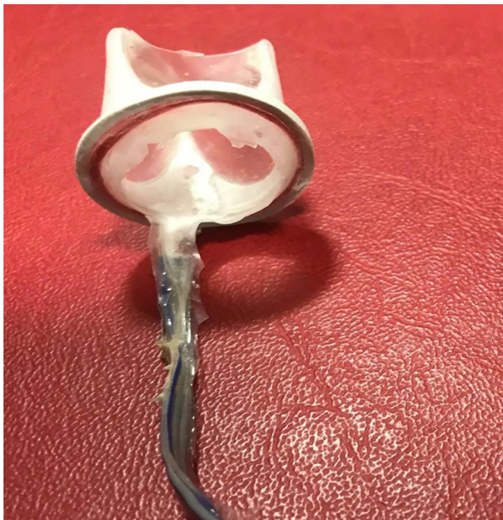
Figure 5.38. Polymeric heart valve instrumented with strain gauge
