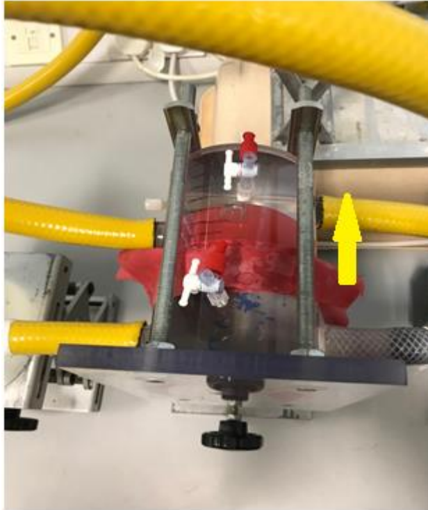
Figure 5.24. The ventricular chamber system in action (membrane extending upwards into the top chamber (shown by yellow arrow) suggests the pump in diastole mode).
