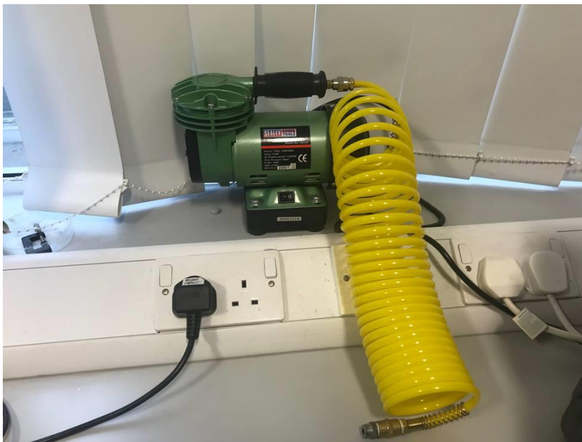
Figure 5.18. The mini air brush compressor used to introduce air into the pneumatic chamber
