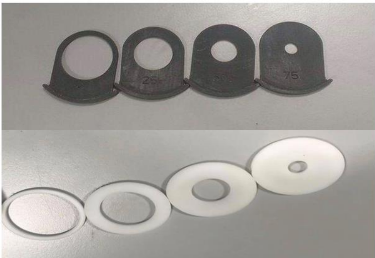
Figure 5.34. Obstruction discs used to simulate the 4 various degrees of valve stenosis/obstruction, from 0%-75% obstruction, from left to right respectively. Top: Polymeric valve. Bottom: Bioprosthetic valve
