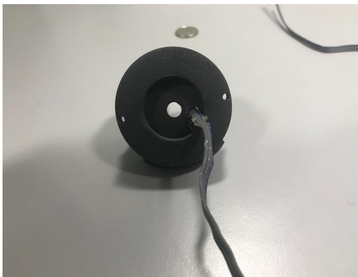
Figure 5.39. Bottom view of the strain gauged polymeric valve in the valve holder with the 75% obstruction disc. Hole has been drilled in the obstruction disc to allow for the lead wires of the strain gauge.
