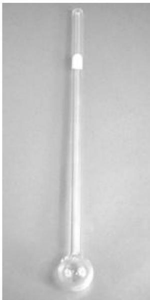
Figure 26: Micromeritics ASAP 2420 Sample Tube.<sup>137</sup>
