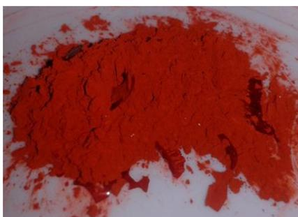
Figure 46: A dried RF gel sample made with no metal carbonate present.
