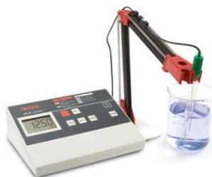
Figure 24: Hanna Instruments pH 20 pH meter.<sup>135</sup>
