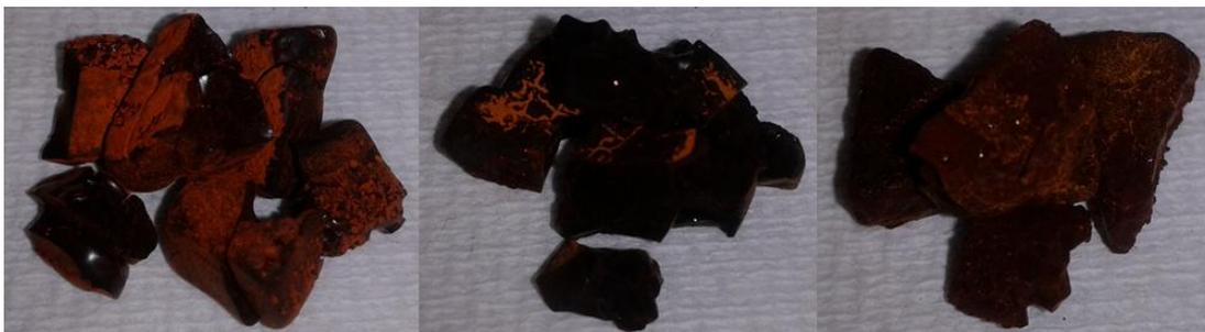
Figure 74: Visual comparison of mixed  $\text{Na}_2\text{CO}_3/(\text{NH}_4)_2\text{CO}_3$  gels with, from left to right, R/C 50, 100 and 200.
