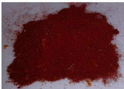
Figure 67: A dried RF gel sample made with ammonium carbonate.
