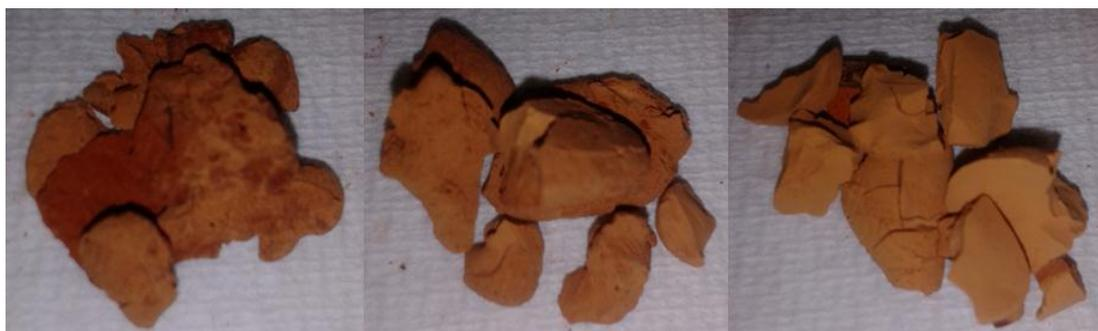
Figure 79: Visual comparison of mixed  $\text{CaCO}_3/(\text{NH}_4)_2\text{CO}_3$  gels with, from left to right, R/C 50, 100 and 200.
