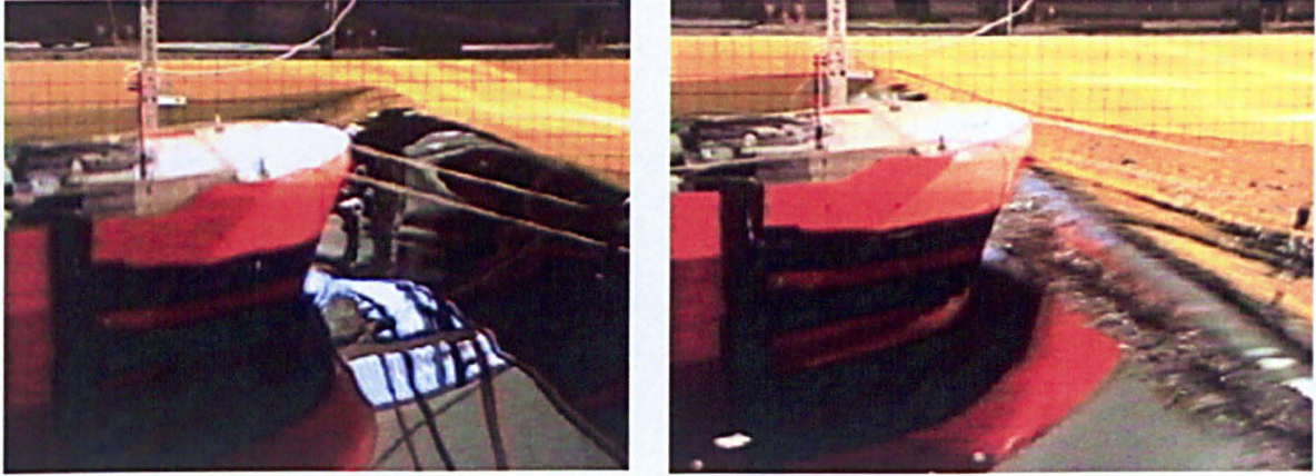
Figure 2.16 Highest and steep fronted new-wave as generated in the model tank
