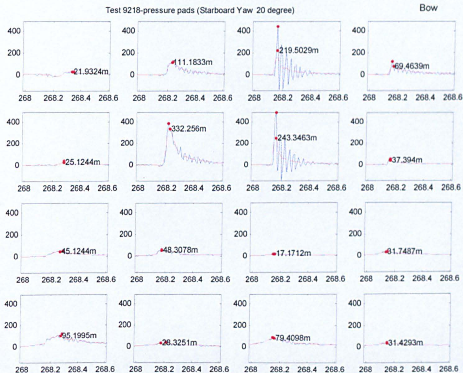
Figure A4.2 Panel pressure time history H_s = 17.08\text{m} , T_z = 12.8\text{sec} , Steepness = 1/15 , Steepness factor = 50%, 20 degree yaw
