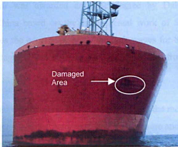
Figure 1.2 The bow damage of Schiehallion FPSO
