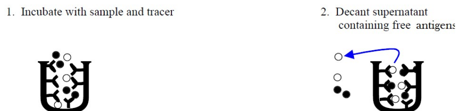
Fig. 1.15: Schematic of solid phase RIA (adapted from Forghani et al. , 1974).
