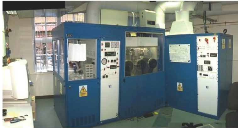
Figure 3.1: Image of the Thomas Swan CCS MOCVD reactor used at the University of Cambridge. The vast majority of devices studied in this work were grown by Dr Menno Kappers using this machine.
