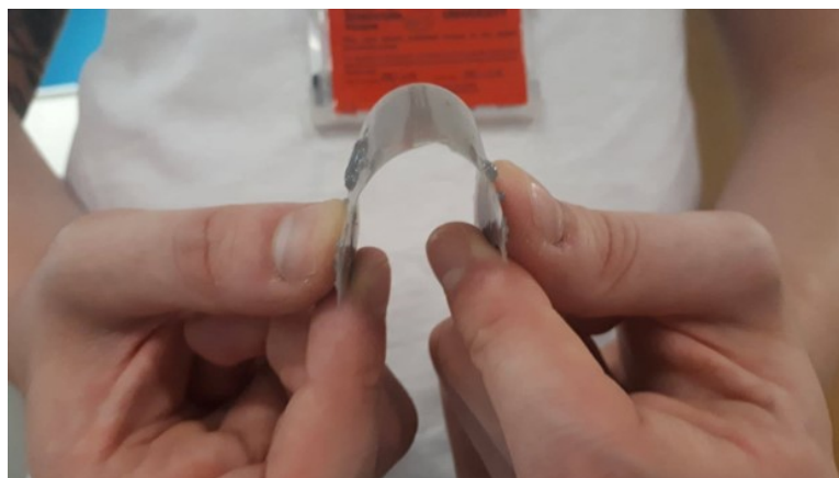
Figure 3.8: An optical image demonstrating how the cured resin can be handled and mechanically flexed without damage. This grey film was cured on a flat microscope objective and easily peeled off and bent.
