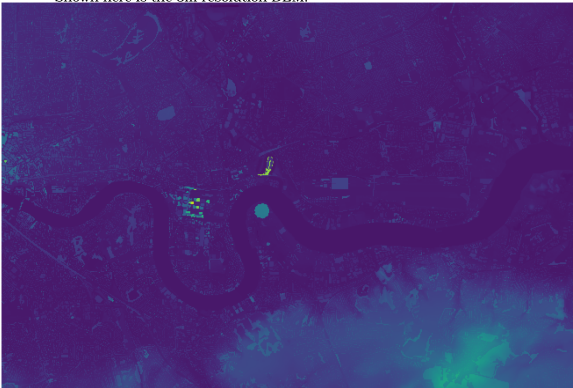
Shown here is the 5m resolution DEM redrawn to 1m resolution with added building heights.
