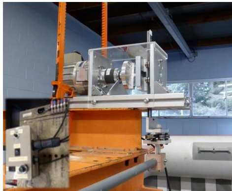
(a) Scotch yoke and DC Servo System
