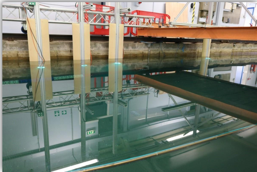
Figure 5.11 Installation of underwater cameras of the motion capture system
