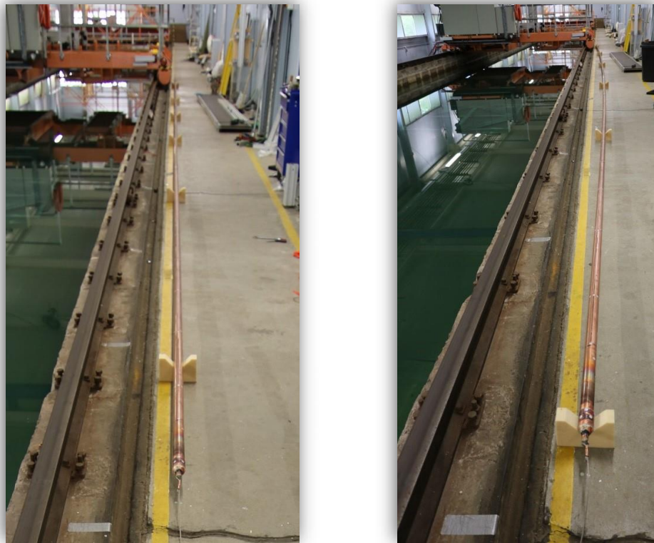
Figure 5.8 Verification/Calibration of the fibre optic sensing system
