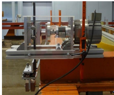
(b) Motor, Gearbox and linear motion guides
