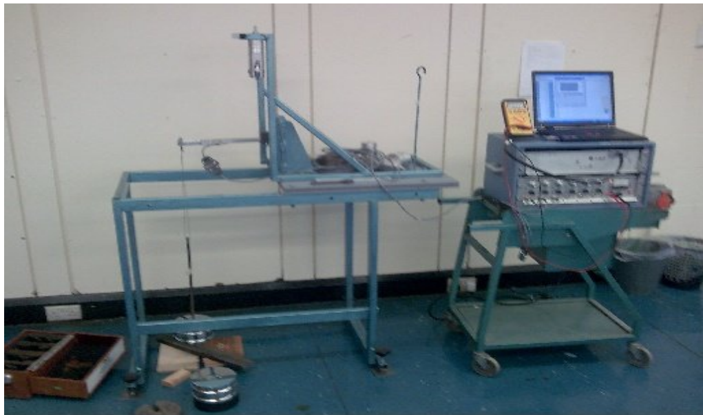
Figure 6.6: Calibration of the strain gauges for the mediolateral bending moment
