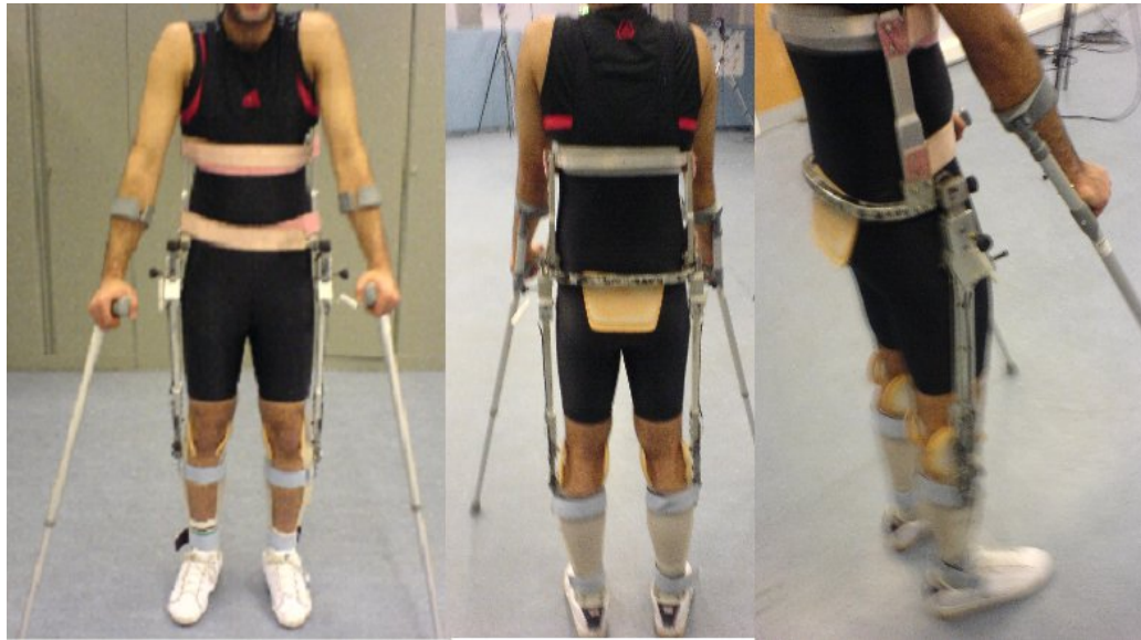
Figure 4.12: The new RGO orthosis, configuration 1, donned by a participant
