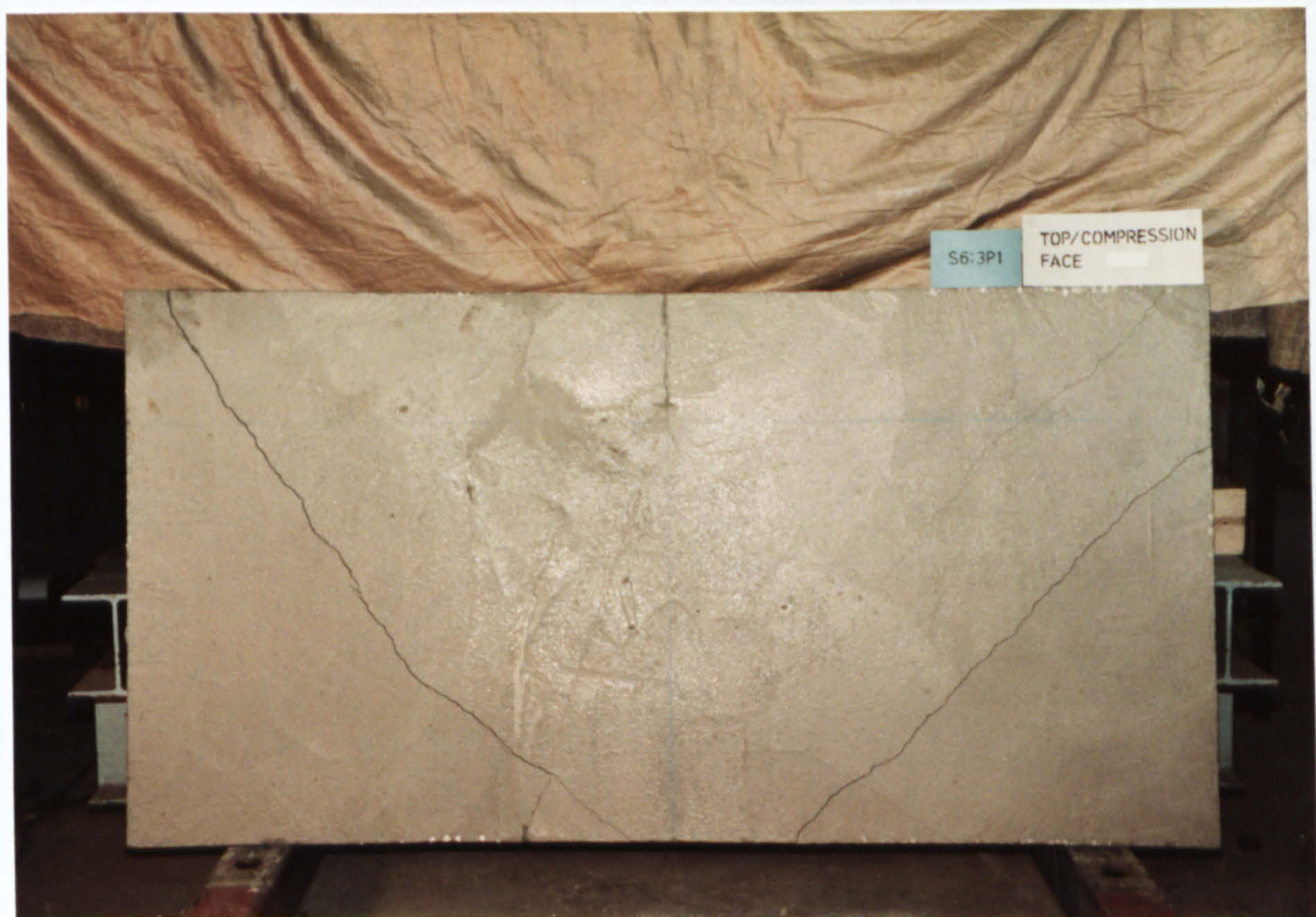
Plate 6.18 Compression Face of Model S63P1 After Failure.
