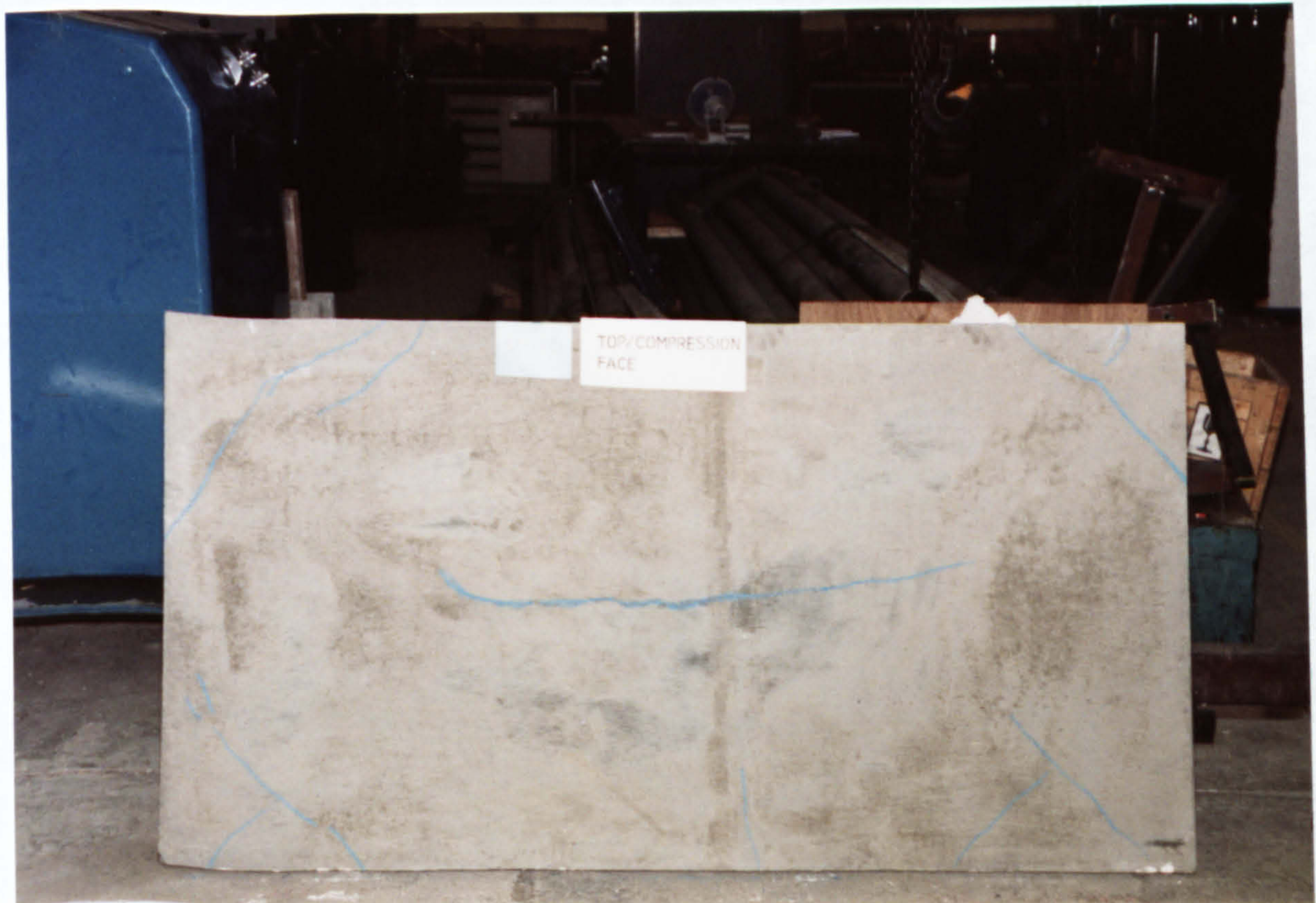
Plate 6.16 Compression Face of Model S54UD After Failure.
