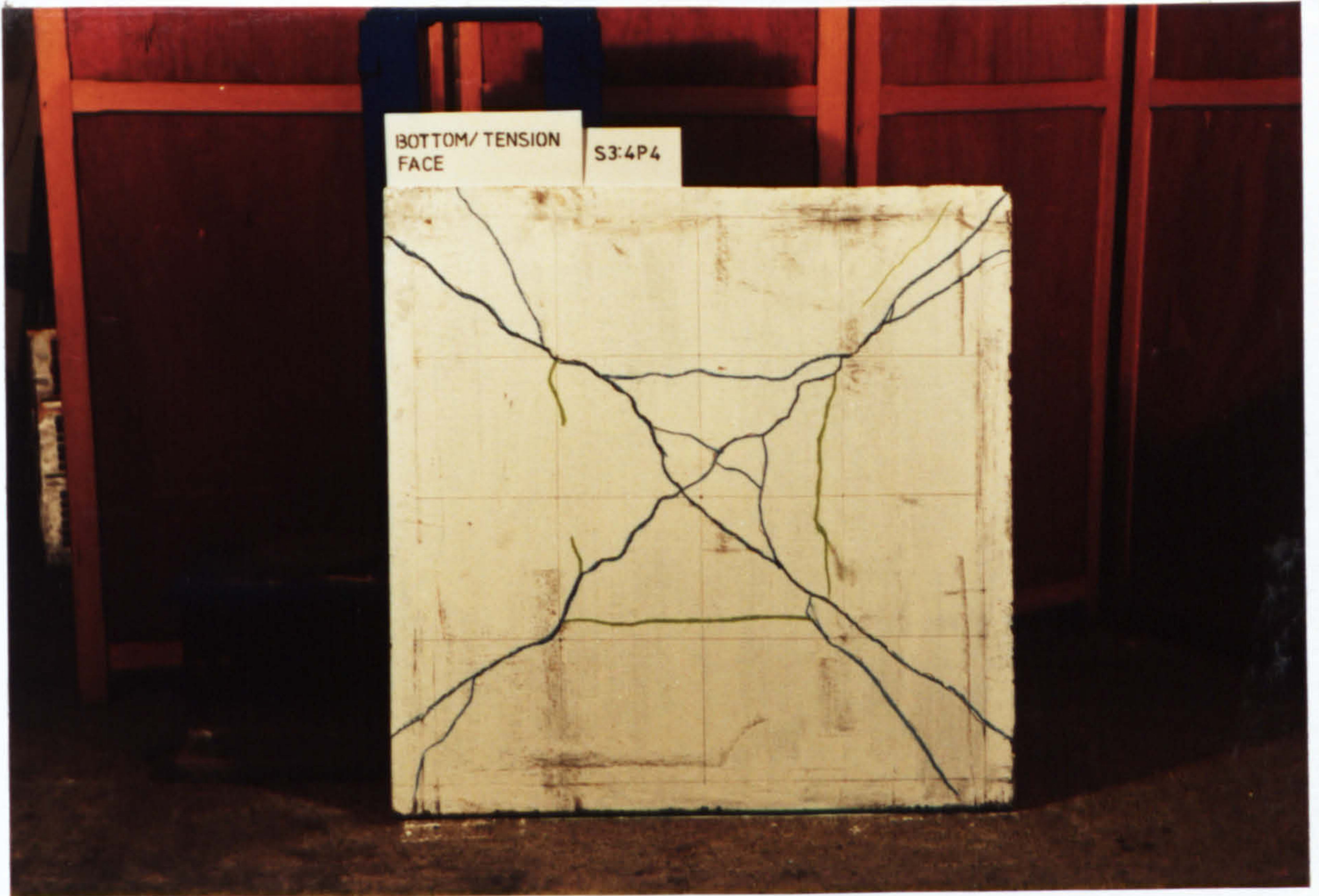
Plate 6.11 Crack Patterns at Failure on the Tension Face of Model S34P4.
