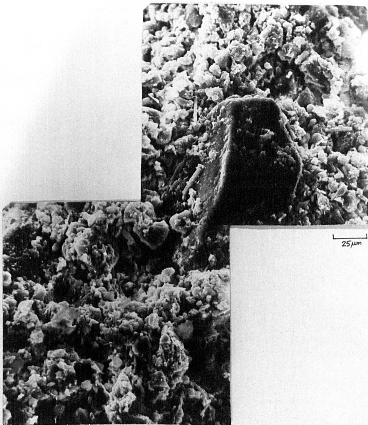
MIC.28. ANTARCTICA TILL - SAND PARTICLE IN CLAY- GRANULAR MATRIX.
