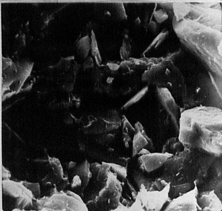
MIC.49 GLEN ORCHY TILL - DETAIL OF CLAY SIZE PARTICLES.
