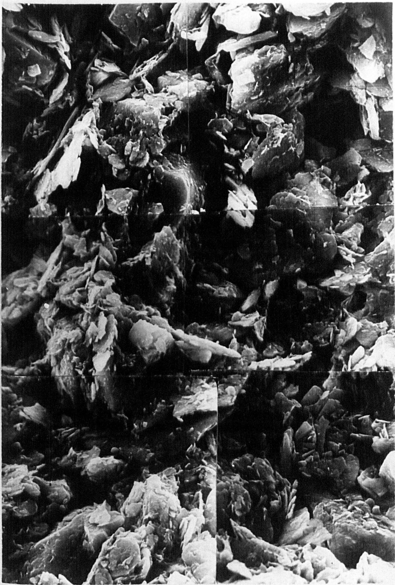
MIC.16. BLAISEN 1965 TILL - DETAIL OF CLAY SIZE ARRANGEMENTS.
