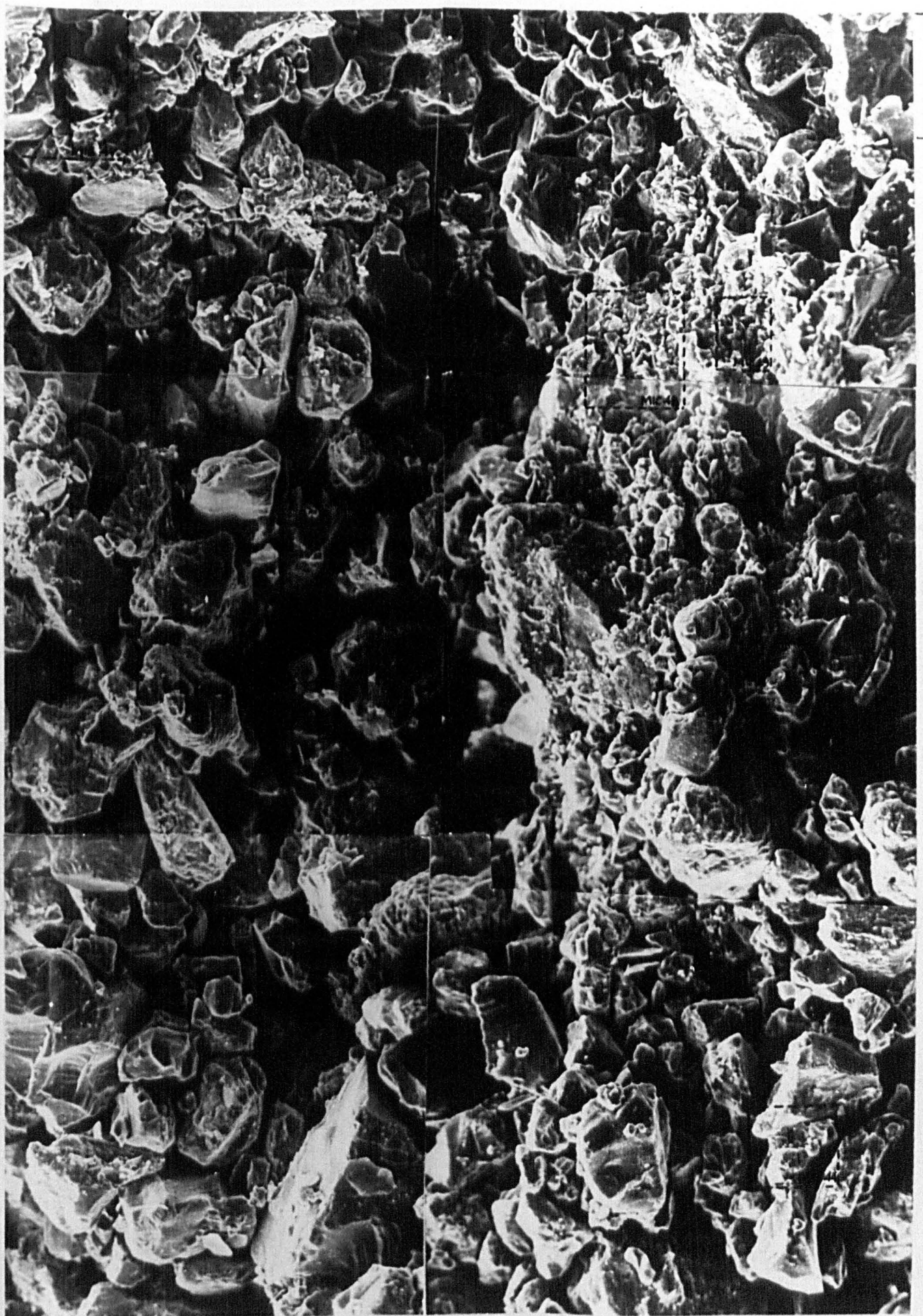
MIC. 43. GLEN ORCHY TILL - DISTRIBUTION OF COARSE AND FINE PARTICLES.
