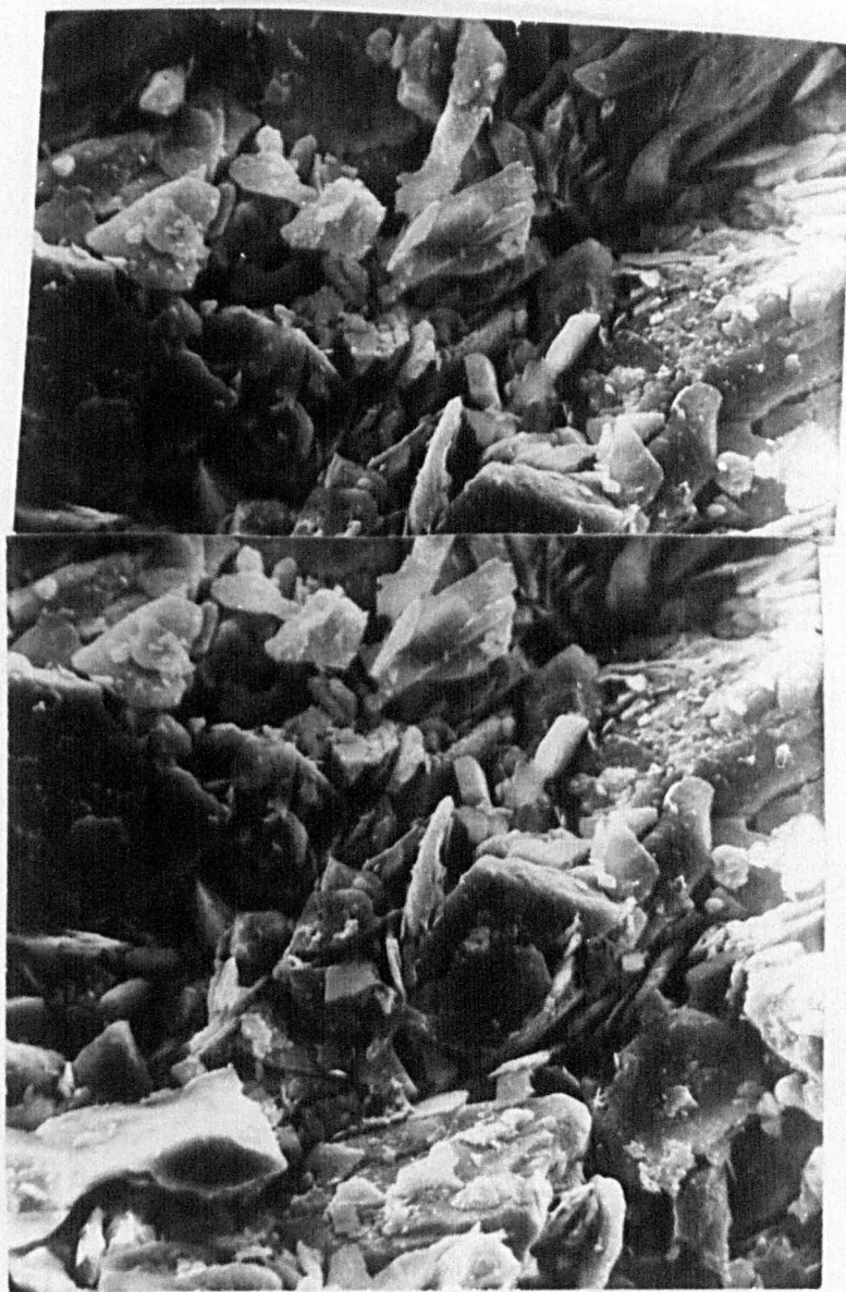
MIC 38 . COWAL TILL - THIN FLAKY FINE PARTICLES.
