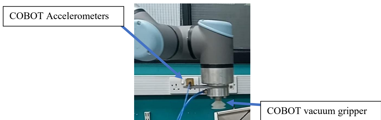
Figure 8-7 COBOT vacuum gripper attached
