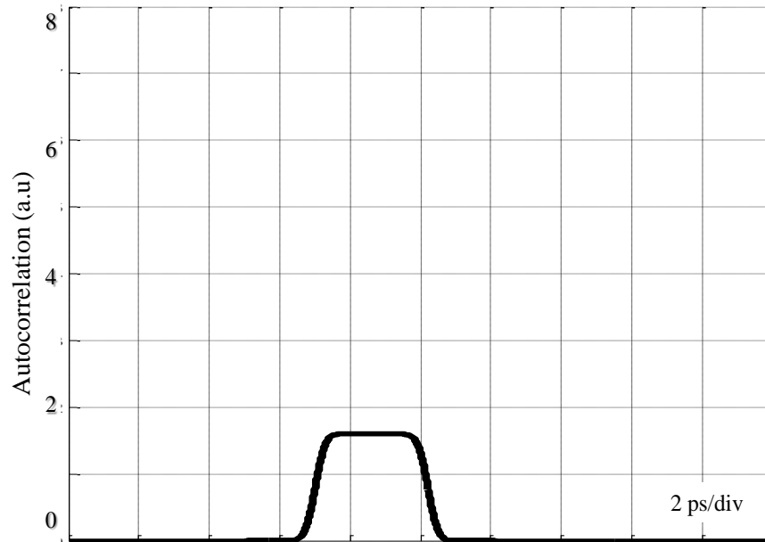
Figure 3.8 Plot of autocorrelation signal formed by decoding OCDMA transmission based on 2D-WH/TS OCDMA codes with 2 ps, 8 wavelength pulses after experiencing 20 o C temperature variation over a distance of 20 km.
