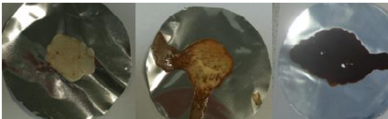
Figure 9.7 – Photographs of the E239 samples created from the ageing rig. The pictures going from left to right show the samples that have been aged for 5, 60 and 300 minutes at 320 °C.
