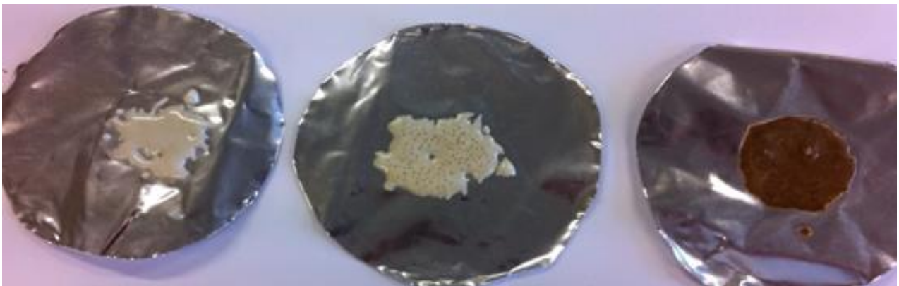
Figure 8.14 – Photographs of the E239 samples created from the ageing rig. The pictures going from left to right show the samples that have been aged for 5, 60 and 300 minutes at 320 °C.
