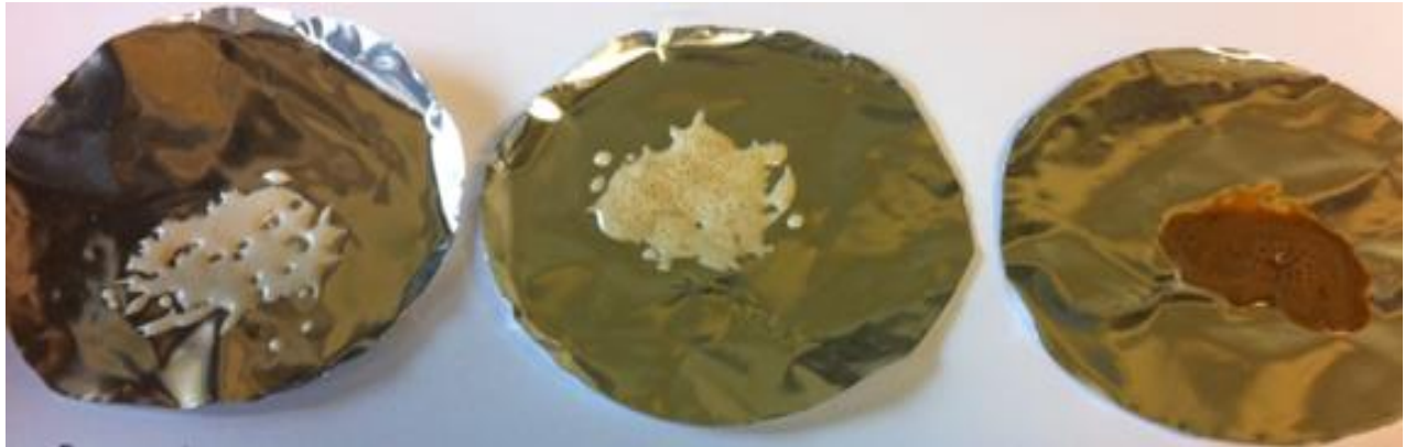
Figure 8.15 – Photographs of the E239 samples created from the ageing rig. The pictures going from left to right show the samples that have been aged for 5 , 60 and 300 minutes at 320 °C.
