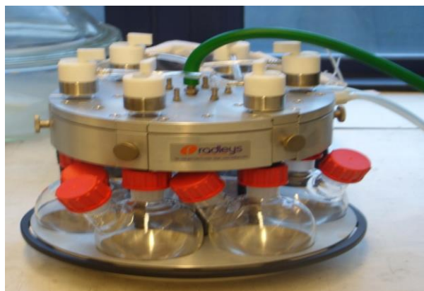
Figure 3.4 – Picture of the 6 position Radleys reaction carousel.
