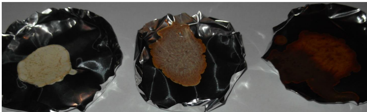
Figure 9.6 – Photographs of the E239 samples created from the ageing rig. The pictures going from left to right show the samples that have been aged for 5, 60 and 300 minutes at 305 °C.
