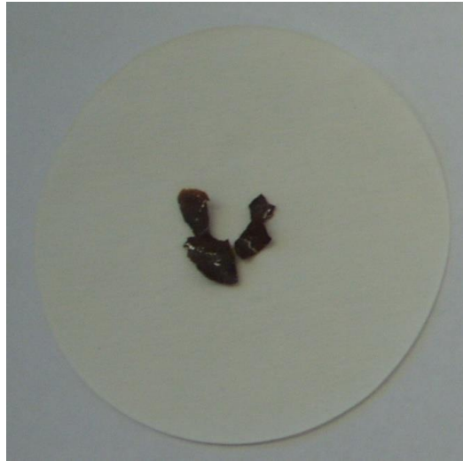
Figure 9.12 – Picture of the gel produced from the E239 sample prepared at 320 °C under air for 300 minutes.
