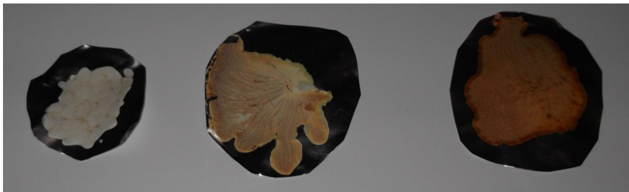
Figure 9.5 – Photographs of the E239 samples created from the ageing rig. The pictures going from left to right show the samples that have been aged for 5 , 60 and 300 minutes at 290 °C.
