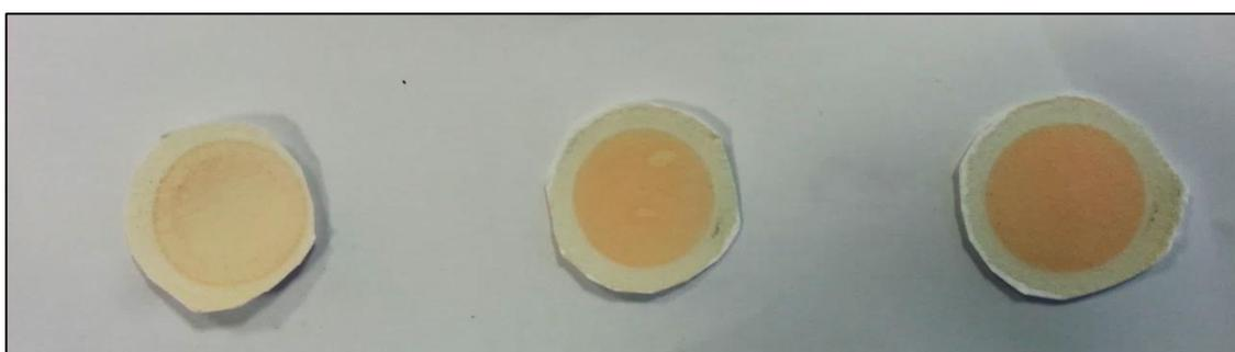
**Figure 4.2: Increase in colour intensity of  $\text{Hg}^{2+}$  complex formed on detecting paper obtained using the Hg bubbler apparatus and  $\text{Hg}^{2+}$  standards with concentration of 25, 50 and 75  $\mu\text{g/L}$ .**
