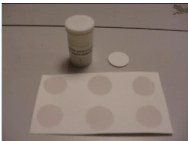
Figure 3.2: Plastic mould and sheet consisting of six CuI detecting papers.
