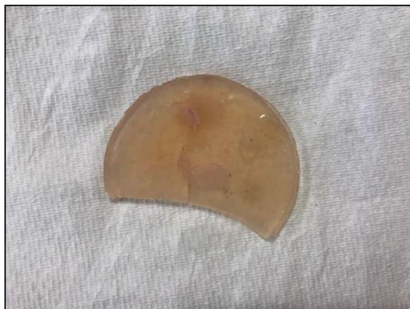
**Figure 6.21:** The observation of yellowish-pink coloration of 5% (w/v) agar caused by the leakage of the immobilised reagent from the sensing membrane.
