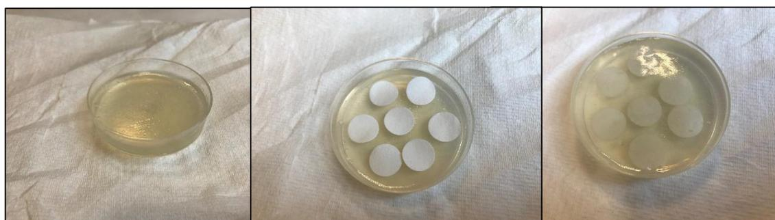
**Figure 6.1:** Covering procedure of the agar-agar membranes by 5% (w/v) agar colloid. (a) melted agar was poured in a petri dish to cover the bottom (about a quarter), (b) agar-agar membranes placed on the surface, (c) another layer of melted agar was poured in the top. The carrier support was cut and peeled off the membranes prior use.
