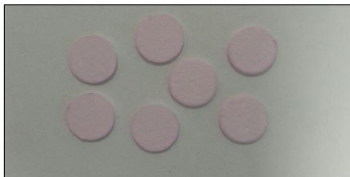
**Figure 5.17: Formation of light pink colour as a result of the reagent ring-opening after completely drying the discs for 24 hrs.**
