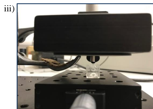
Figure 3.8: a) Schematic of the fluorescence lifetime system incorporating liquid light guides and a translational stage to place the sample where the same couplings for the light guides to the excitation source and detector were used as in the previous setup, and b) photographs of the i) full setup with the translational stage, with a more detailed view of the sample stage design in ii) and iii).
