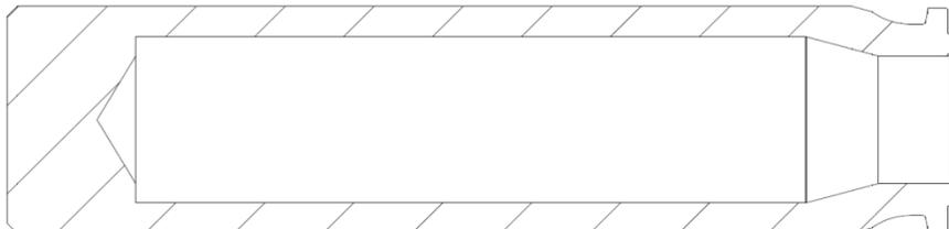
**Figure 3-9: Plunger section**
