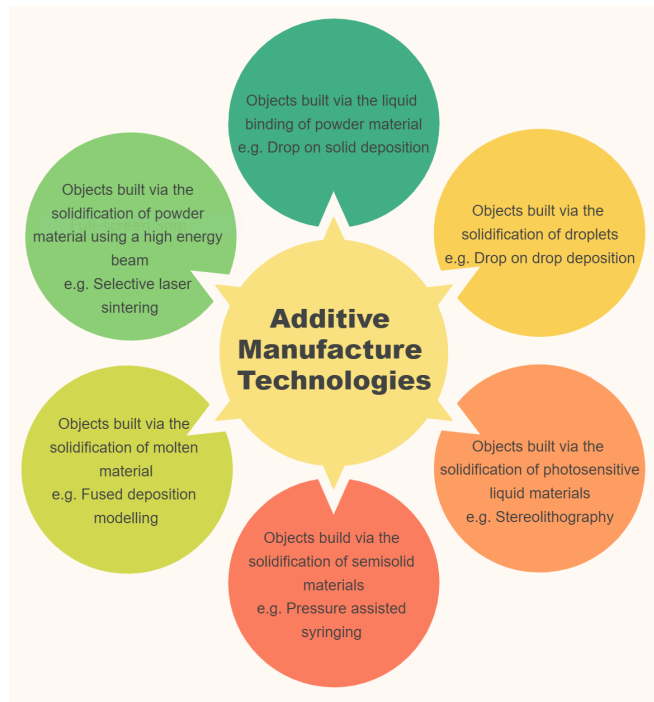
Figure 1.4: A selection of the AM techniques, with an example for each, adapted from (Jamróz et al., 2018).
