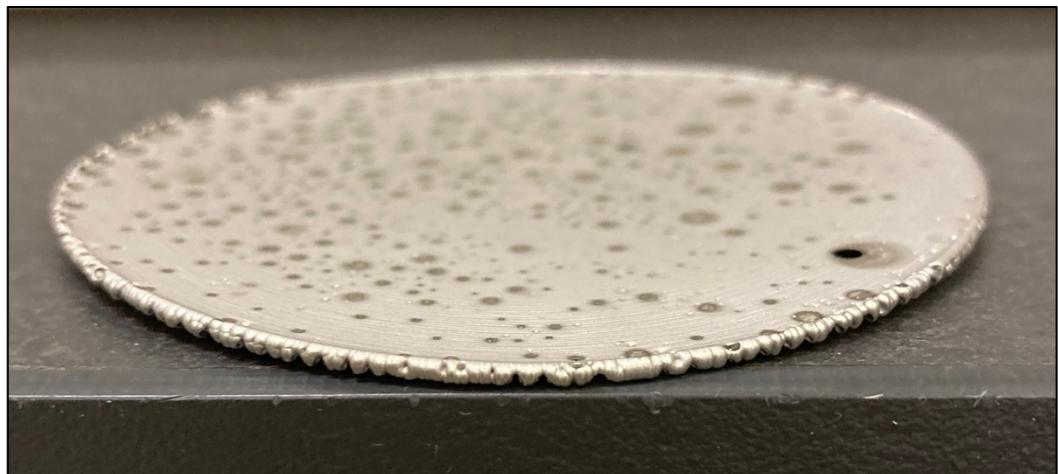
**Figure 4. 9:** Real-life nickel electroform produced in the prototype electroforming reactor at  $-2.5 \text{ V}$  and  $-1 \text{ A}$ , for  $10800 \text{ s}$ , at  $50 \text{ }^\circ\text{C}$ , under agitation.
