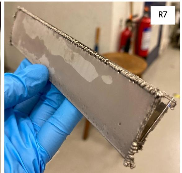
**Figure 5. 7:** Nickel mechanical vane electroforms R5, R6 and R7. The difference in the dendrites size is highlighted, with R5 presenting the thinnest dendrites around its leading edges and R7 the thicker ones. Electroforms R5, R6 and R7 were produced at  $7.22 A/dm^2$  after deposition for 3.5 h, 5 h and 6 h, respectively, at 50 °C.
