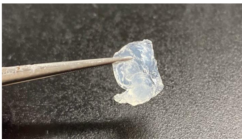
Figure 8.22: Alginate:G 4 RGDSP hydrogel (3.3% (w/v):0.25 mM) crosslinked via BaCl 2 (66 mM).
