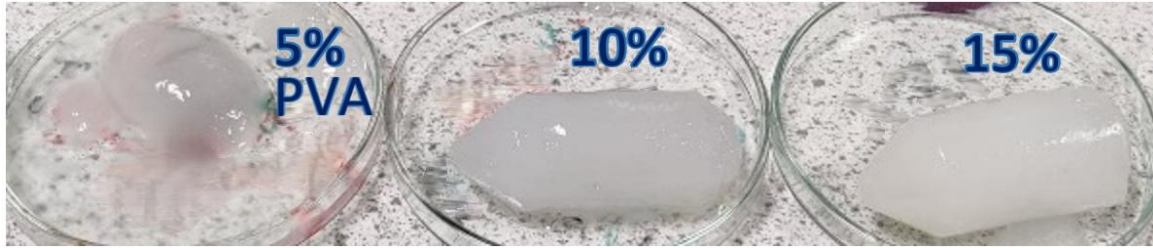
Figure 7.25. Freeze-thaw PVA gels formed from solutions of varying PVA wt%, after 2 freeze thaw cycles.
