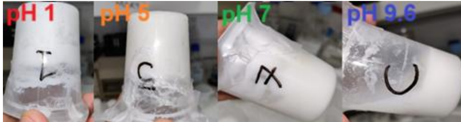
Figure 7.18. 1 wt% PEI in CS at pH 1, 5, 7 and 9.6, from left to right, left for 7 days. No NaCl accelerator solution was used.
