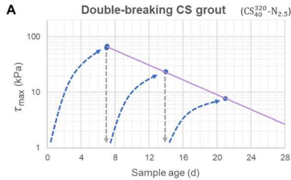
Figure 5.4. \tau_{max} data for a CS_{40}^{320}-N_{2.5} sample cured for 7 d, broken, healed for 7 d, broken again, and re-healed for a further 7 d. The blue arrows represent curing and re-healing, and the grey arrows represent breaking. The purple line is an exponential fit.
