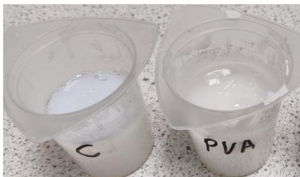
Figure 7.22. On the left is standard gelled CS grout; on the right is gelled CS/PVA grout, containing 1 wt% PVA. These were each prepared with 1.7 M NaCl accelerator, at 5:1 volume ratio. In the case of the CS/PVA grout, the PVA was dissolved in the accelerator. The upper layer of water which formed from phase separation has been removed from the gelled CS/PVA grout here.
