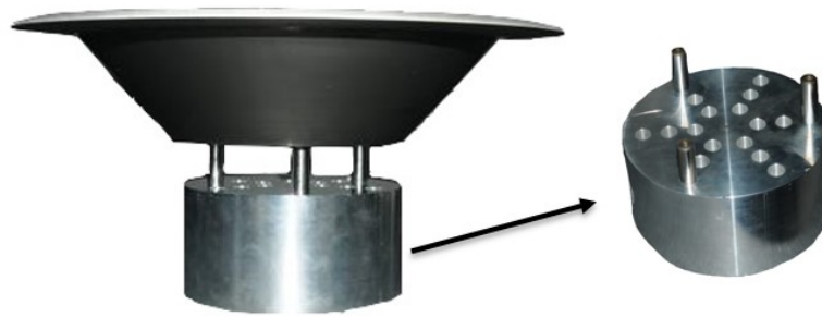
Figure 4.5: Set-up of a shear formed part on the fixture for CMM measurement.
