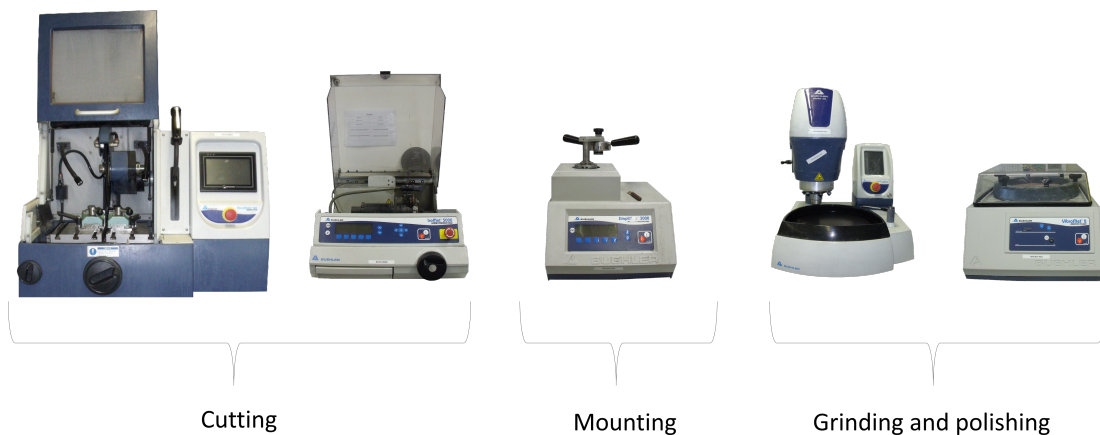
Figure C.8: Metallurgical preparation – Equipment.
