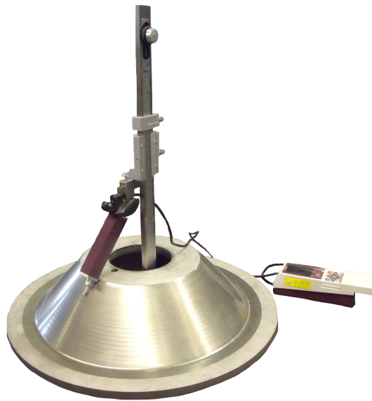
Figure 4.3: Set-up of the Surfatest SJ-210 and its fixture to measure the surface roughness of a shear formed part.
