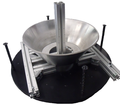
Figure 4.4: Scanning with a rotating table and a frame using ATOS III Triple Scan.
