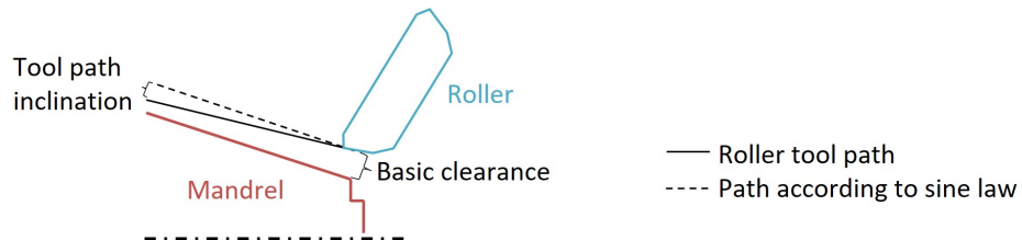
Figure 2.4: Tool path inclination – adapted from Kunert et al. (2005).
