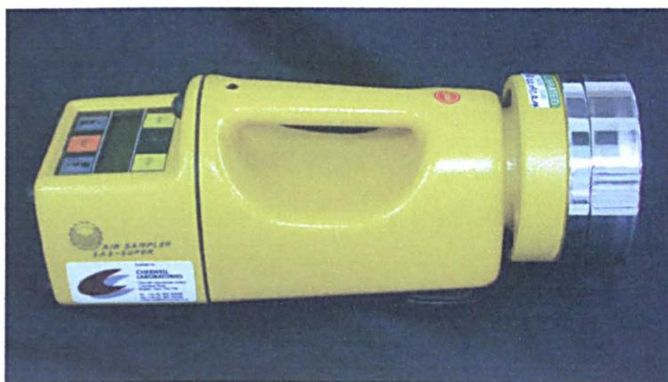
**FIGURE 4.1** *SAS Super-180 Air Sampler*
