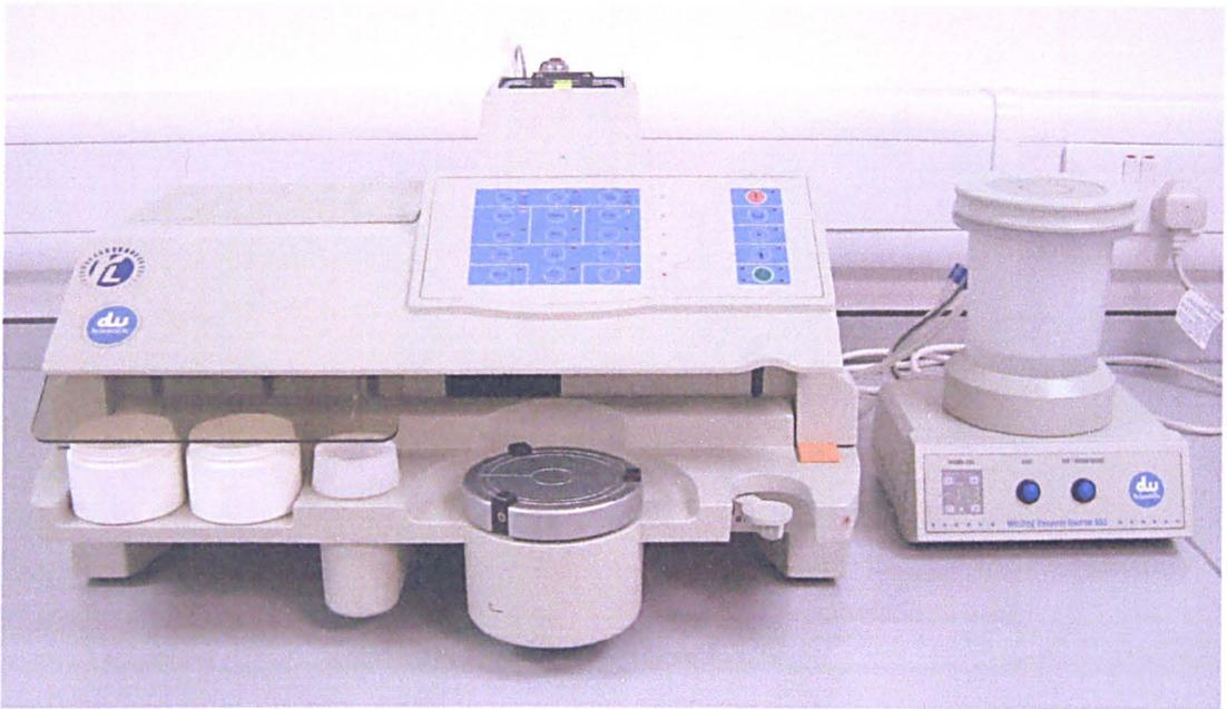
**FIGURE 3.1** *WASP 2 Spiral Plater*
