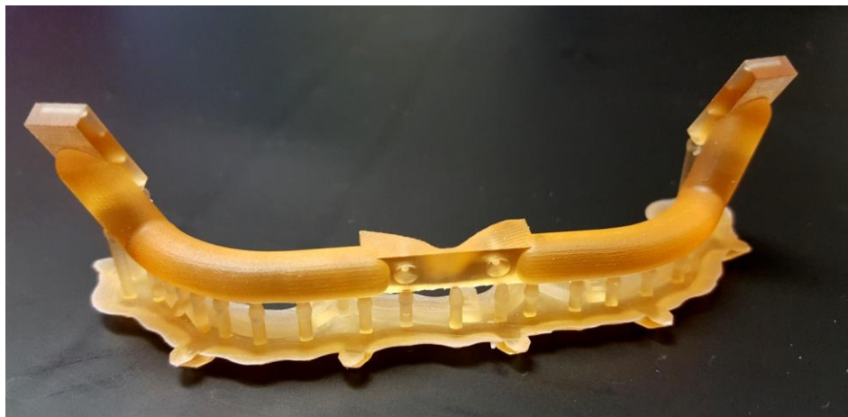
Figure 3.5.12 Framework post curing before the support structures were removed with the use of the snipping tool
