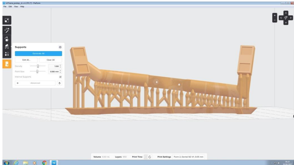
Figure 3.5.10 Support structures applied post editing
