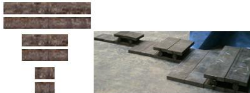
Figure 7.3: Difference Sizes of Steel Plates Used for Load and Support Conditions in Series "1".
