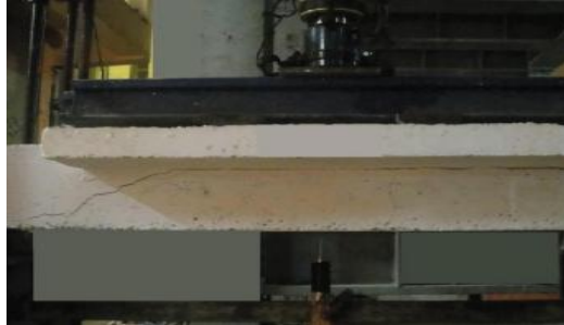
Figure 3.4: Wide Beams Tested by Hanafy et al. (2012), they may be considered as T-Sectioned Wide Beams.
