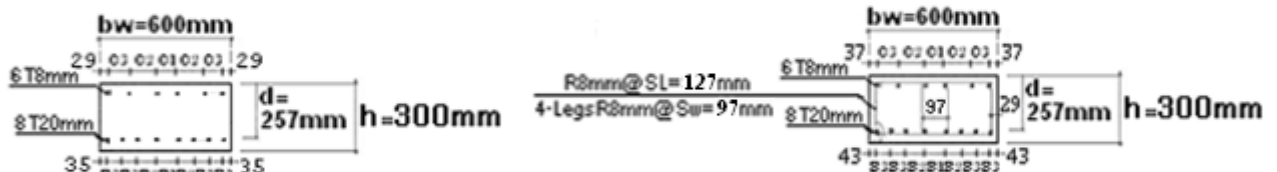
Beams in Type (C)
