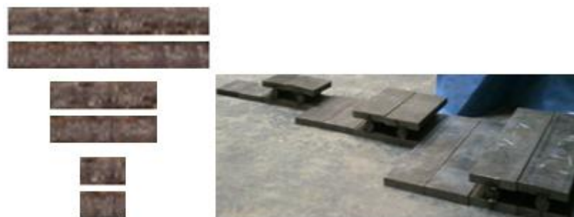
Figure 9.3: Difference Sizes of Steel Plates Used for Load and Support Conditions in Series "2".
