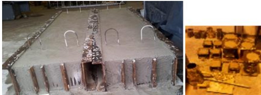
Figure 5.6: Beams in Series "A" together with own Control Samples after Concrete Casting.
