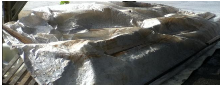
Figure 9.7: The Curing Process of Typical Beams in Series "2" after Removing the Shutters.
