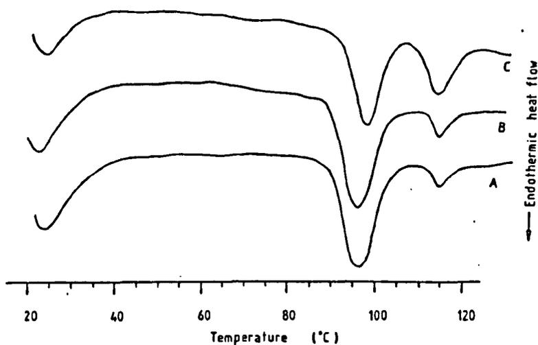
Fig. 90 DSC thermograms of amylose-lauric acid complexes formed from original alkaline solutions (0.01M KOH), neutralised (pH 4.6) and precipitated at temperatures: A, 50°C; B, 60°C; C, 70°C.
