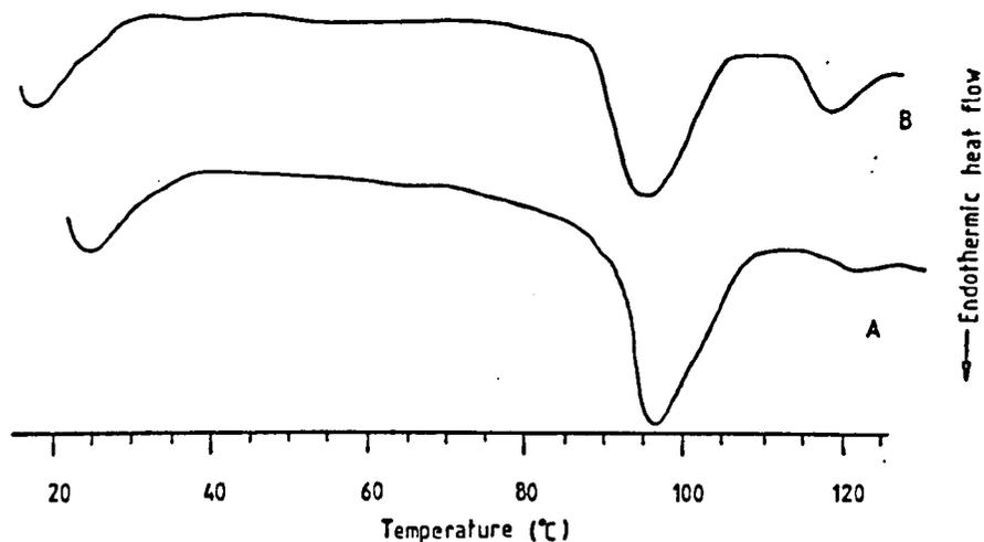
Fig. 97 DSC thermograms of amylose complexes with palmitic acid formed from original alkaline solutions (0.01M KOH), neutralised, precipitated and extracted with methanol: A as wet precipitate at 50°C for 1 h; B as freeze-dried precipitate at 20°C for 1 h.
