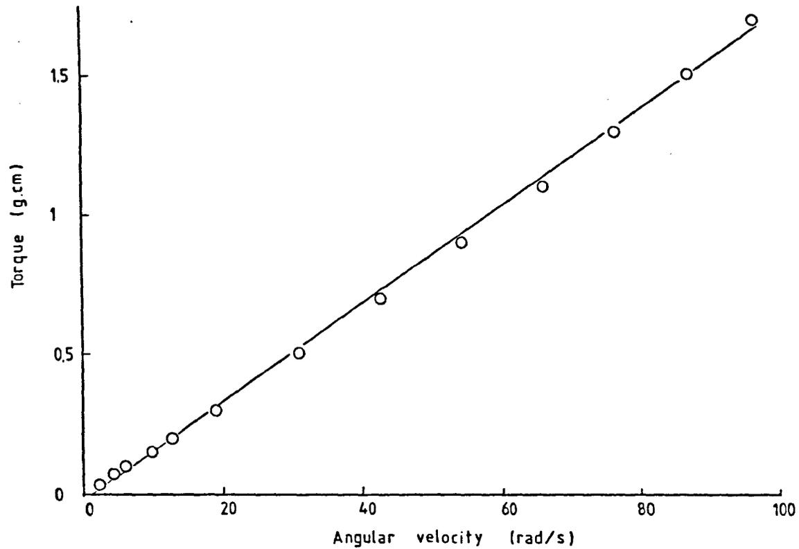
Fig. 93 Measured angular velocity as a function of the applied torque for the air bearing friction of the Viscoelastic analyser (Sangamo). Regression equation: Friction torque:  $y = -0.0205 + 0.0174\Omega$ ;  $r = 0.9995$ .
