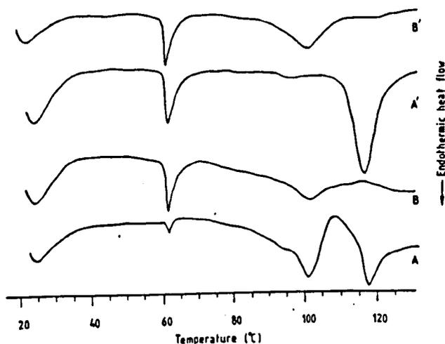
Fig. 87 DSC thermograms of amylose complexes with palmitic acid formed: A, from original alkaline solution (0.01M KOH), neutralised, precipitated and heated at 90°C for 16 h; B, from original DMSO solution, precipitated after dilution with H<sub>2</sub>O and buffer (pH 4.6) and heated at 90°C for 16 h; A', prepared as A but heated at 135°C for 30 min and then at 90°C for 16 h; B', prepared as B but heated at 135°C for 30 min and then at 90°C for 16 h.
