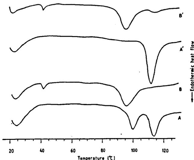
Fig. 86 DSC thermograms of amylose complexes with lauric acid formed: A, from original alkaline solution (0.01M KOH), neutralised, precipitated and heated at 90°C for 16 h; B, from original DMSO solution, precipitated after dilution with H<sub>2</sub>O and buffer (pH 4.6) and heated at 90°C for 16 h; A', prepared as A but heated at 135°C for 30 min and then at 90°C for 16 h; B', prepared as B but heated at 135°C for 30 min and then at 90°C for 16 h.
