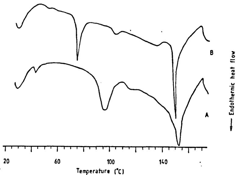
Fig.89 DSC thermograms of amylose complexes with: A, lauric acid from original DMSO solution, precipitated after dilution with water and buffer (pH 4.6), heated at 135°C for 30 min and then at 90°C for 16 h; B, arachidic acid prepared and heattreated as A.
