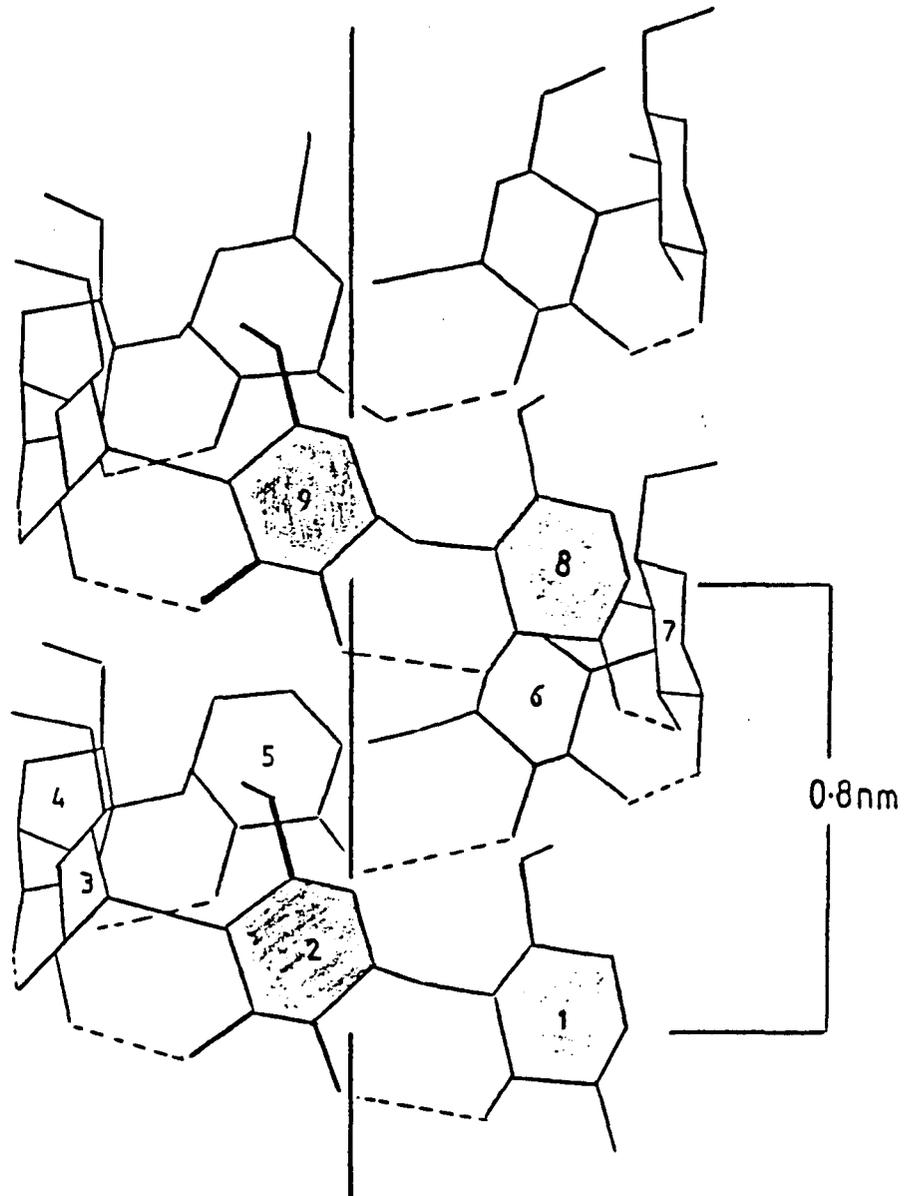
Fig. 25. Amylose helix showing pitch (0.8 nm) and seven residues per turn. (French and Murphy, 1977).
