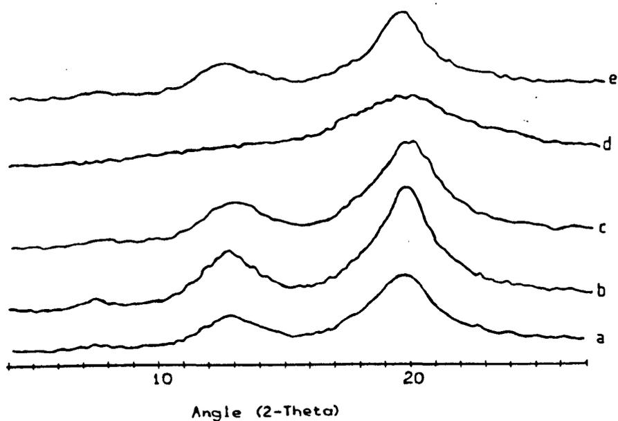
Fig. 92 X-ray diffraction diagrams of freeze-dried amylose-fatty acid complexes: a, capric acid-amylose complex (0.150); b, capric acid-amylose complex precipitated at 50°C (0.200); c, palmitic acid-amylose complex (0.045); d, palmitic acid-amylose complex precipitated from DMSO (10%)-water solution; e, arachidic acid-amylose complex (0.045). Molar ratio FA/AM in parentheses.
