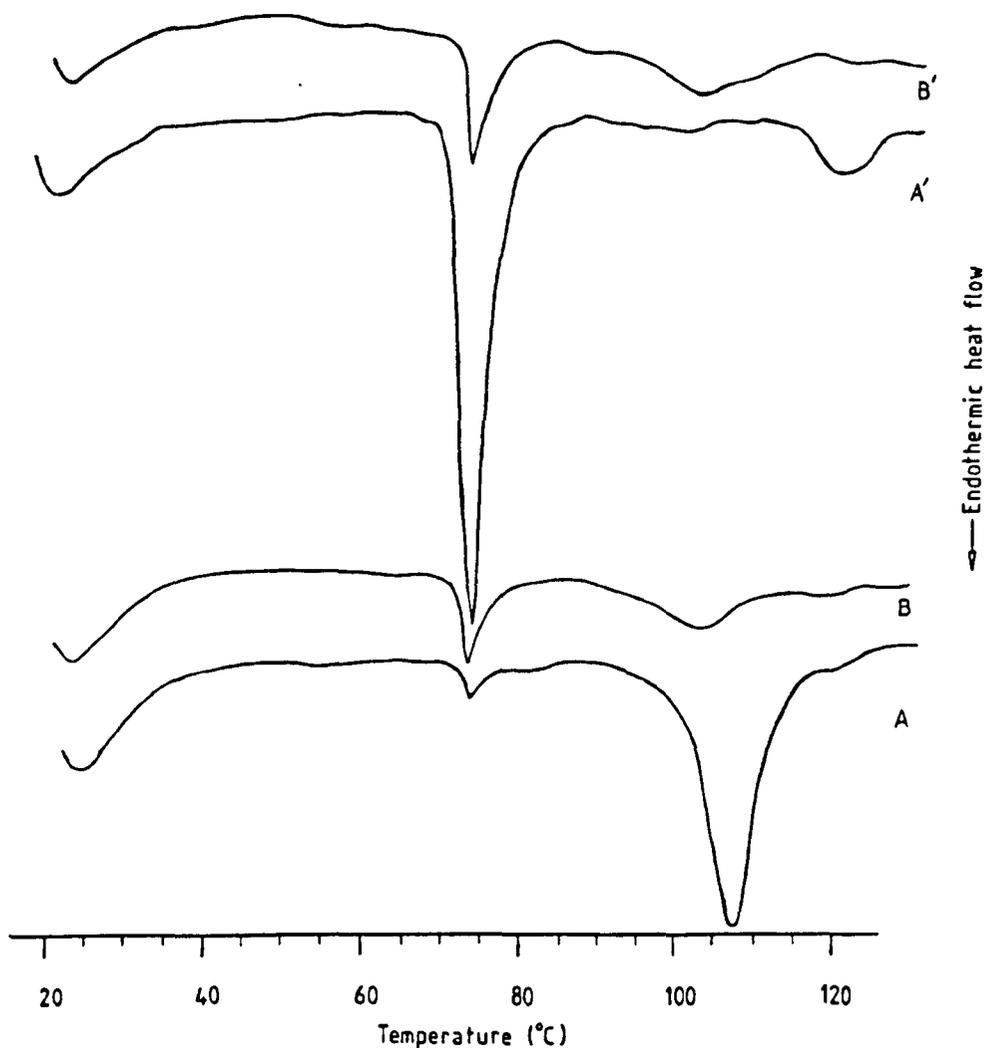
Fig. 88 DSC thermograms of amylose complexes with arachidic acid formed: A, from original alkaline solution (0.01M KOH), neutralised, precipitated and heated at 90°C for 16 h; B, from original DMSO solution, precipitated after dilution with H<sub>2</sub>O and buffer (pH 4.6) and heated at 90°C for 16 h; A', prepared as A but heated at 135°C for 30 min and then at 90°C for 16 h; B', prepared as B but heated at 135°C for 30 min and then at 90°C for 16 h.
