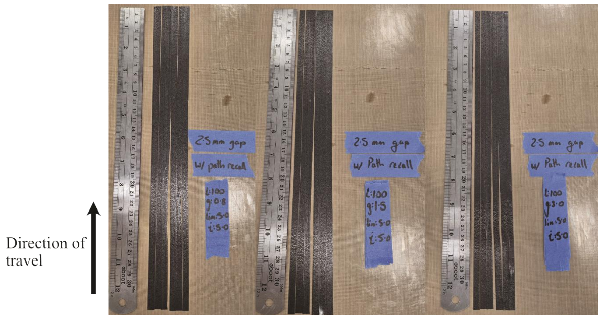
Figure 7.13. 2.5 mm gap mitigation for L = 100.0 mm with varying gain values (0.8, 1.5, 3.0)
