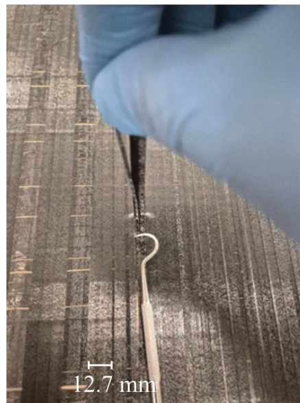
Figure 4.8. Fibre breakage during RM3
