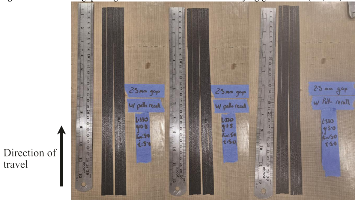
Figure 7.14. 2.5 mm gap mitigation for L = 330.0 mm with varying gain values (0.8, 1.5, 3.0)
