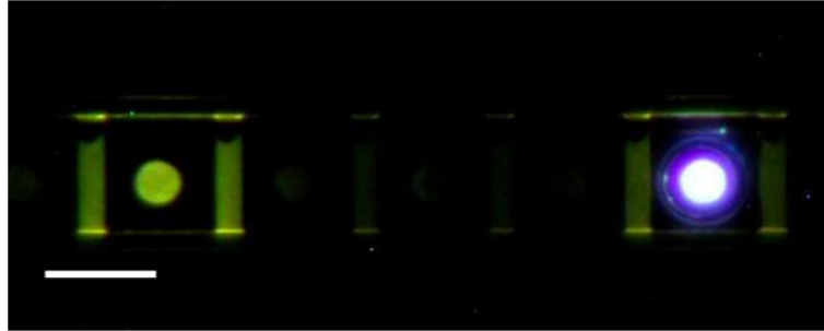
Fig. 1.9 Inkjet printed organic semiconductor material on micro-LED pixels. Optical micrographs of two LED pixels: bare UV micro-LED pixel (left) and the LED pixel with integrated light emitting polymer structure (right). The scale bar represents 50 \mu\text{m} ; from [17].
