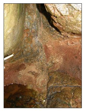
Figure 3.6: PSZ detail of VPF in the saprolitic bole layer. Note brecciation of basalt on either side of the slip surface, and then the narrowing of fault-related deformation within the bole itself. Photo toward north.
